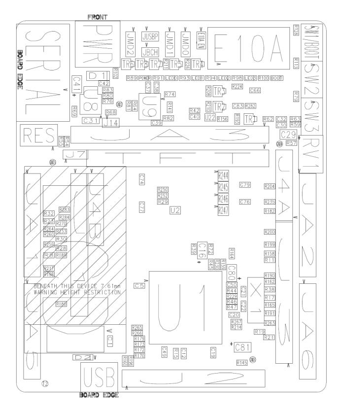
Figure 11-1: Component Placement (Top Layer)
