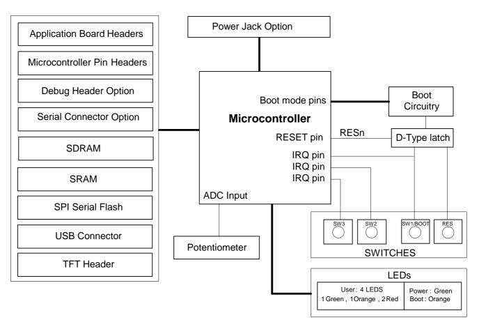
Figure 5-1: Block Diagram
