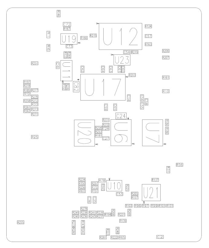
Figure 11-2: Component Placement (Bottom Layer)
