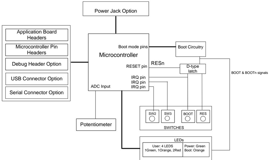
Figure 5.1: Block Diagram
