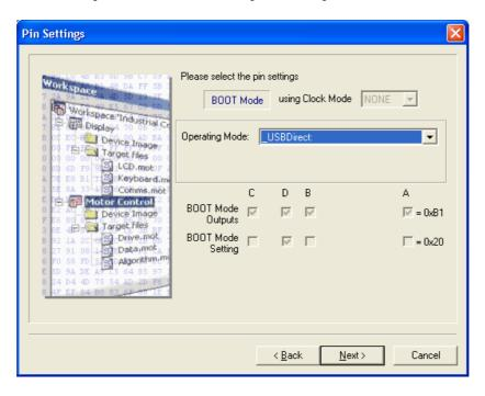
Figure 7.1: Boot Mode FDT configuration
