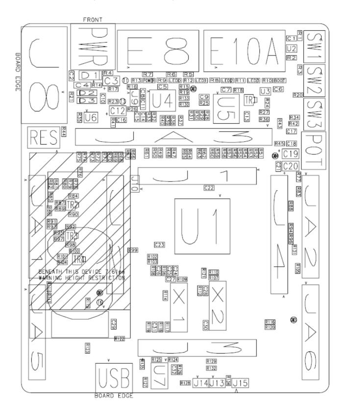
Figure 11-1: Component Placement
