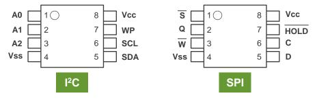
Pin Arrangement: 8-pin SOP / 8-pin TSSOP (Top View)
