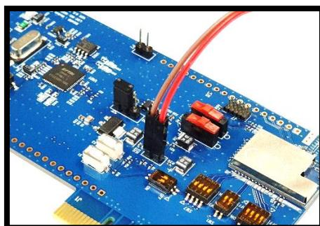
**Figure 60: Test Point for Current Measurement**
