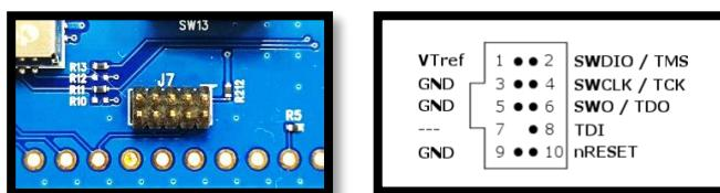
**Figure 2: JTAG Pin Connection**
