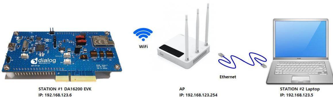
**Figure 30: Iperf Test Environment**
