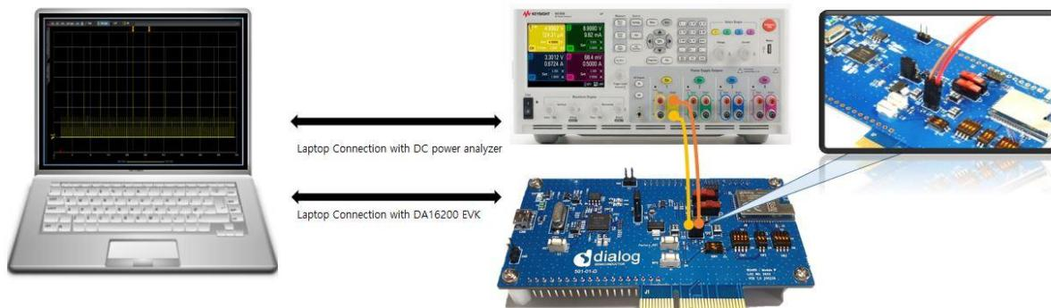
**Figure 21: Current Test Environment**
