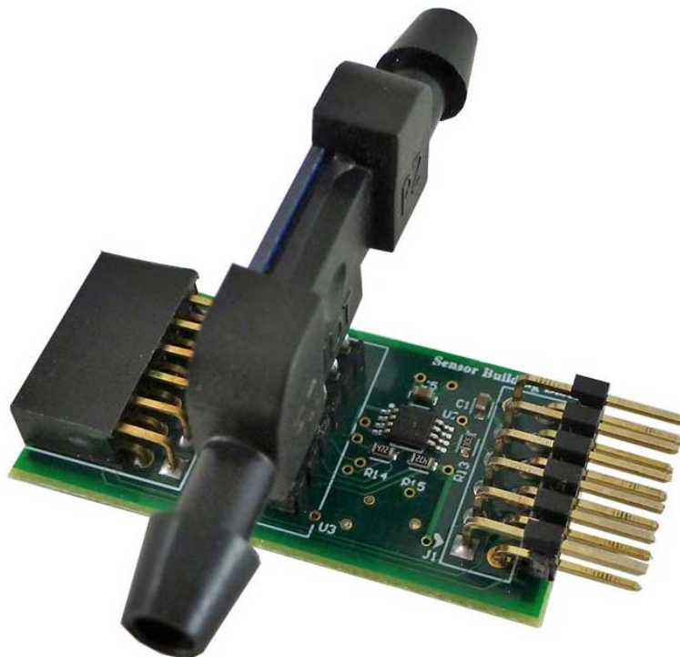
Figure 1. US082-FS2012EVZ Pmod Board
