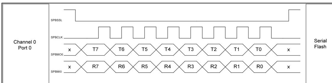
Figure 5.5.2: Single bit single channel operation mode.
