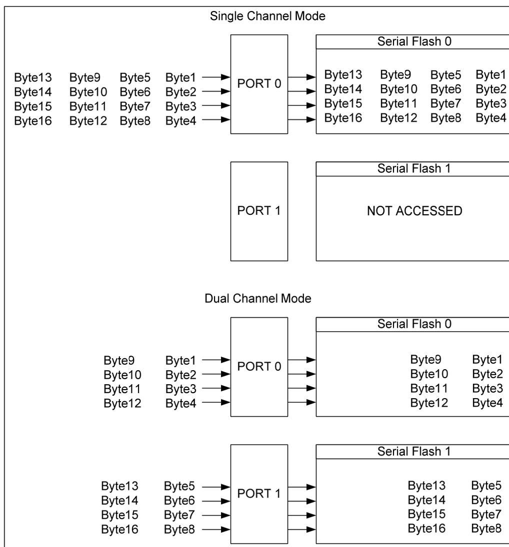
**Figure 5.3: Memory access of Single and Dual Mode QSPI Operation.**
