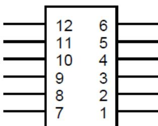
Figure 5.5: Digilent Pmod™ Compatible Header Pin Numbering
