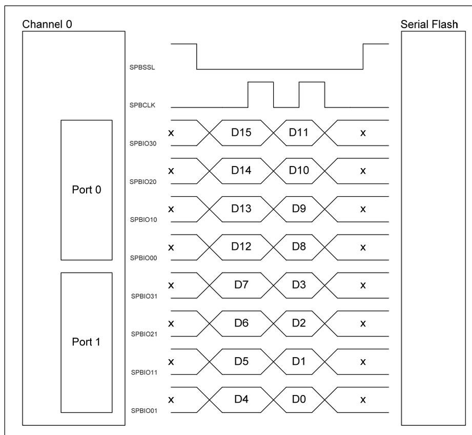
Figure 8.4: Example of a 4-bit data size using two serial flash memories.
