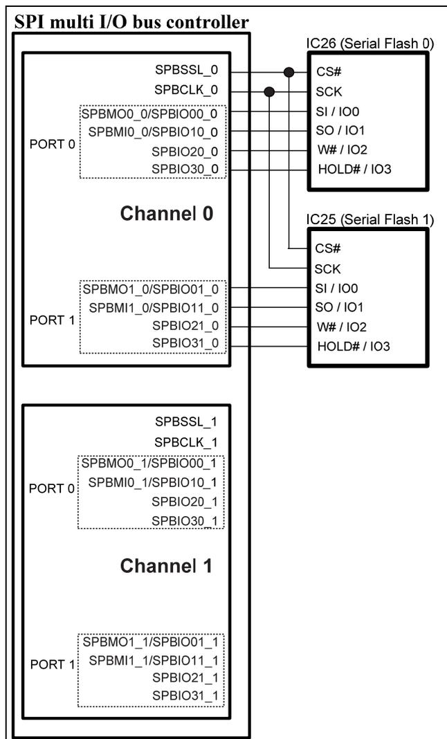
Figure 5.5.1: RZ/A1H SPI multi I/O controller.
