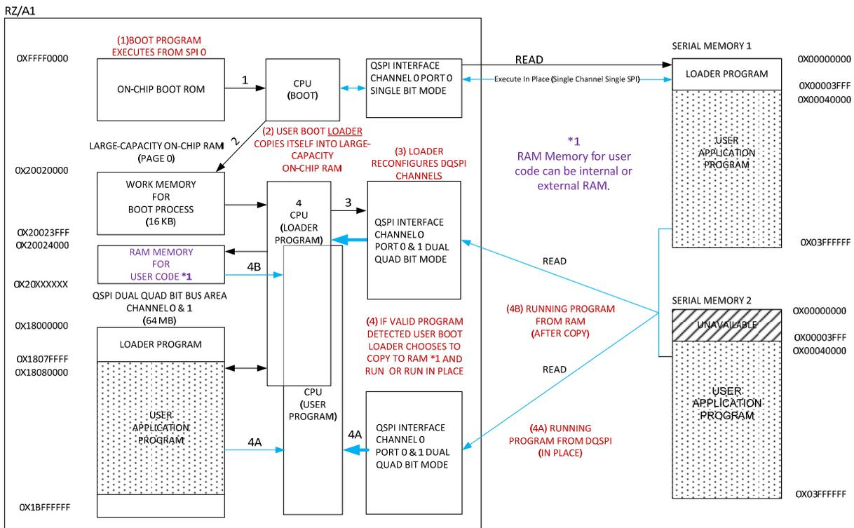
Figure 8.2: Boot process of user code stored in QSPI devices.
