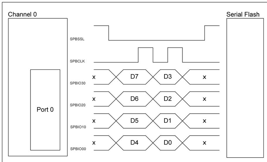
Figure 8.3: Example of a 4-bit data size using one serial flash memory.
