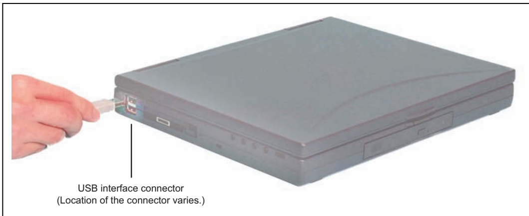
Figure 4.4 Connecting the USB interface cable (host machine side)
