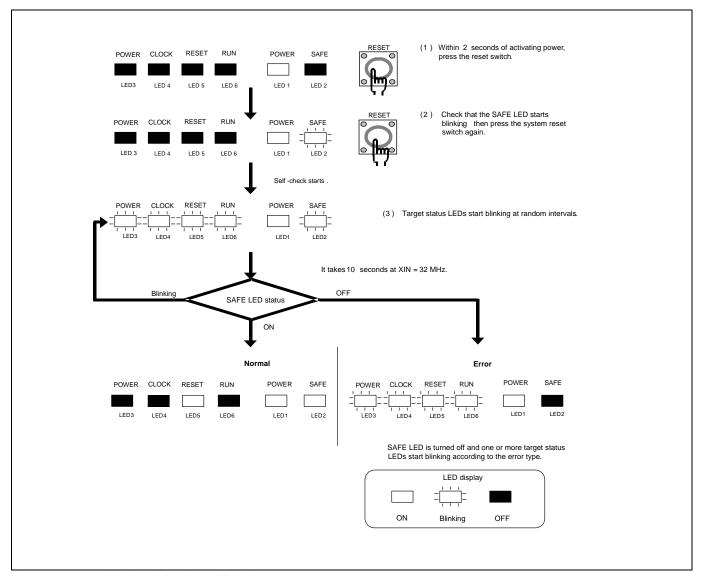
Figure 2.10 LED display during the self-check
