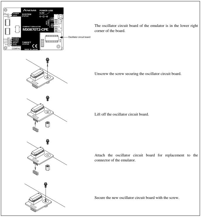
Figure 2.22 Replacing oscillator circuit boards
