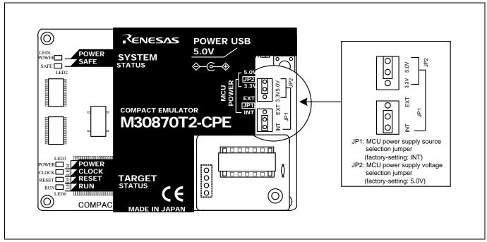
Figure 2.6 Jumper switch locations
