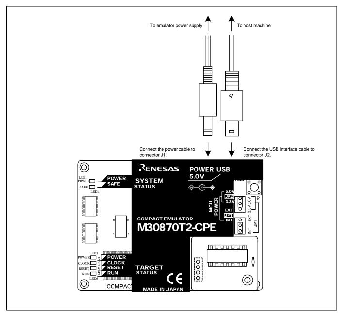
Figure 2.5 Connecting the emulator system
