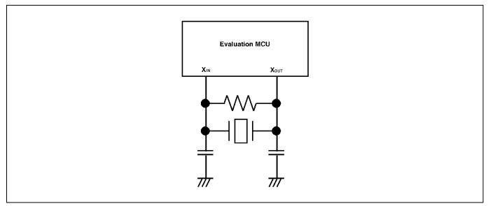
Figure 2.26 Circuit in which oscillation does not occur
