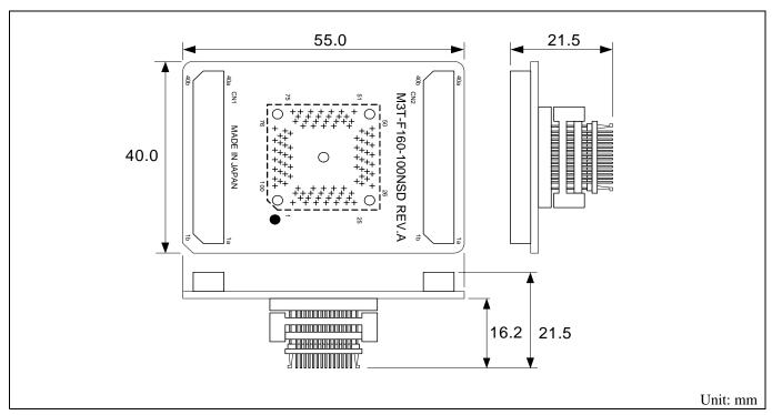
Figure 4.6 External dimensions of the M3T-F160-100NSD
