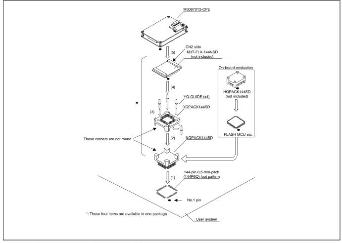
Figure 2.19 Connecting to a 144-pin 0.5-mm-pitch foot pattern
