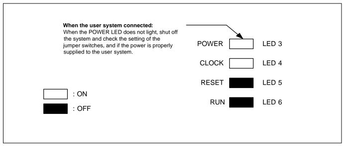
Figure 2.9 Target status LEDs display when the emulator starts up normally (when user system connected)
