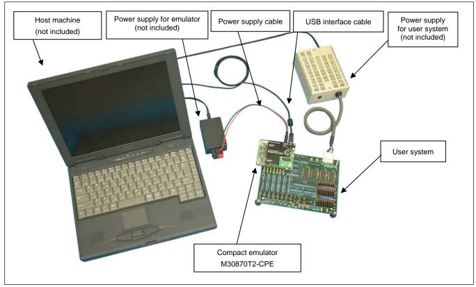
Figure 1.1 System configuration
