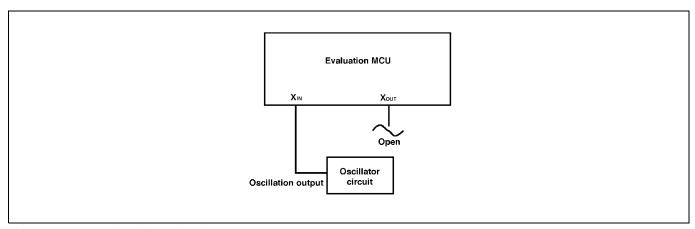
Figure 2.25 External oscillator circuit
