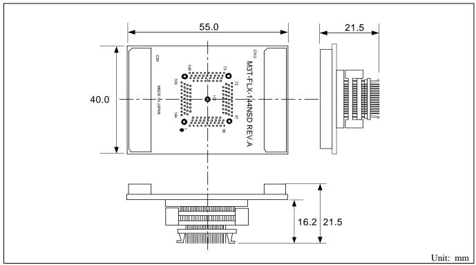
Figure 4.7 External dimensions of the M3T-FLX-144NSD
