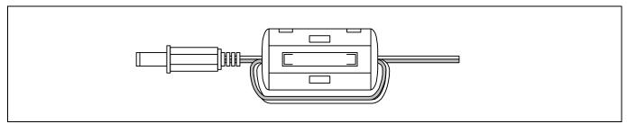
Figure 2.2 Attaching the ferrite core
