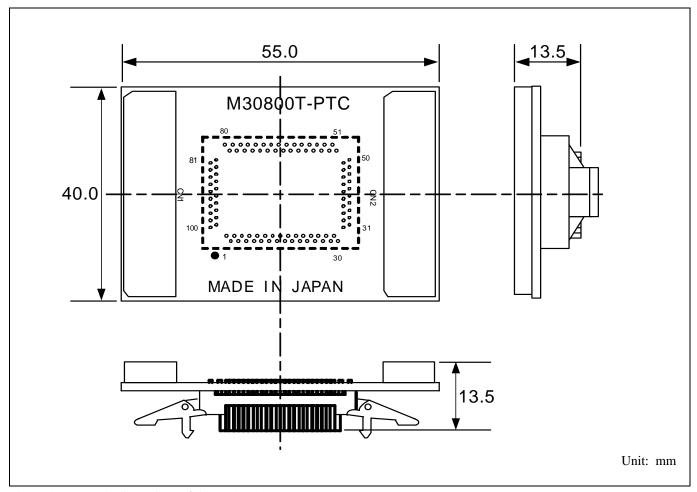
Figure 4.5 External dimensions of the M30800T-PTC
