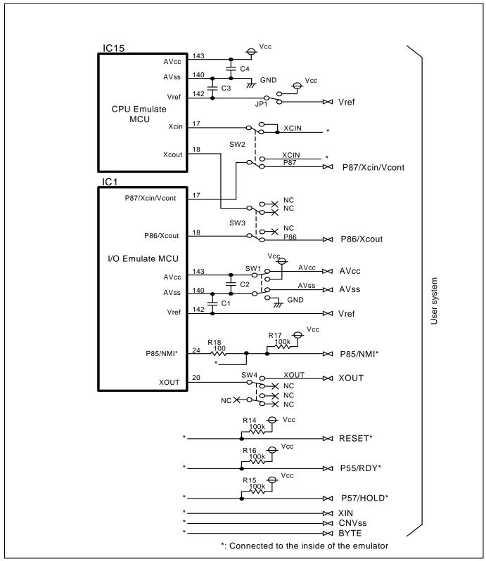
Figure 4.2 Connection diagram (when using M30870T-EPBM REV.C) (2/3)
