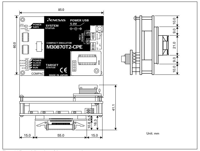
Figure 4.4 External dimensions of the compact emulator
