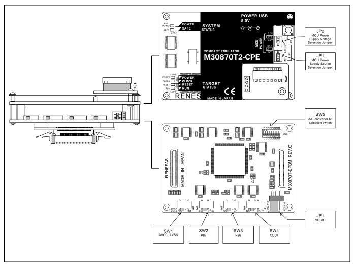
Figure 2.21 Positions of the switches (with M30870T-EPBM REV.C)
