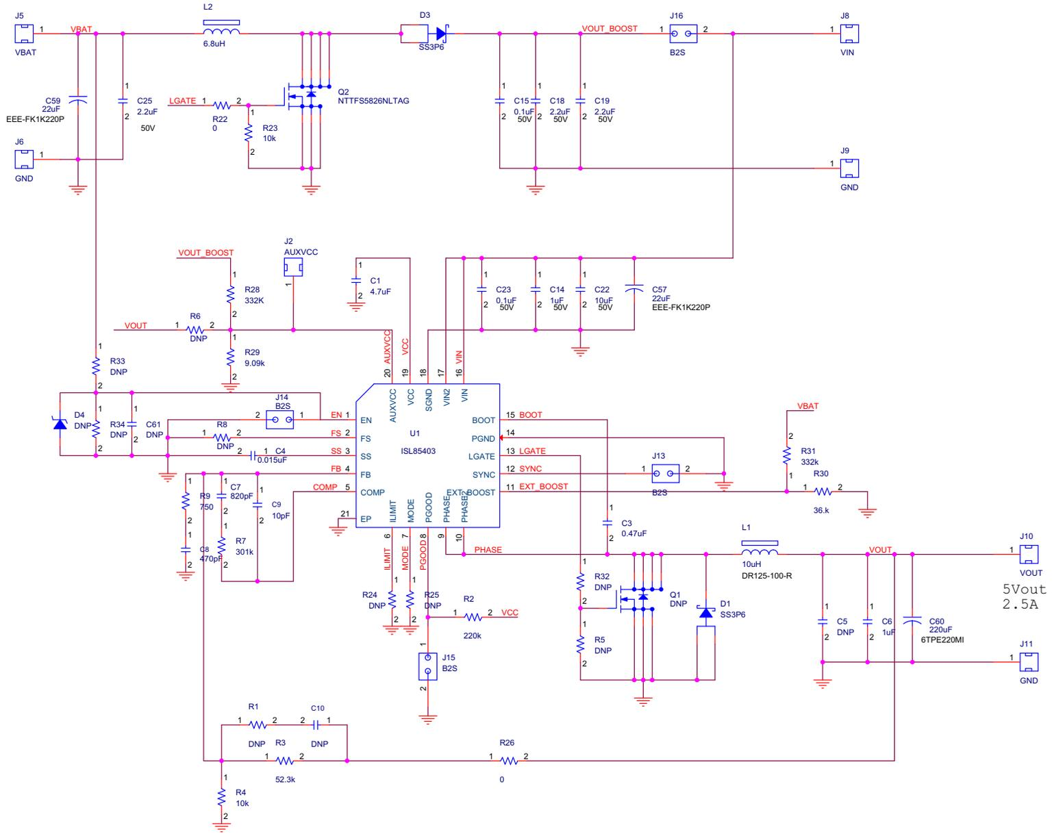
FIGURE 5. ISL85403EVAL1Z SCHEMATIC
