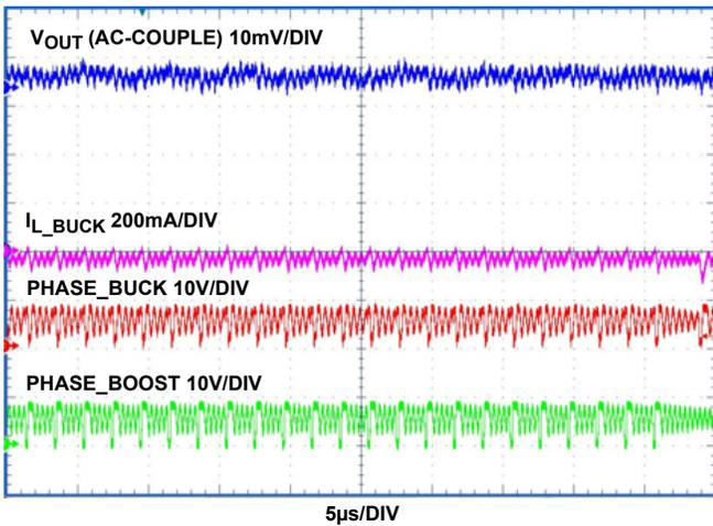
FIGURE 8. OUTPUT RIPPLE AT 0A LOAD ( $V_{IN} = 5V$ )
