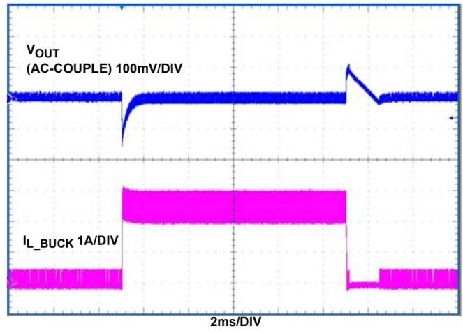
FIGURE 19. LOAD TRANSIENT RESPONSE 0A->2.5A,  $V_{IN} = 36V$
