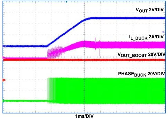
FIGURE 25. SOFT-START WITH 2Ω LOAD ( $V_{IN} = 36V$ )
