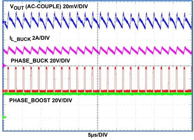
FIGURE 15. OUTPUT RIPPLE AT 2.5A LOAD ( $V_{IN} = 36V$ )
