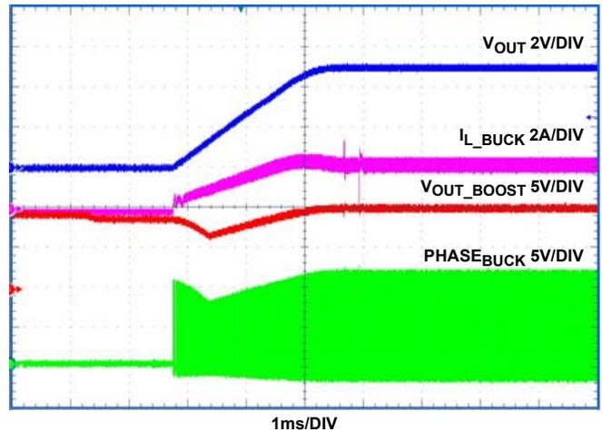
FIGURE 23. SOFT-START WITH 2Ω LOAD ( $V_{IN} = 5V$ )
