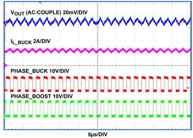
FIGURE 9. OUTPUT RIPPLE AT 2.5A LOAD ( $V_{IN} = 5V$ )
