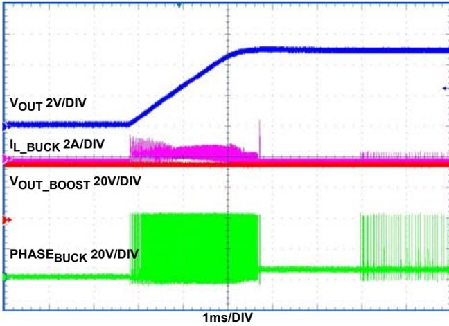
FIGURE 24. SOFT-START AT 0A LOAD ( $V_{IN} = 36V$ )
