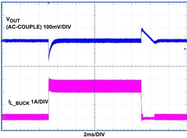
FIGURE 18. LOAD TRANSIENT RESPONSE 0A->2.5A,  $V_{IN} = 24V$
