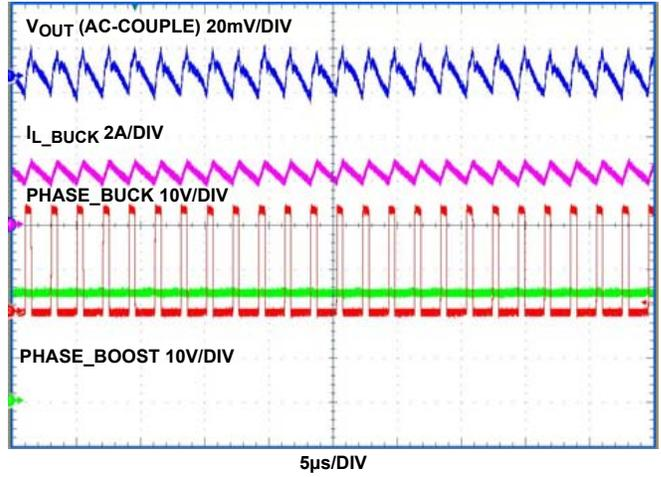
FIGURE 13. OUTPUT RIPPLE AT 2.5A LOAD ( $V_{IN} = 24V$ )
