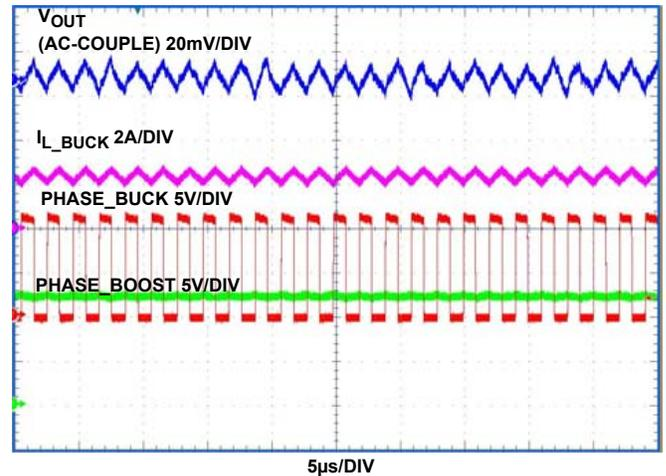
FIGURE 11. OUTPUT RIPPLE AT 2.5A LOAD ( $V_{IN} = 12V$ )
