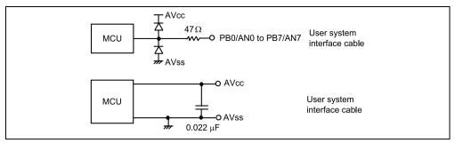
Figure 7.3 User System Interface Circuit for PB0 to PB7, AVcc and AVss Signals
