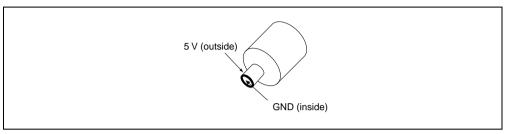
Figure 2.6 Polarity of Power Supply Plug
