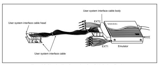
Figure 2.5 Plugging User System Interface Cable Body to Emulator
