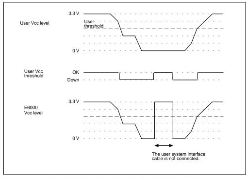
Figure 2.10 Voltage Level Monitoring (Example for Vcc = 3.3 V)
