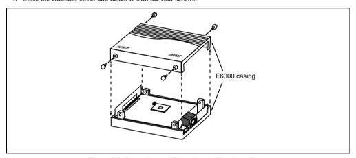
Figure 7.5 Removing and Fastening the Emulator Cover
