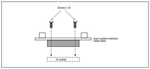
Figure 2.3 Example of Connecting User System Interface Cable Head to User System
