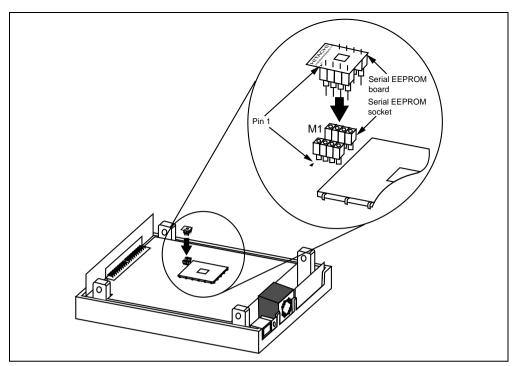
Figure 7.6 Installing Serial EEPROM Board
