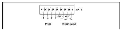
Figure 2.7 External Probe Connector 1
