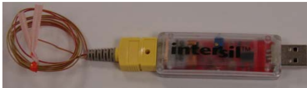
FIGURE 1. DAQ ON A STICK WITH THERMOCOUPLE
