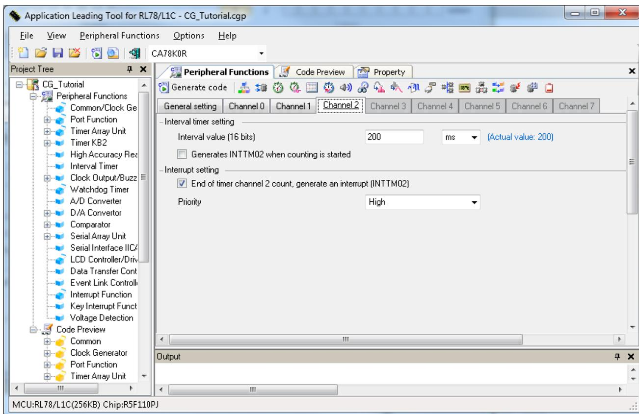
Figure 3-9 Timer Array Unit tab – Channel 2
