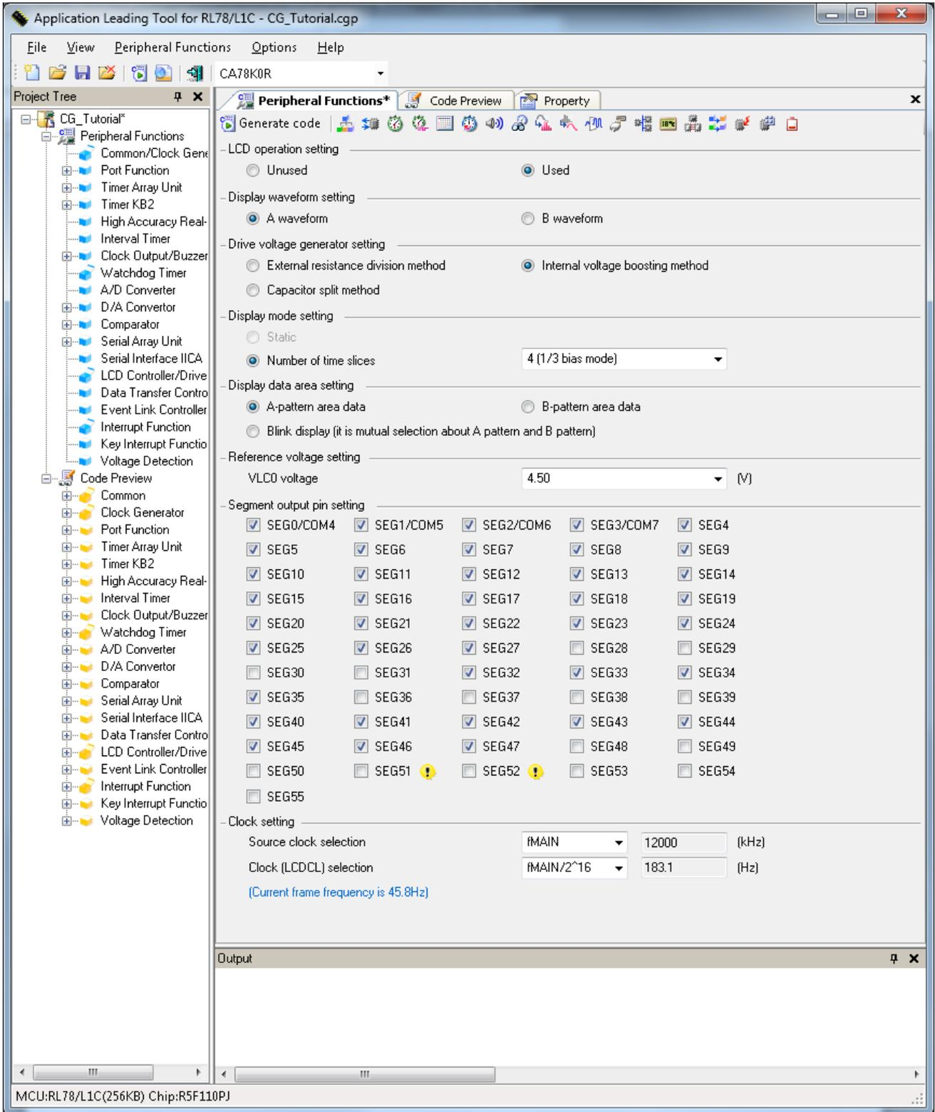
Figure 3-5 LCD Controller/Driver tab
