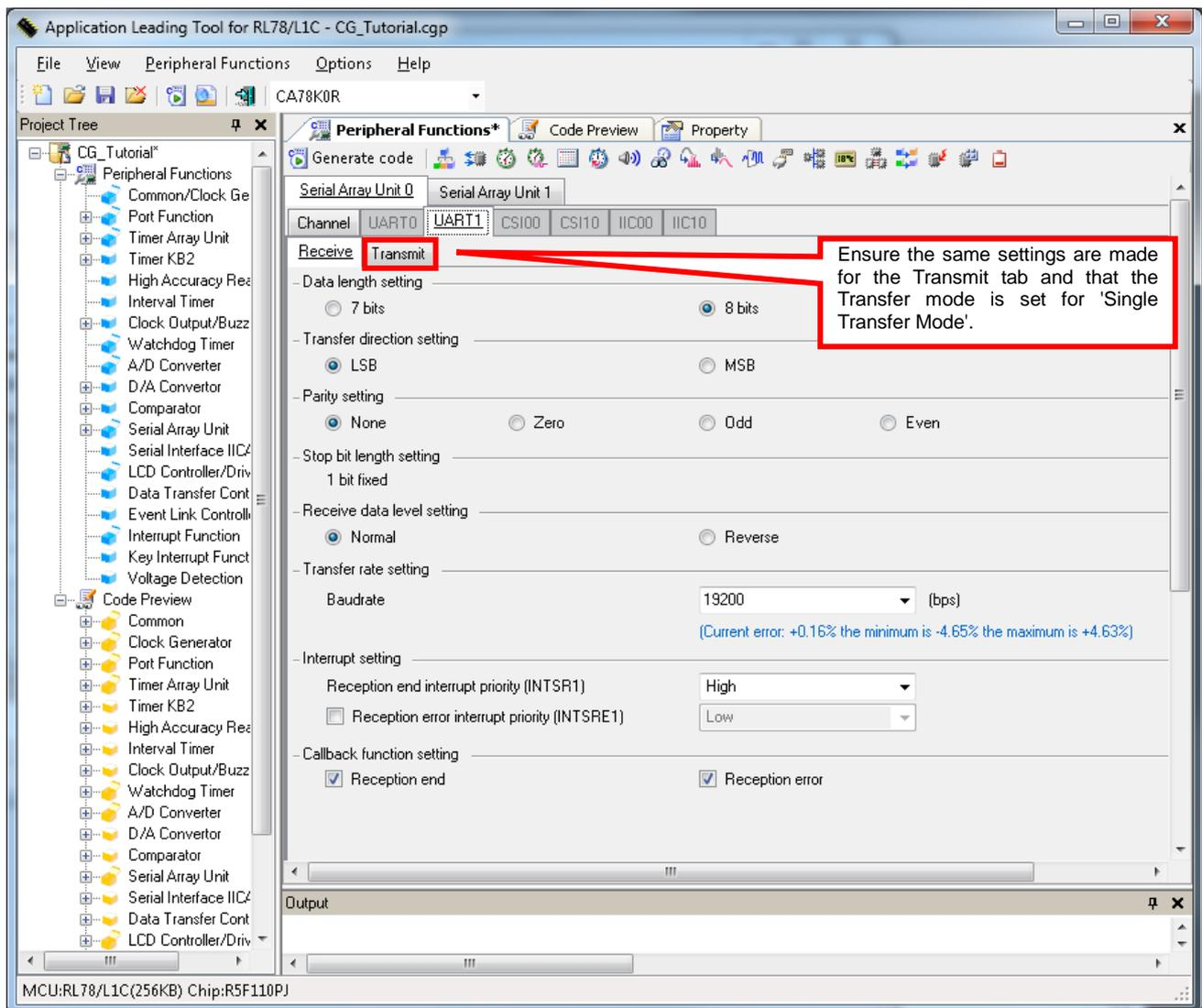
Figure 3-12 Serial Array Unit 0 tab – UART1 settings
