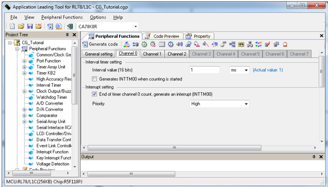
Figure 3-7 Timer Array Unit tab – Channel 0
