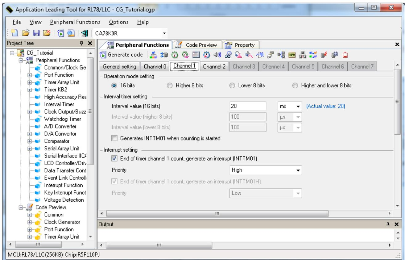
Figure 3-8 Timer Array Unit tab – Channel 1
