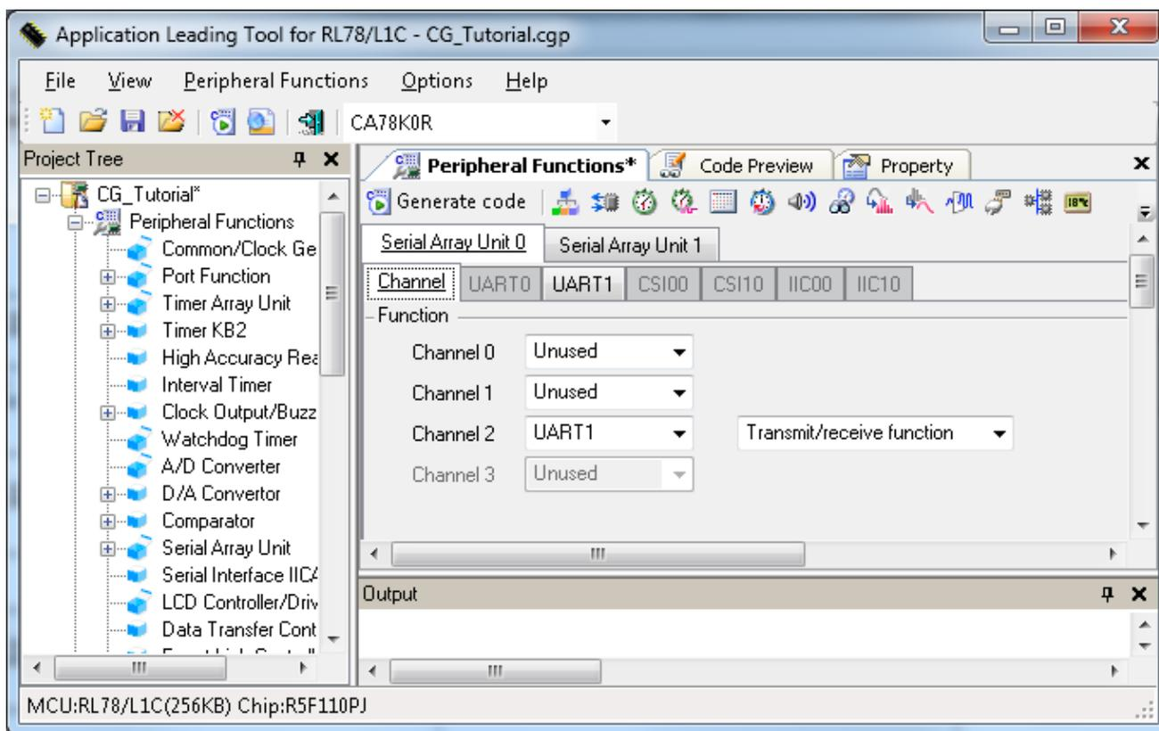
**Figure 3-11 Serial Array Unit 0 tab – Channel function selection**
