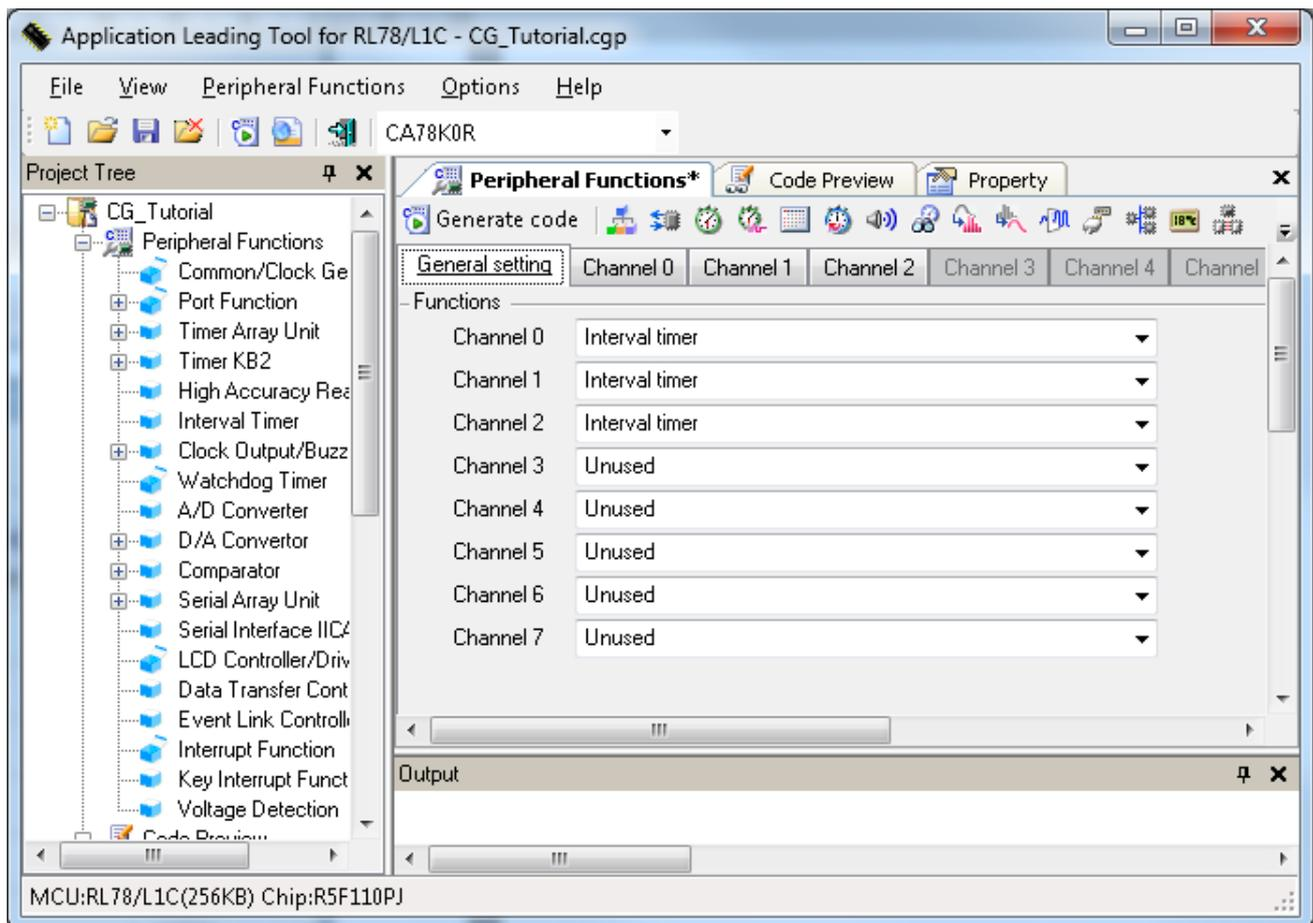
**Figure 3-6 Timer Array Unit tab – General setting**
