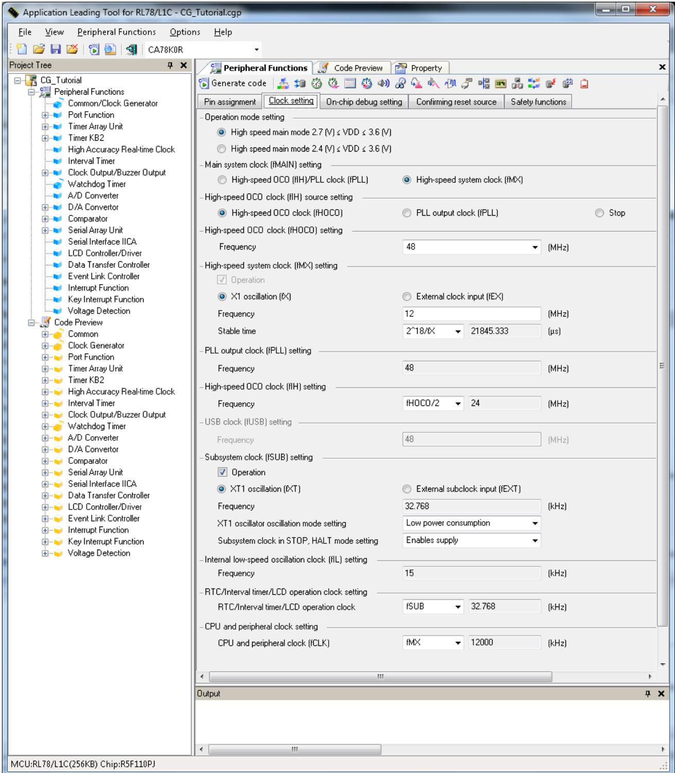
Figure 3-3 Clock setting tab
