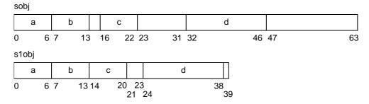
(5) Alignment condition of top structure object
