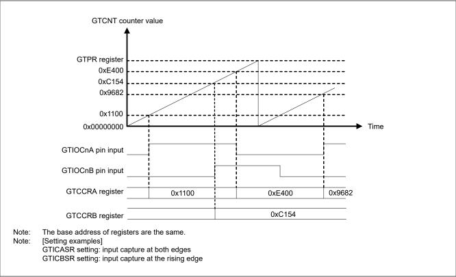
Figure 20.10 Example of input capture operation
