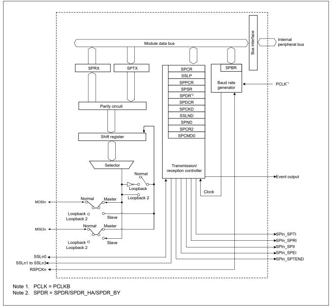
Figure 27.1 SPI block diagram
