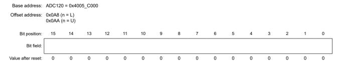
The ADWINULB and ADWINLLB registers specify the reference data when the compare window B function is used. ADWINLLB sets the lower reference for window B, and ADWINULB sets the upper reference for window B.
