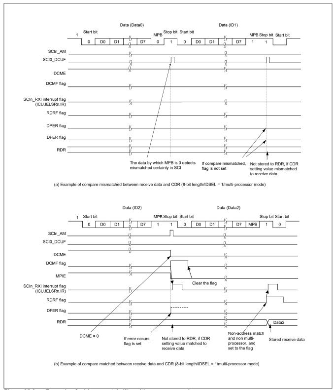
Figure 25.6 Example of address match (2) multi-processor mode
