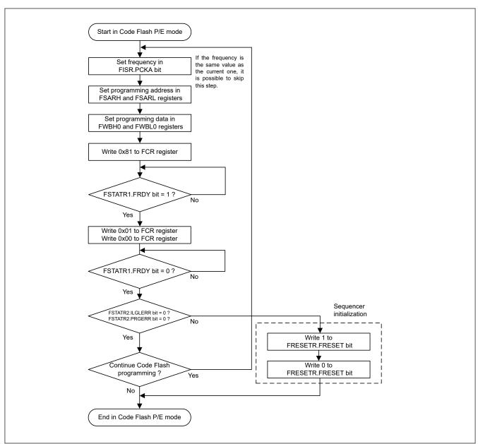
Figure 35.19 Flowchart for programming of the code flash
