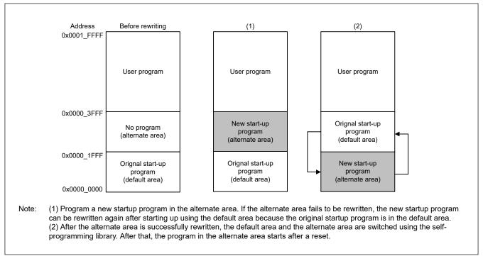
Figure 35.8 Overview of the Startup Program Protection
