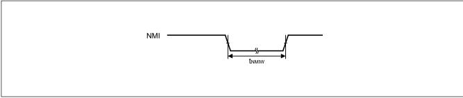
Figure 39.12 NMI interrupt input timing
