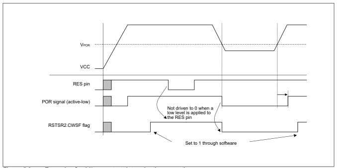
Figure 5.3 Example of cold/warm start determination operation
