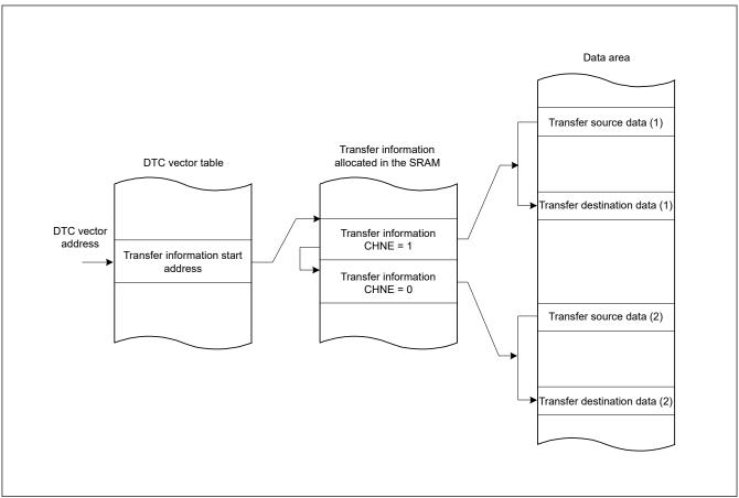
Figure 15.8 Chain transfer operation
