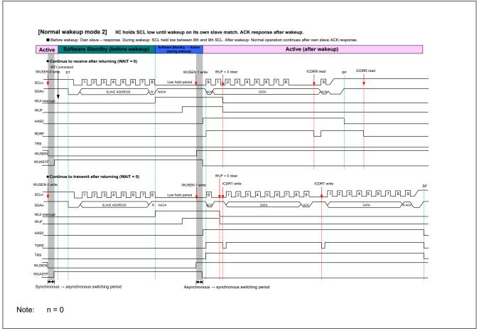
Figure 26.34 Timing of normal wakeup mode 2
