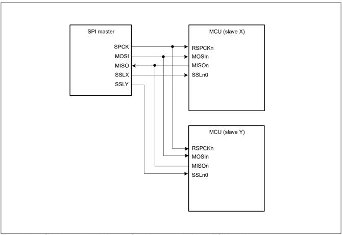
Figure 27.9 Single-master/multi-slave configuration example with the MCU as a slave
