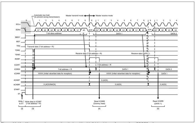
Master receive operation timing (1) with 7-bit address format when RDRFS = 0
