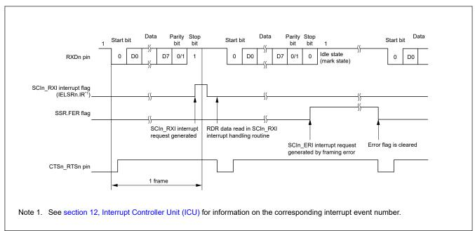
Figure 25.14 Example of SCI operation for serial reception in asynchronous mode (2) when RTS function is used, and with 8-bit data, parity bit, and 1 stop bit
