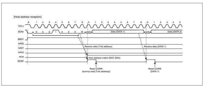
Figure 26.29 HOA flag set timing during reception of host address
