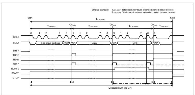
Figure 26.50 SMBus timeout measurement
