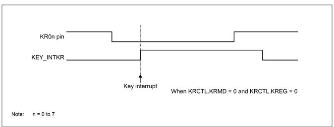
Figure 18.2 Operation of KEY\_INTKR signal when a key interrupt is input to a single channel
