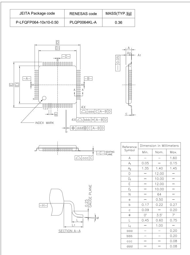
Figure 2.2 LQFP 64-pin 0.5mm pitch (2)
