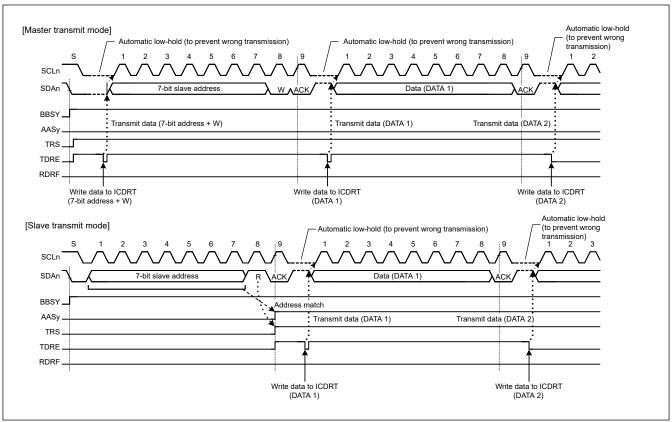
Figure 26.38 Automatic low-hold operation in transmit mode
