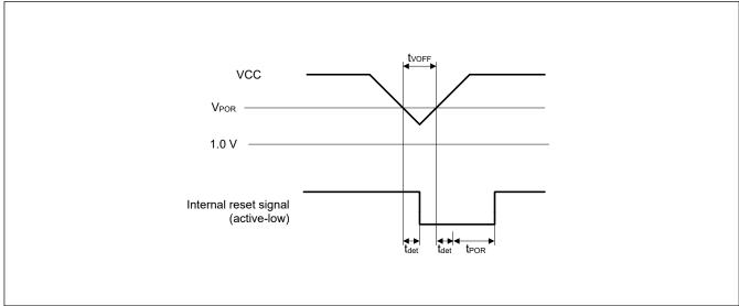
Figure 39.41 Voltage detection reset timing
