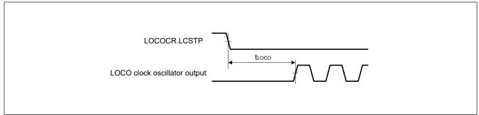
Figure 39.4 LOCO clock oscillation start timing
