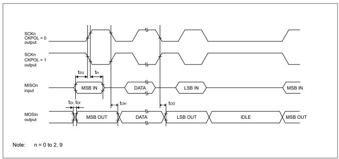
Figure 39.23 SCI simple SPI mode timing (master, CKPH = 1)
