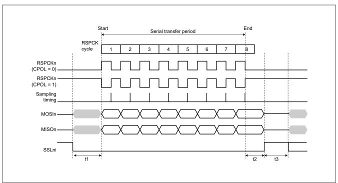
Figure 27.23 SPI transfer format when CPHA = 1
