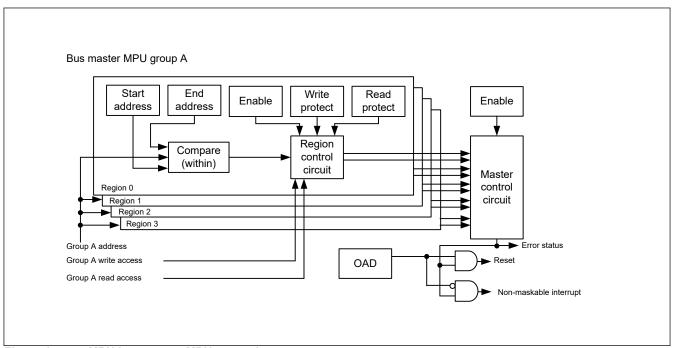
Figure 14.4 MPU bus master MPU group A
