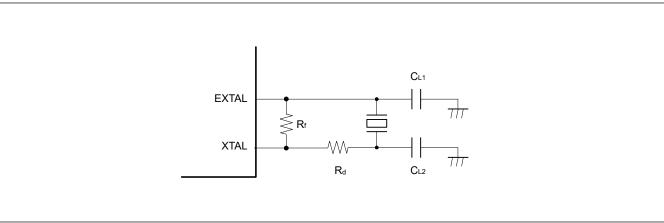
Figure 8.5 Example of crystal resonator connection
