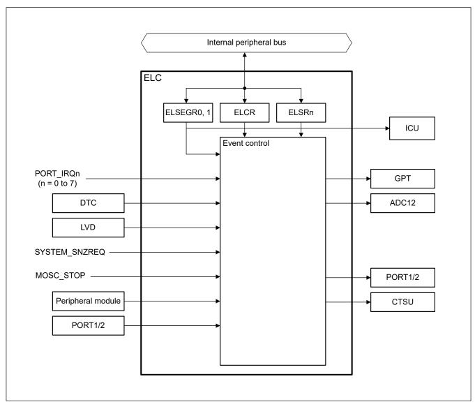
Figure 16.1 ELC block diagram
