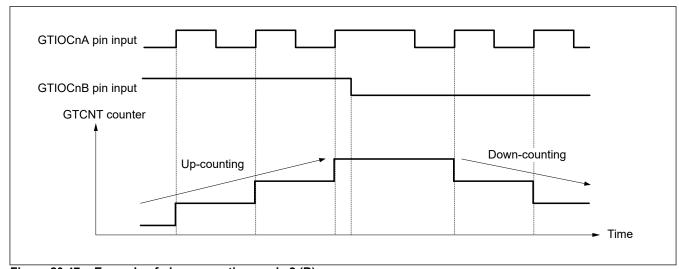
Figure 20.47 Example of phase counting mode 2 (B)
