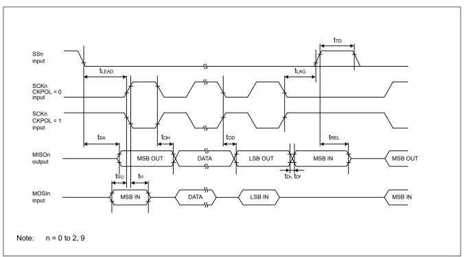
Figure 39.25 SCI simple SPI mode timing (slave, CKPH = 1)
