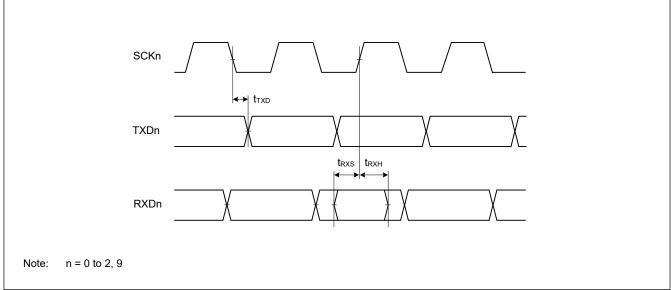
Figure 39.21 SCI input/output timing in clock synchronous mode
