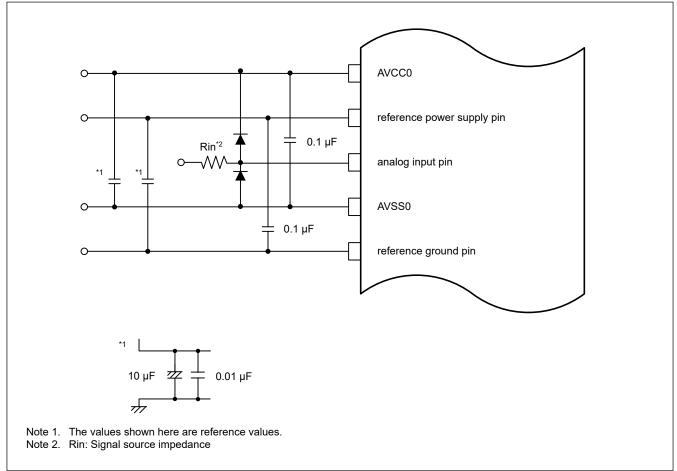
Figure 29.33 Example protection circuit for analog inputs
