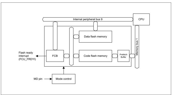
Figure 35.1 Flash memory-related modules block diagram
