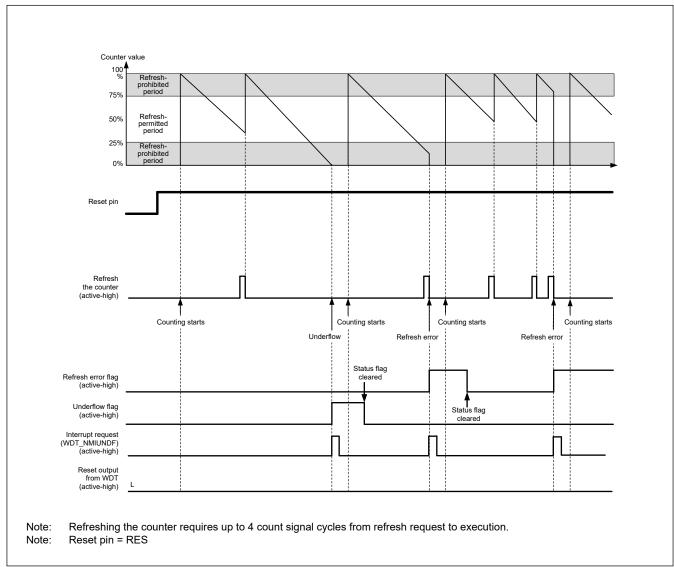
Figure 23.4 Operation example in auto start mode
