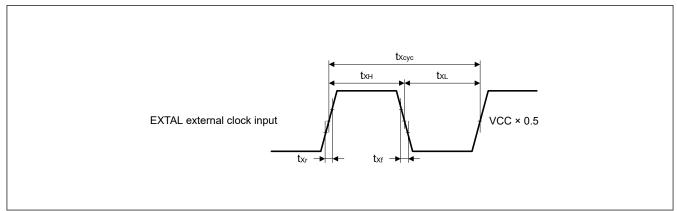
Figure 39.3 EXTAL external clock input timing
