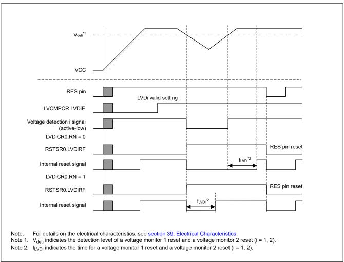
Figure 5.2 Example of operations during voltage monitor 1 and voltage monitor 2 resets
