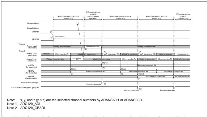
Figure 29.21 Group priority operation example 1-5: Continuously activating single scan for group B (when ADGSPCR.GBRP = 1)
