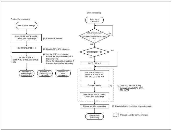
Figure 27.39 Error processing flow for slave mode
