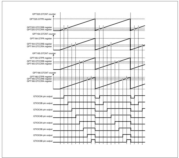
Figure 20.39 Example of synchronized PWM output
