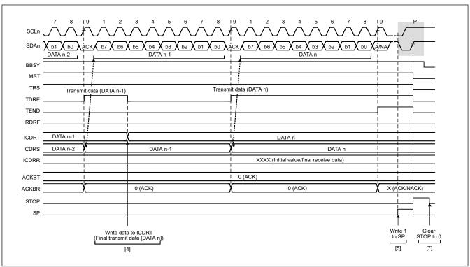
Figure 26.9 Master transmit operation timing (3)
