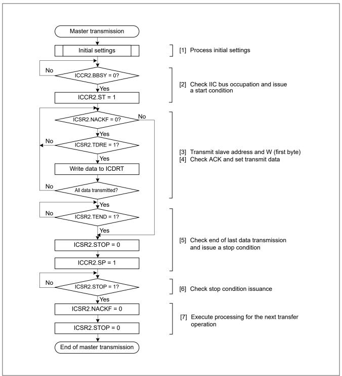
Figure 26.6 Example master transmission flow
