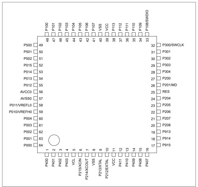
Figure 1.3 Pin assignment for LQFP 64-pin (top view)
