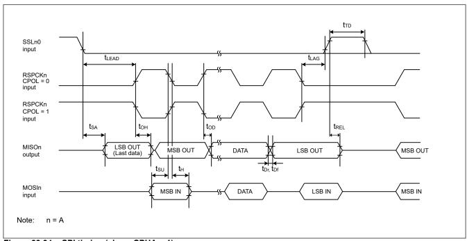
Figure 39.34 SPI timing (slave, CPHA = 1)
