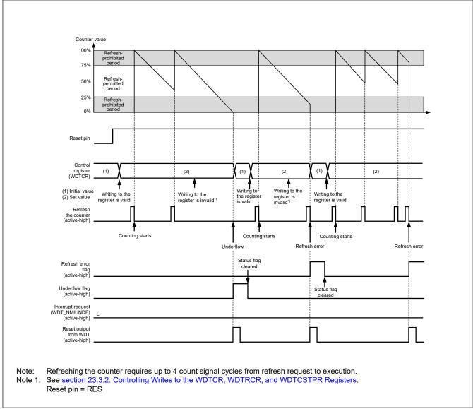
Figure 23.3 Operation example in register start mode
