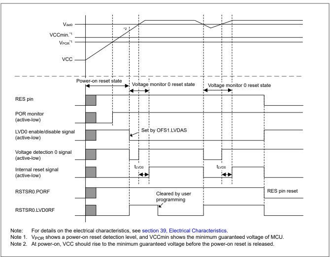
Figure 5.1 Example of operations during a power-on reset
