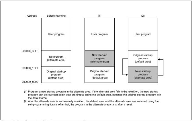
Figure 35.6 Overview of startup program protection
