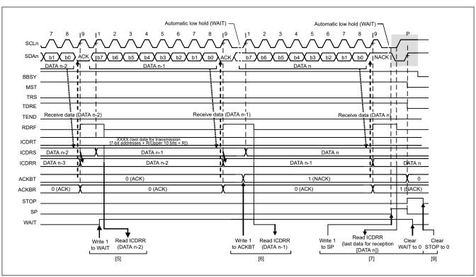
Figure 26.14 Master receive operation timing (3) when RDRFS = 0
