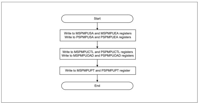
Figure 14.2 CPU stack pointer monitor register setting flow
