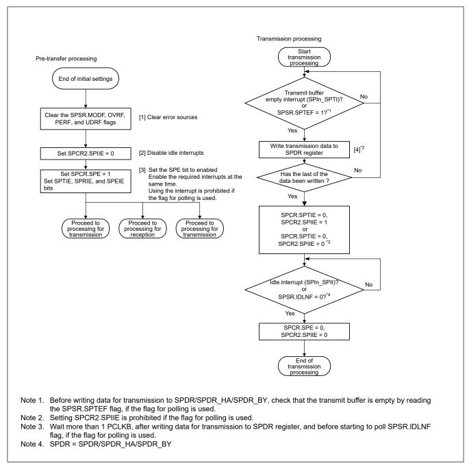
Figure 27.33 Transmission flow in master mode
