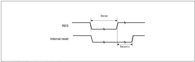
Figure 39.8 Reset input timing (1)
