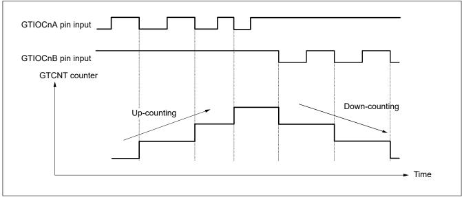
Figure 20.49 Example of phase counting mode 3 (A)
