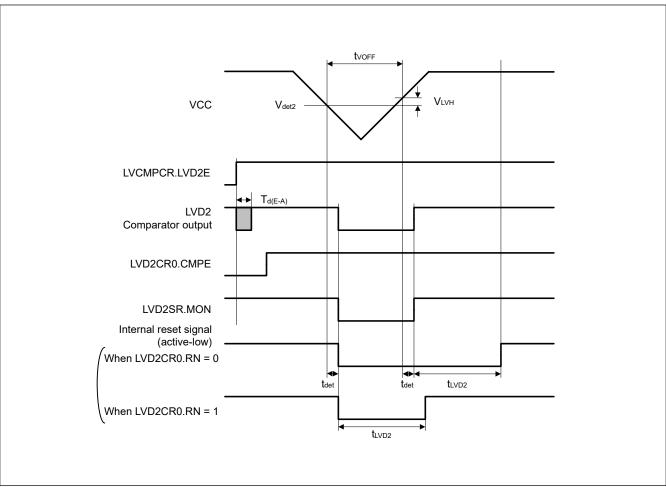
Figure 39.45 Voltage detection circuit timing (V<sub>det2</sub>)
