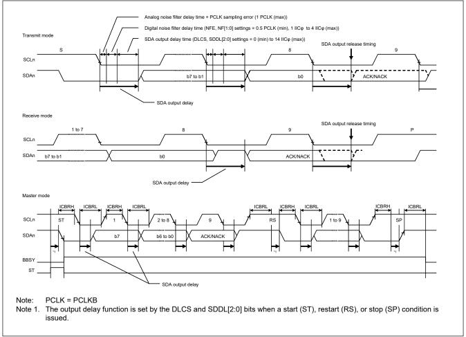
Figure 26.22 SDA output delay function
