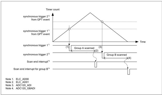
Figure 29.14 Example basic operation in group scan mode when synchronous triggers from the ELC are
