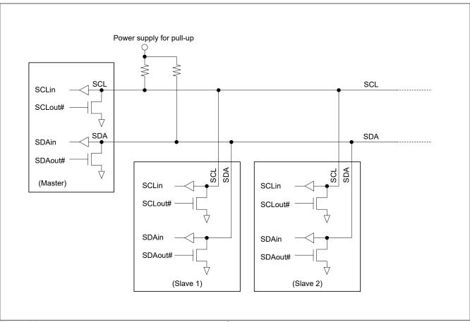
Figure 26.2 I/O pin connection to an external circuit (I<sup>2</sup>C bus configuration example)
