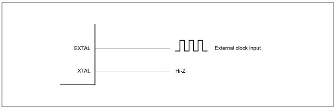
Figure 8.7 Equivalent circuit for external clock
