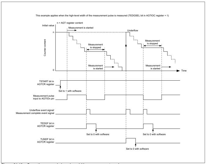
Figure 21.10 Operation example in pulse width measurement mode
