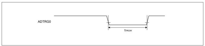
Figure 39.18 ADC12 trigger input timing
