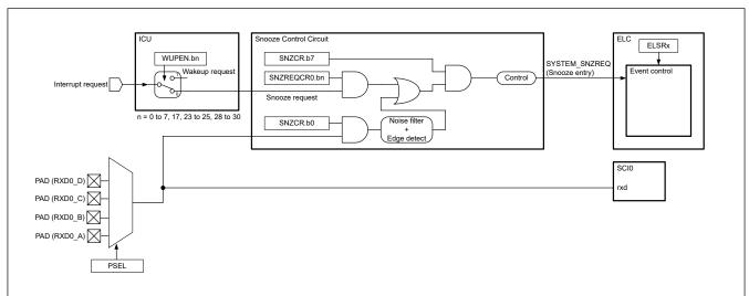
Figure 10.7 Snooze mode entry configuration
