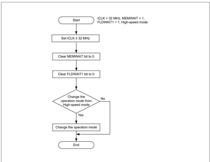
Figure 8.4 When setting ICLK ≤ 32 MHz from ICLK > 32 MHz
