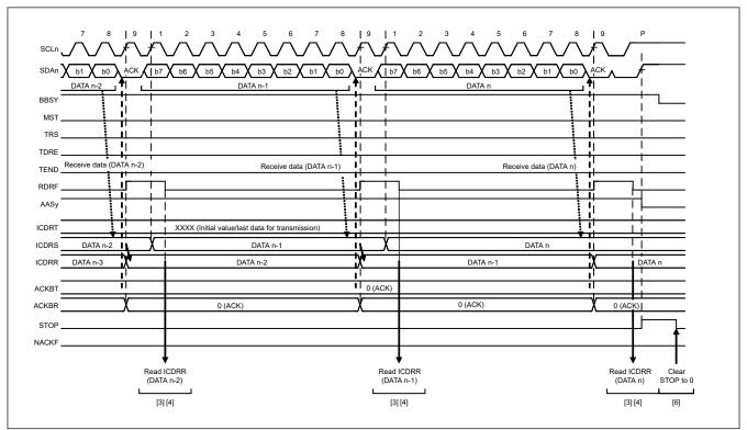
Figure 26.20 Slave receive operation timing (2) when RDRFS = 0
