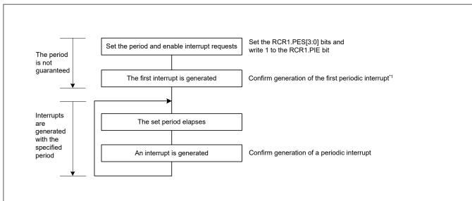
Note 1. When an interrupt generation period changes while the periodic interrupt is used, an interrupt might be generated at the completion of the setting. If the interrupt is generated immediately after the setting, the period is not guaranteed for two interrupts including the current interrupt.
