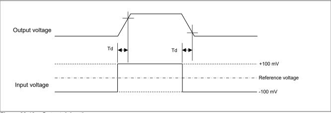
Figure 39.46 Output delay time
