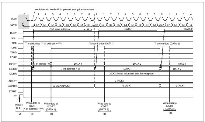
Figure 26.7 Master transmit operation timing (1) with 7-bit address format
