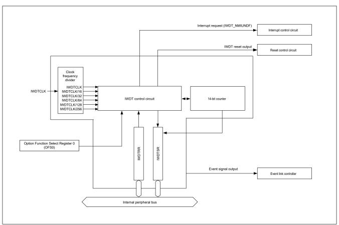
Figure 24.1 IWDT block diagram
