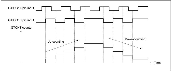
Figure 20.52 Example of phase counting mode 4
