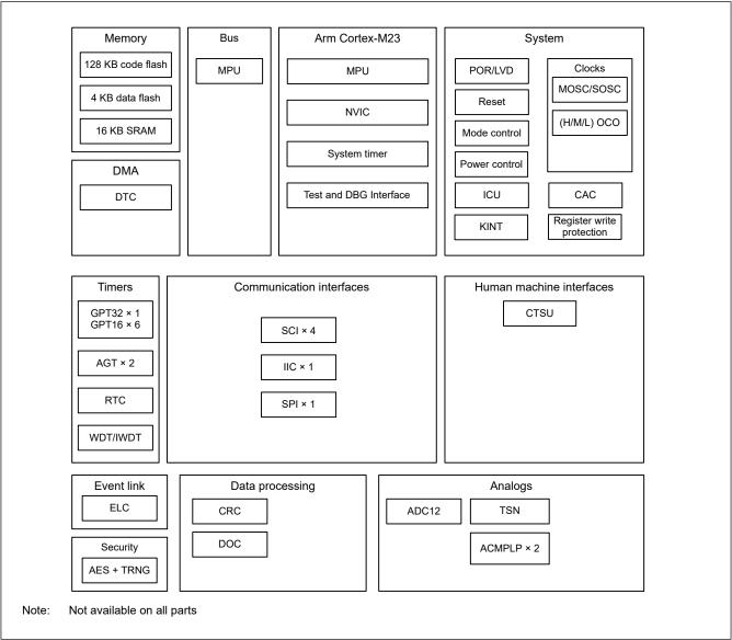
Figure 1.1 Block diagram
