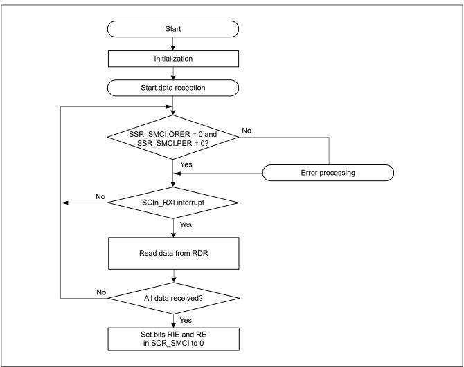
Figure 25.56 Example flow of smart card interface reception
