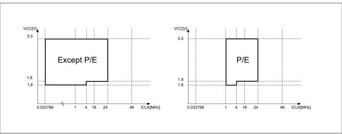
Figure 10.3 Operating voltages and frequencies in Middle-speed mode
