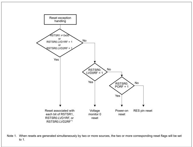
Figure 5.4 Example of reset generation source determination flow
