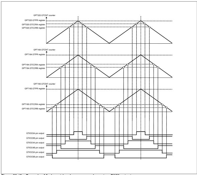
Figure 20.42 Example of 3-phase triangle-wave complementary PWM output
