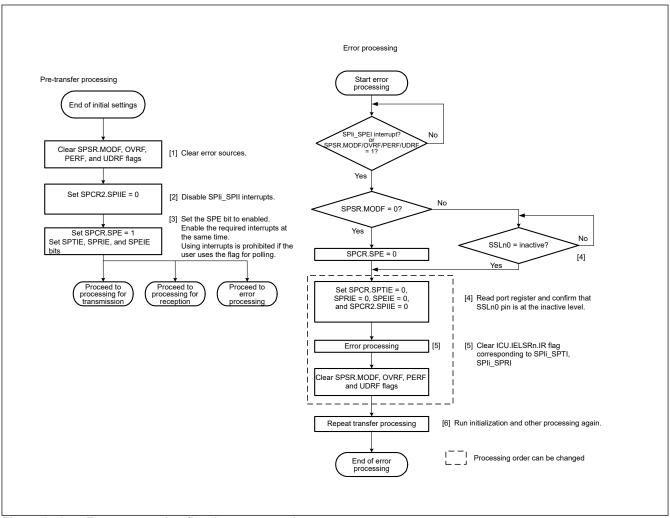
Figure 27.35 Error processing flow in master mode
