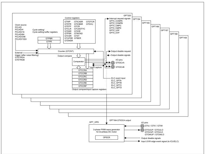
Figure 20.1 GPT block diagram
