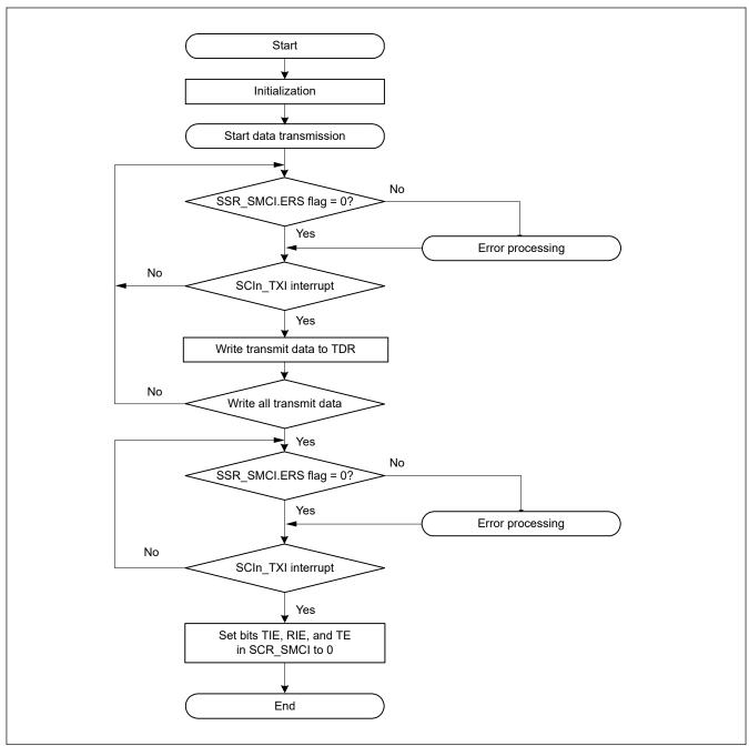
Figure 25.54 Example flow of smart card interface transmission
