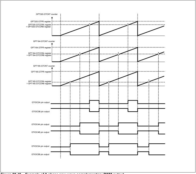
Figure 20.40 Example of 3-phase saw-wave complementary PWM output
