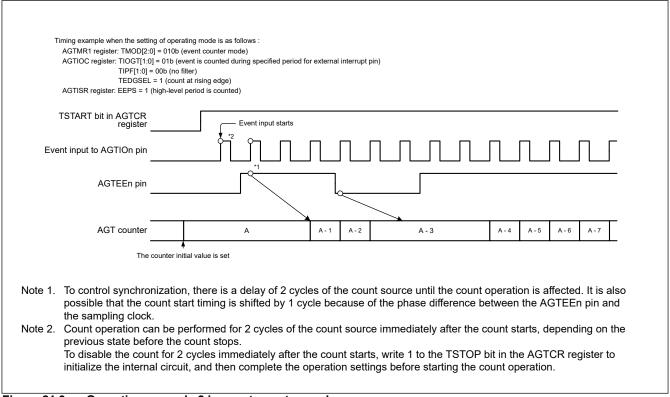
Figure 21.9 Operation example 2 in event counter mode
