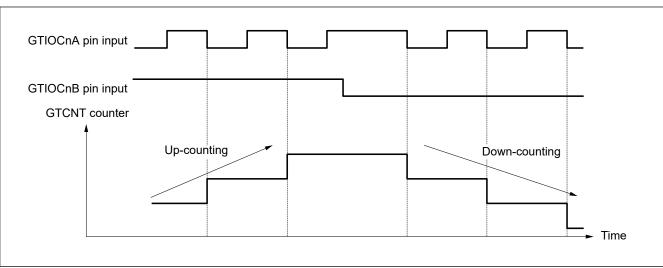
Figure 20.46 Example of phase counting mode 2 (A)
