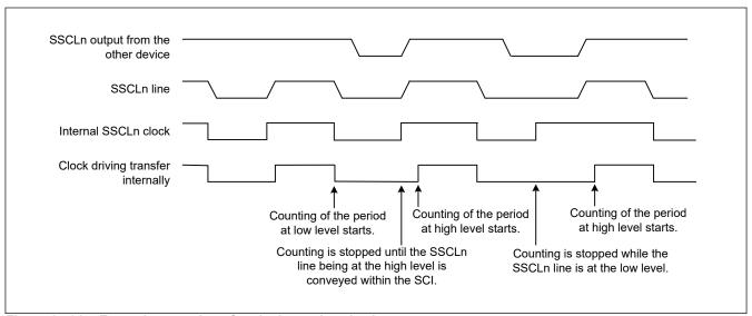
Figure 25.61 Example operations for clock synchronization
