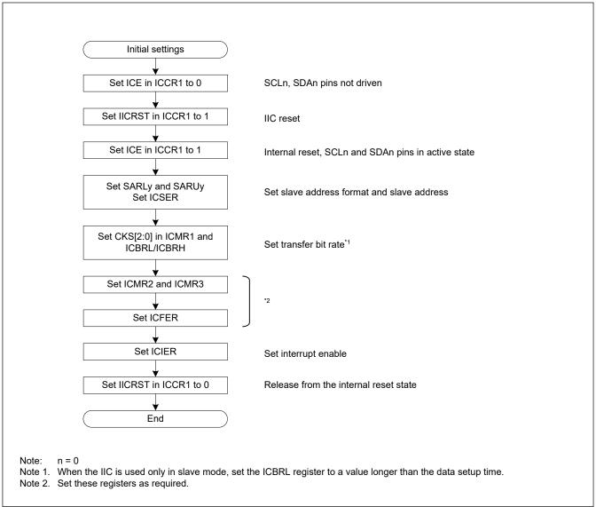
Figure 26.5 Example IIC initialization flow
