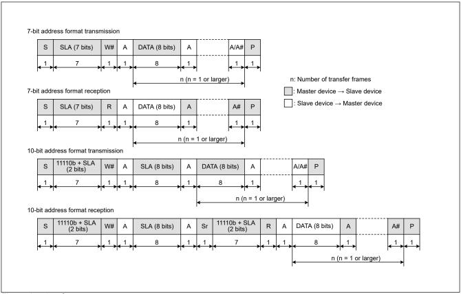
Figure 25.58 I<sup>2</sup>C bus format
