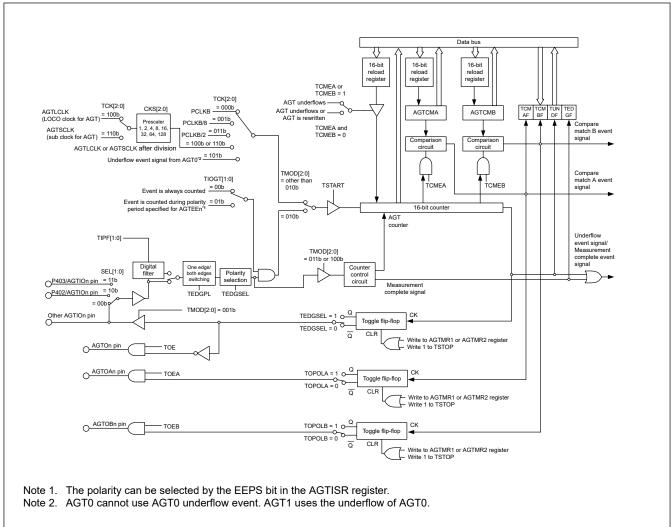
Figure 21.1 AGT block diagram
