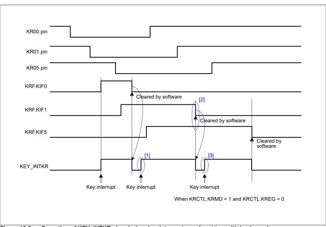
Figure 18.5 Operation of KEY\_INTKR signal when key interrupts are input to multiple channels
