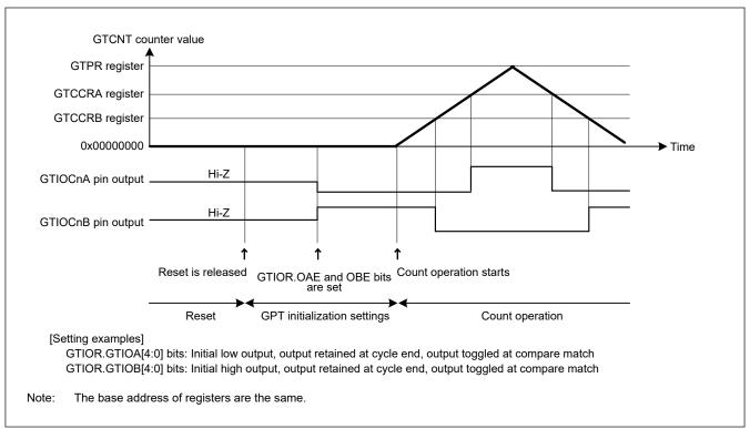
Figure 20.62 Example of pin settings after reset
