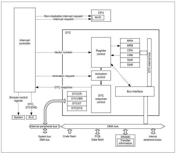
Figure 15.1 DTC block diagram
