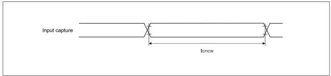
Figure 39.16 GPT input capture timing
