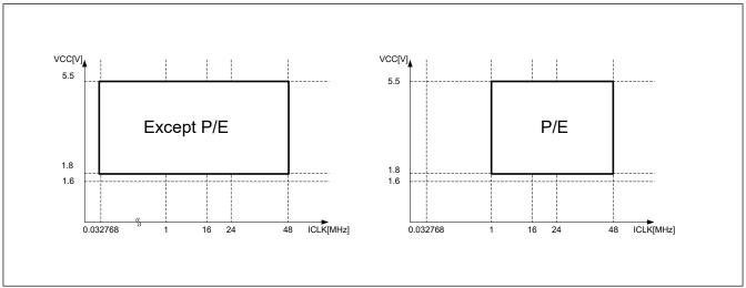
Figure 10.2 Operating voltages and frequencies in High-speed mode
