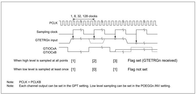
Figure 19.2 Example of digital filter operation
