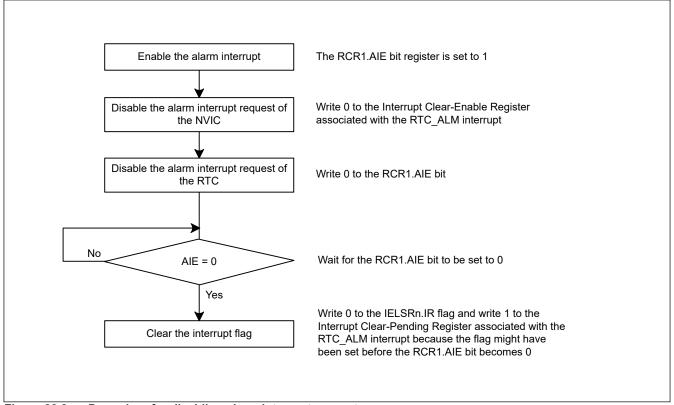
Figure 22.8 Procedure for disabling alarm interrupt request
