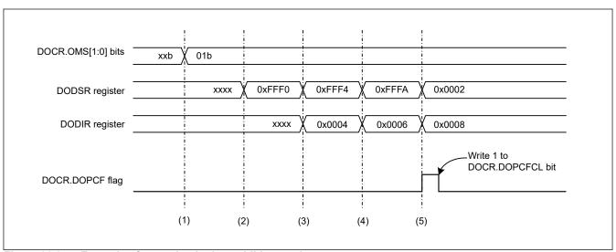
Figure 33.3 Example of operation in data addition mode
