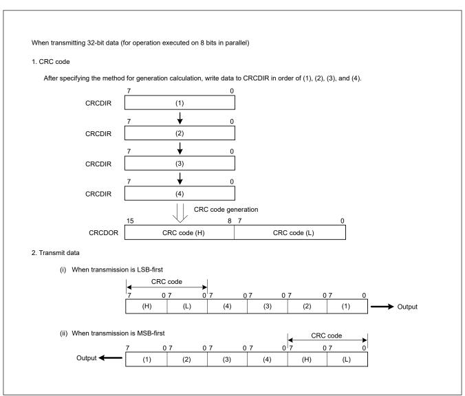
Figure 28.6 LSB-first and MSB-first data transmission
