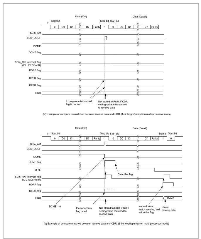
Figure 25.5 Example of address match (1) normal mode
