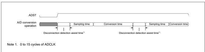
Figure 29.27 Operation of A/D conversion when disconnection detection assist function is used
