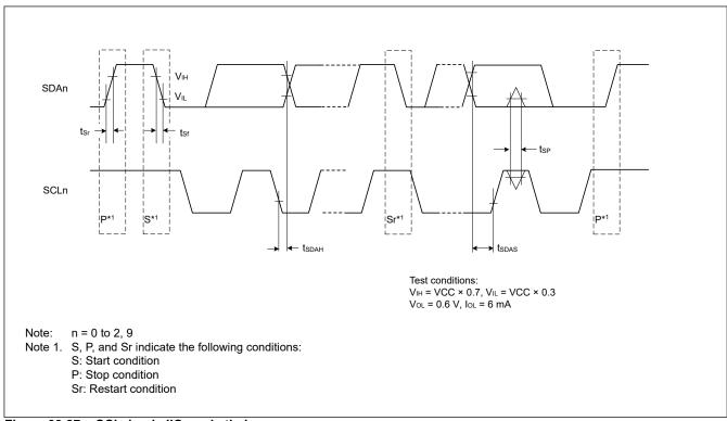
Figure 39.27 SCI simple IIC mode timing
