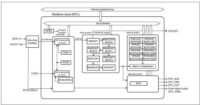
Figure 22.1 RTC block diagram
