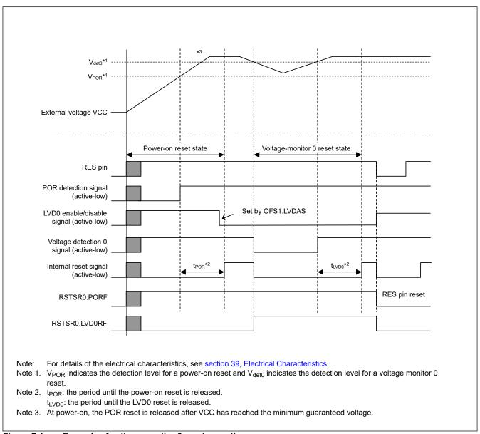
Figure 7.4 Example of voltage monitor 0 reset operation
