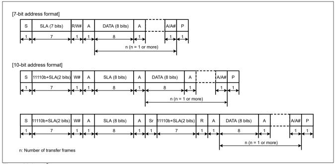
Figure 26.3 I<sup>2</sup>C bus format
