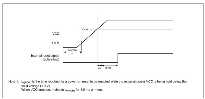
Figure 39.42 Power-on reset timing
