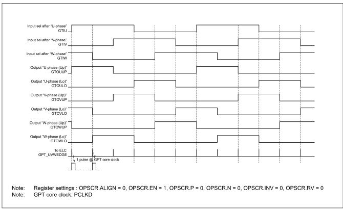
Figure 20.56 Example of 6-phase level output operation
