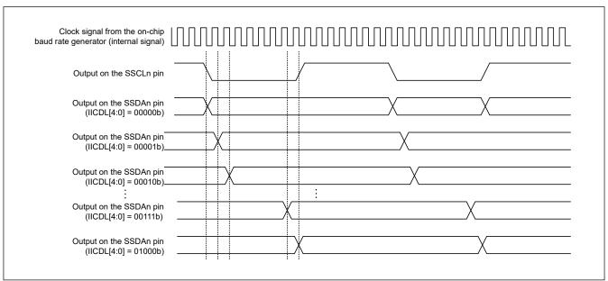
Figure 25.62 Timing of delays in SDAn output
