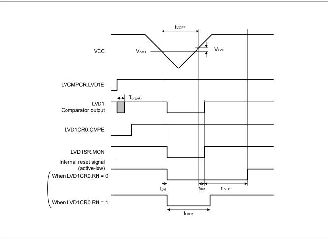
Figure 39.44 Voltage detection circuit timing (V<sub>det1</sub>)
