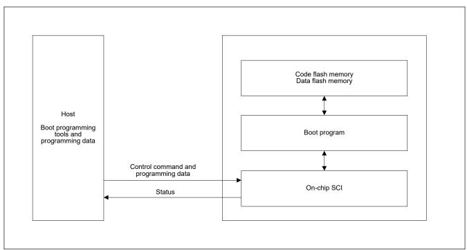
Figure 35.10 System configuration in SCI boot mode
