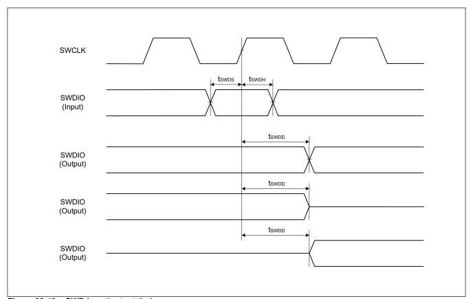
Figure 39.48 SWD input/output timing
