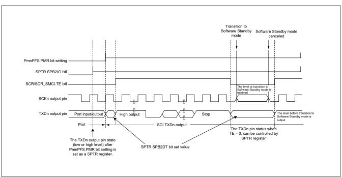
Figure 25.73 Port pin states during transition to Software Standby mode with internal clock and asynchronous transmission
