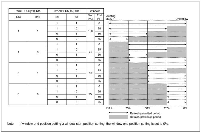
Figure 24.2 IWDTRPSS[1:0] and IWDTRPES[1:0] bit settings and refresh-permitted period
