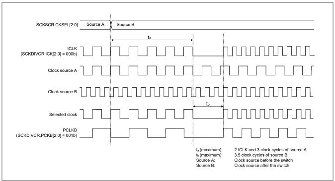
Figure 8.13 Timing of clock source switching
