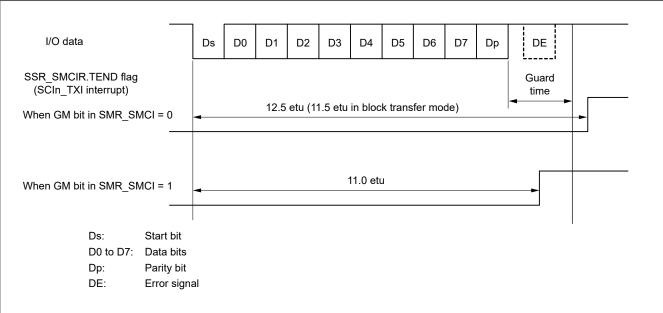
Figure 25.53 SSR.TEND flag generation timing during transmission
