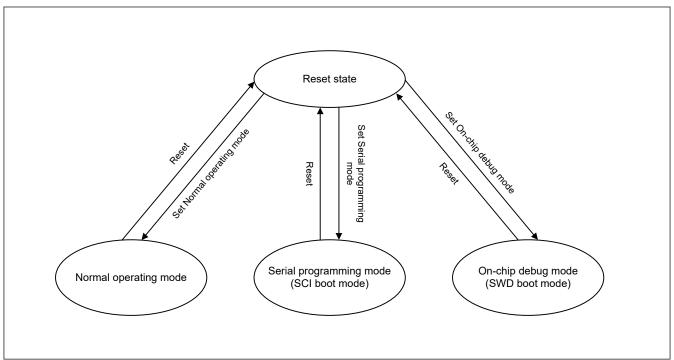
Figure 35.4 Mode transitions associated with flash memory
