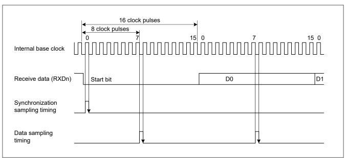
Figure 25.3 Receive data sampling timing in asynchronous mode
