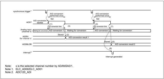
Figure 29.10 Example operation in single scan mode when double-trigger mode is selected and the analog input (channel x) is duplicated
