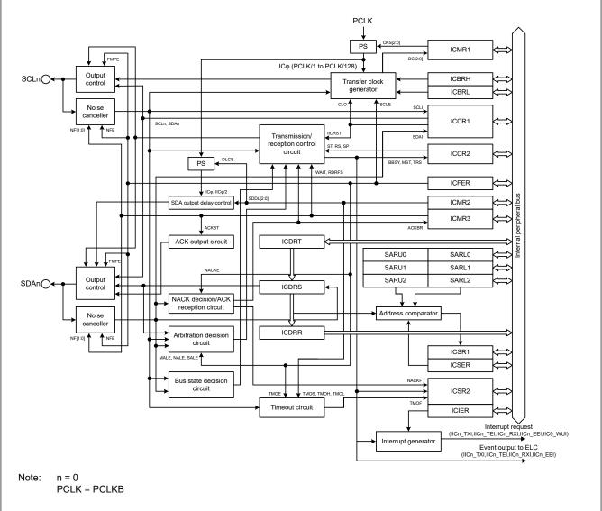
Figure 26.1 IIC block diagram
