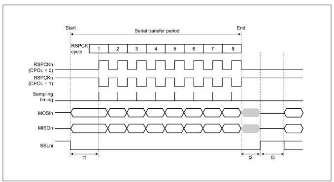
Figure 27.22 SPI transfer format when CPHA = 0
