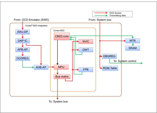
Figure 2.1 Cortex-M23 block diagram
