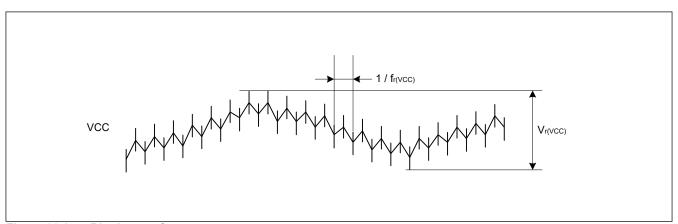
Figure 39.2 Ripple waveform
