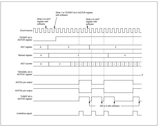
Figure 21.7 Operation example in pulse output mode
