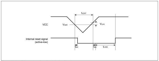
Figure 39.43 Voltage detection circuit timing (V<sub>det0</sub>)
