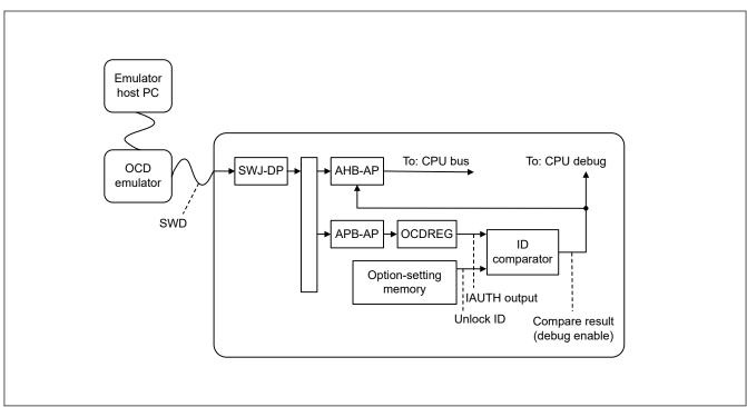
Figure 2.3 SWD Authentication mechanism block diagram
