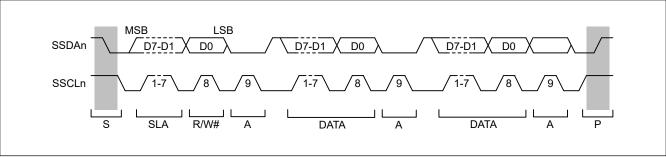
Figure 25.59 I<sup>2</sup>C bus timing when SLA is 7 bits
