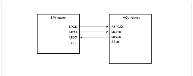
Figure 27.12 Clock synchronous master/slave configuration example with the MCU as a slave and CPHA = 1
