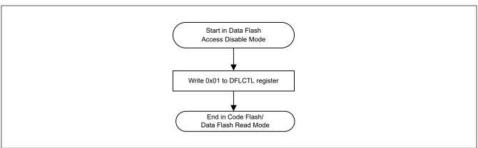
Figure 35.14 Mode transitions to read mode from data flash access disable mode
