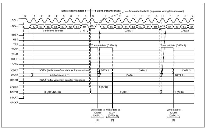
Figure 26.16 Slave transmit operation timing (1) with 7-bit address format
