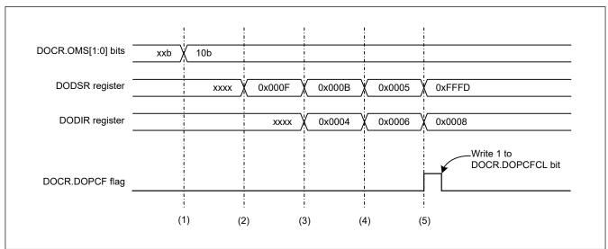
Figure 33.4 Example of operation in data subtraction mode
