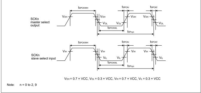
Figure 39.22 SCI simple SPI mode clock timing
