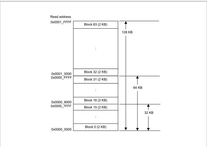
Figure 35.2 Mapping of the code flash memory
