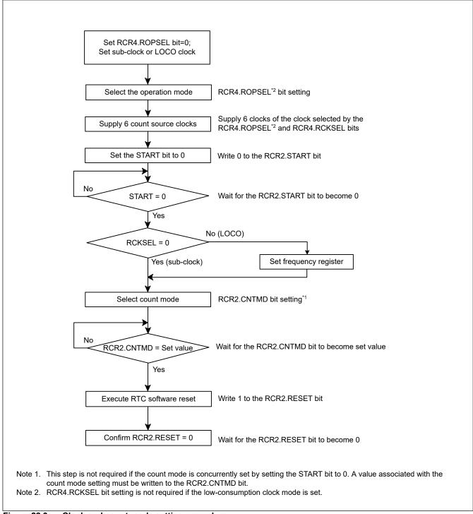
Figure 22.3 Clock and count mode setting procedure
