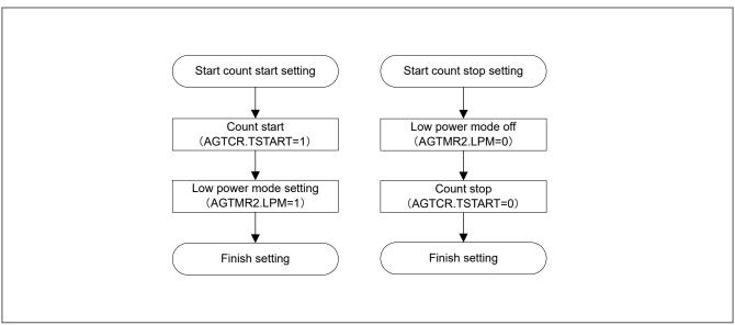
Figure 21.2 LPM how to write flow chart
