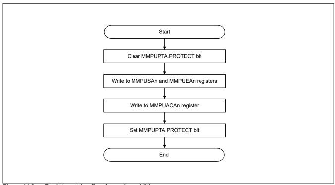
Figure 14.8 Register setting flow for region addition
