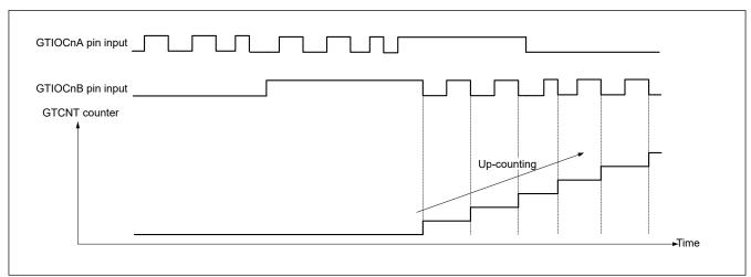
Figure 20.54 Example of phase counting mode 5 (B)
