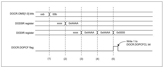
Figure 33.2 Example of operation in data comparison mode
