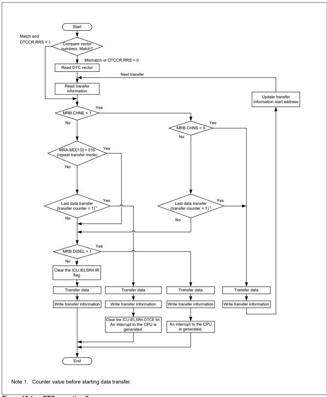
Figure 15.4 DTC operation flow
