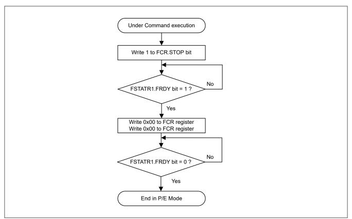
Figure 35.31 Simple flowchart for the forced stop procedure
