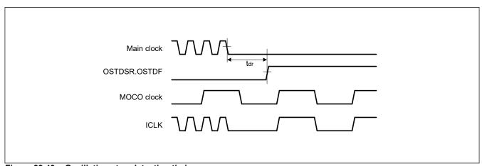
Figure 39.40 Oscillation stop detection timing
