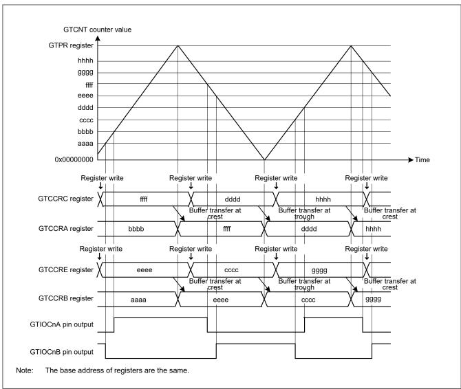
Figure 20.22 Example of triangle-wave PWM mode 2 operation with buffer operation, low output from the GTIOCnA pin and high output from the GTIOCnB pin at count start, output toggled at GTCCRA/GTCCRB compare match, and output retained at cycle end
