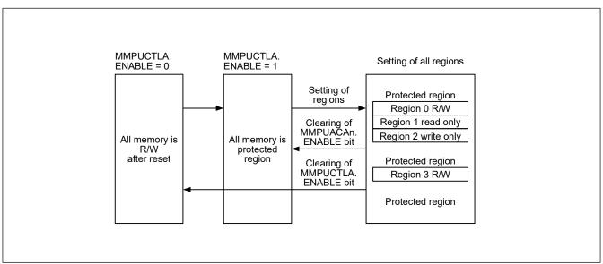
Figure 14.5 Use case of bus master MPU
