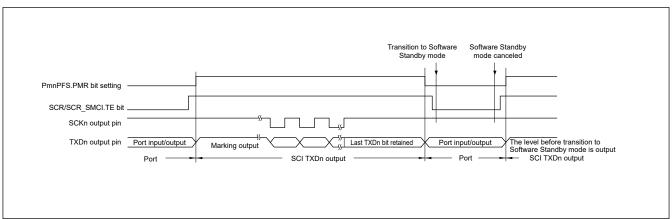
Figure 25.74 Port pin states during transition to Software Standby mode with internal clock and clock synchronous transmission
