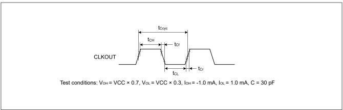
Figure 39.36 CLKOUT output timing
