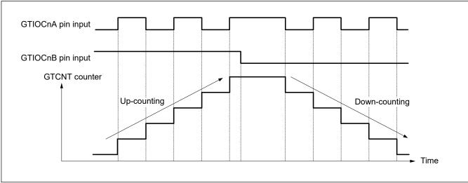
Figure 20.48 Example of phase counting mode 2 (C)
