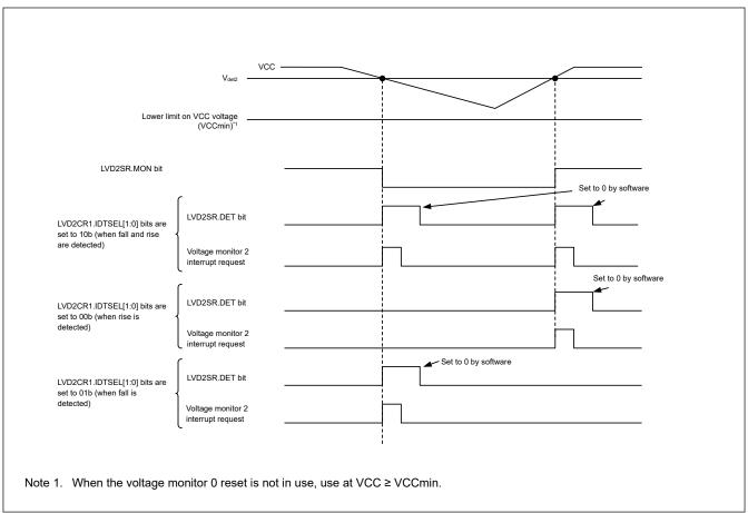
Figure 7.6 Example of voltage monitor 2 interrupt operation
