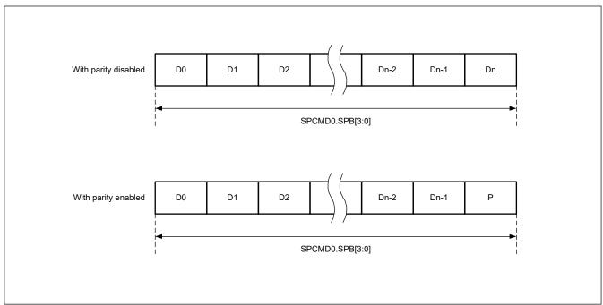
Figure 27.13 Data format with parity disabled and enabled
