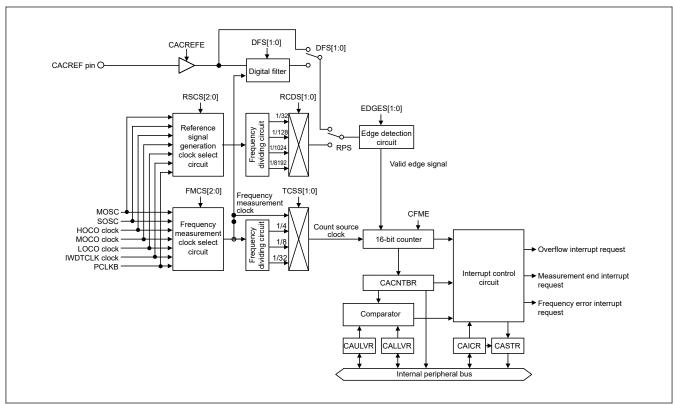
Figure 9.1 CAC block diagram
