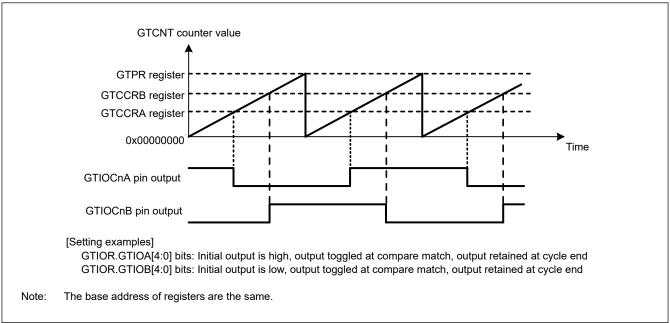
Figure 20.8 Example of toggled output operation (1)
