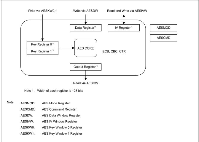
Figure 36.1 Module construction of AES engine
