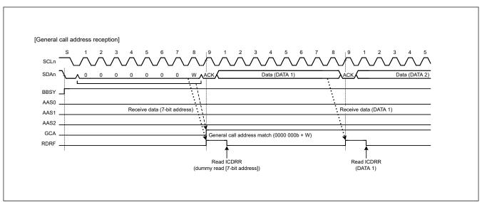
Figure 26.27 Timing of GCA flag setting during reception of general call address
