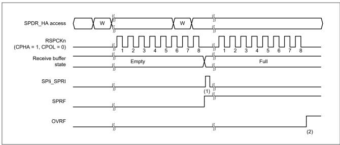
Figure 27.24 Operation example when SPCR.TXMD = 0
