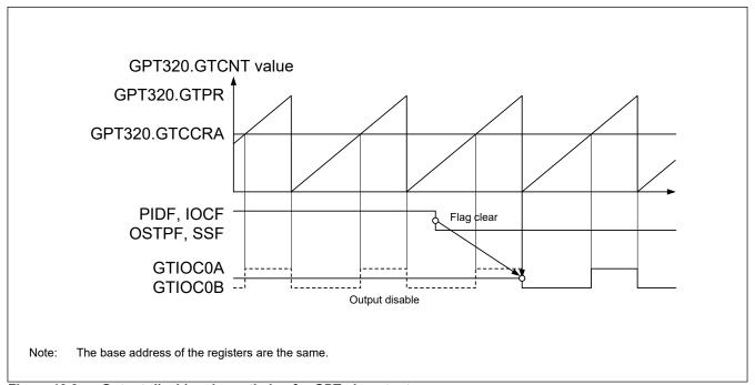
Figure 19.3 Output-disable release timing for GPT pin outputs
