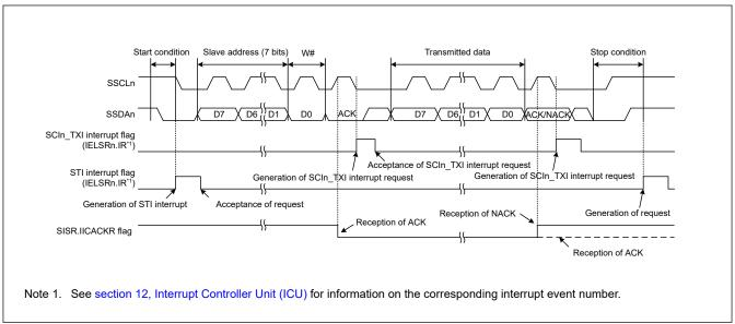
Figure 25.63 Example 1 of operations for master transmission in simple IIC mode with 7-bit slave addresses, transmission interrupts, and reception interrupts
