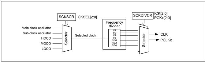
Figure 8.12 Block diagram of clock source selector
