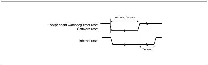
Figure 39.9 Reset input timing (2)
