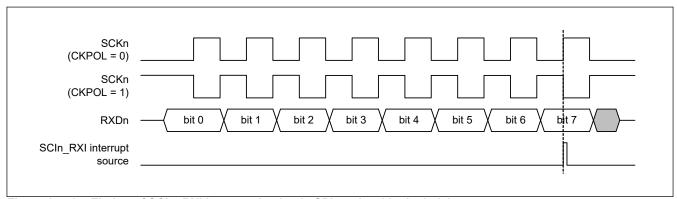
Figure 25.78 Timing of SCIn\_RXI interrupt in simple SPI mode with clock delay
