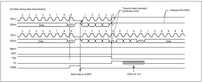
Figure 26.44 Example of slave arbitration-lost detection when SALE = 1
