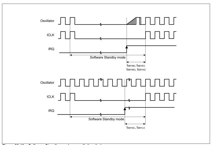
Figure 39.10 Software Standby mode cancellation timing
