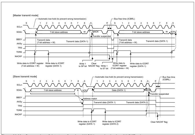
Figure 26.39 Suspension of data transfer when NACK is received, when NACKE = 1
