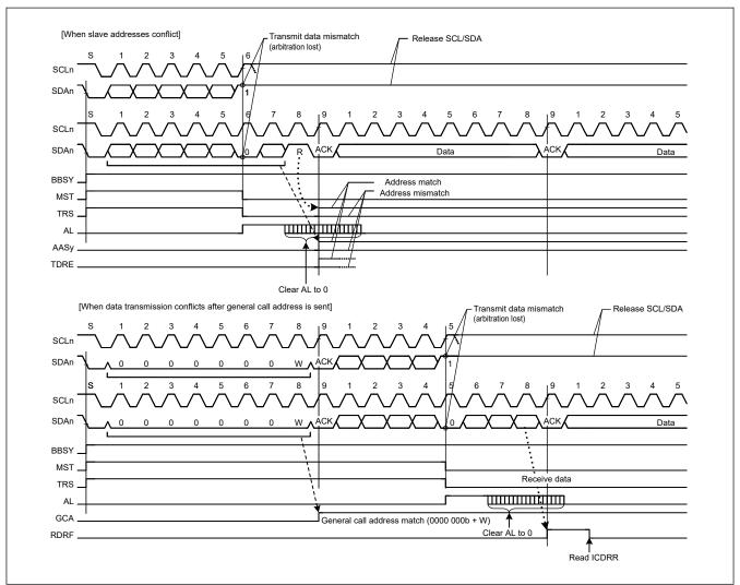
Figure 26.41 Examples of master arbitration-lost detection when MALE = 1
