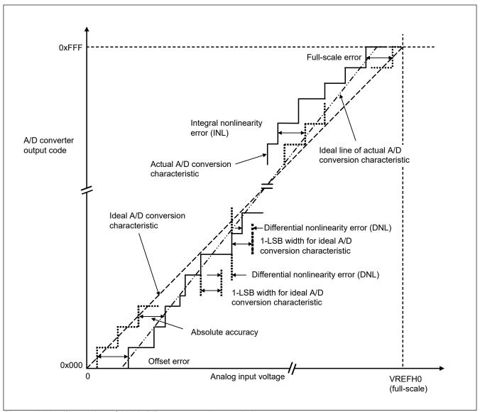
Figure 39.39 Illustration of 12-bit A/D converter characteristic terms
