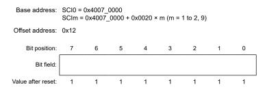
MDDR corrects the bit rate adjusted by the BRR register.
