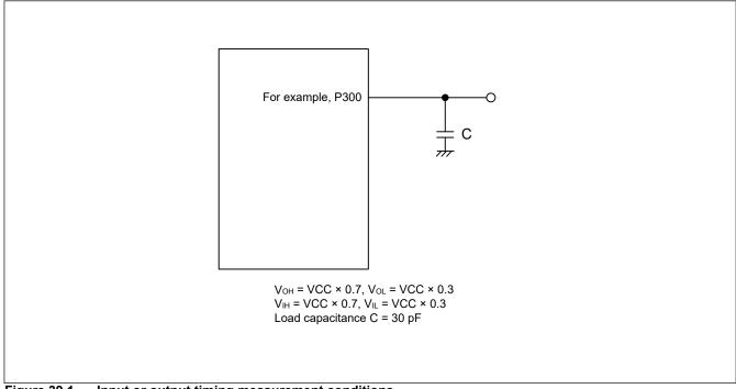
Figure 39.1 Input or output timing measurement conditions
