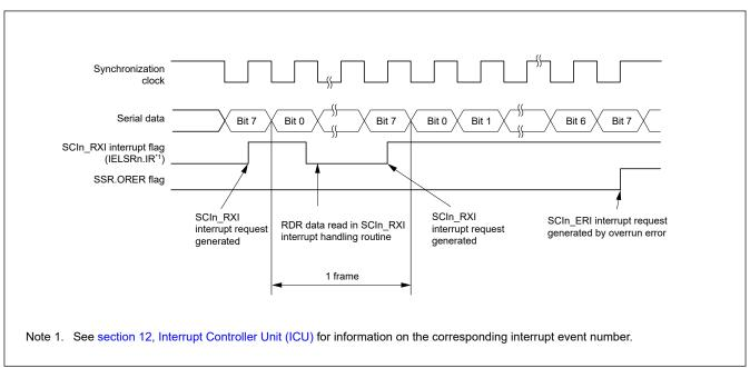
Figure 25.41 Example operation for serial reception in clock synchronous mode (1) when the RTS function is not used
