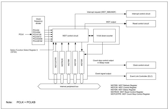
Figure 23.1 WDT block diagram
