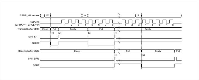
Figure 27.27 Operation example of the SPIi\_SPTI and SPIi\_SPRI interrupts when CPHA = 1 and CPOL = 0 in
