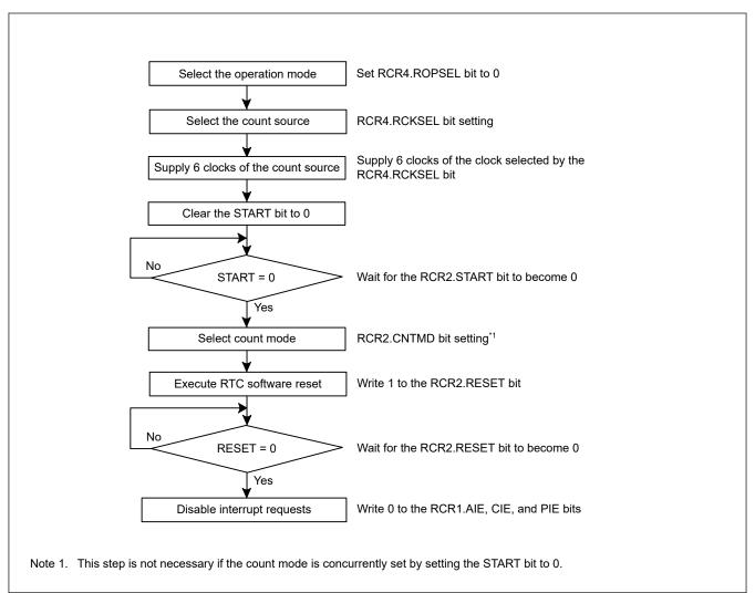
Figure 22.12 Initialization procedure
