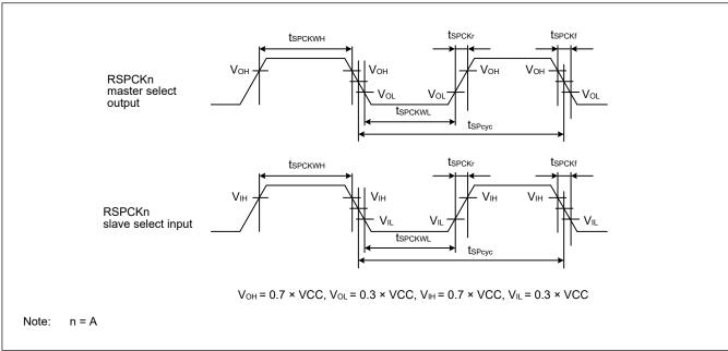
Figure 39.28 SPI clock timing
