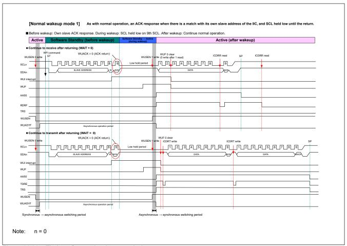
Figure 26.32 Timing of normal wakeup mode 1
