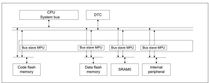
Figure 14.9 Bus slave MPU block diagram
