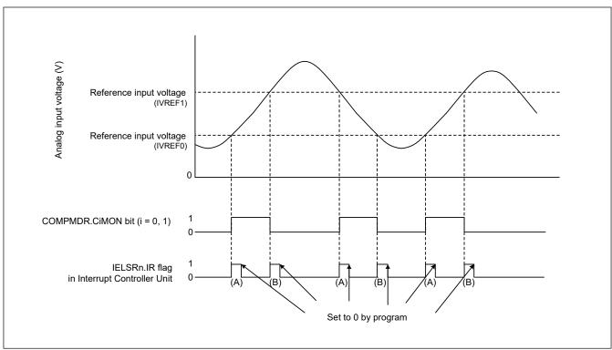
Figure 31.4 Operating example of ACMPLPi (i = 0, 1) when window function is enabled
