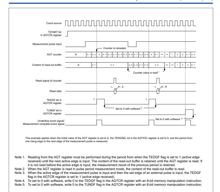
Figure 21.11 Operation example in pulse period measurement mode
