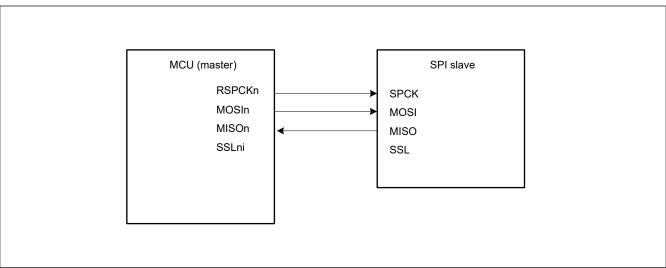
Figure 27.11 Clock synchronous master/slave configuration example with the MCU as a master
