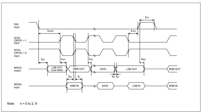
Figure 39.26 SCI simple SPI mode timing (slave, CKPH = 0)
