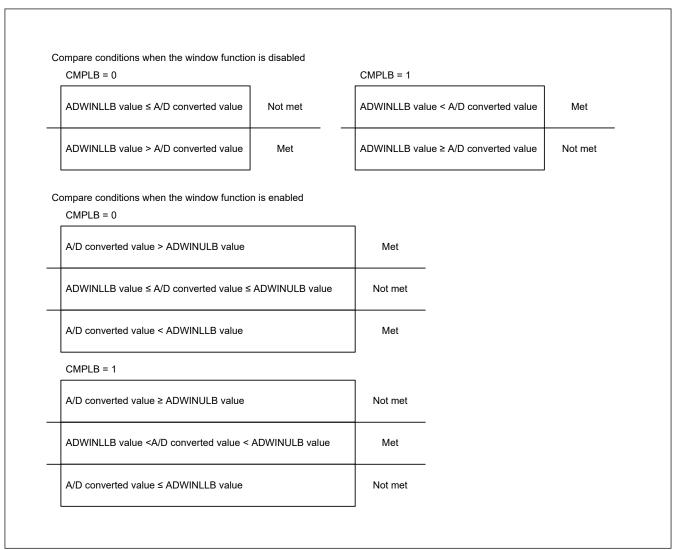
Figure 29.6 Explanation of compare conditions for compare function Window B
