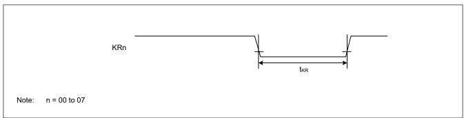
Figure 39.19 Key interrupt input timing
