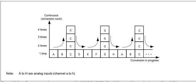
Figure 29.2 Scan conversion sequence with ADADC.ADC[2:0] = 011b, set 1 for analog inputs C and G by ADADS0/1
