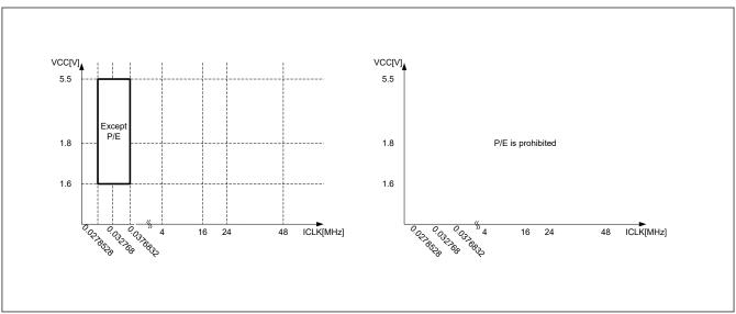
Figure 10.5 Operating voltages and frequencies in Subosc-speed mode
