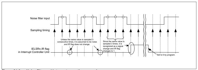
Figure 31.6 Noise filter and interrupt operation example
