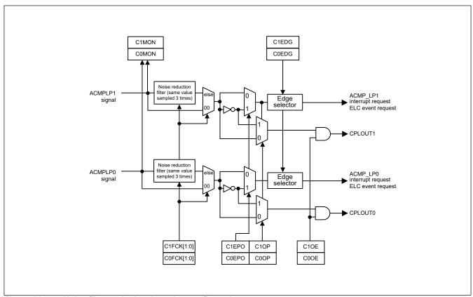
Figure 31.5 Noise filter and edge detection configuration
