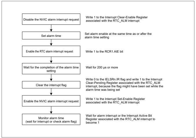
Figure 22.7 Using the alarm function
