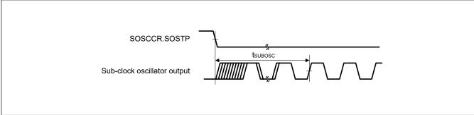
Figure 39.6 Sub-clock oscillation start timing
