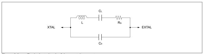
Figure 8.6 Equivalent circuit of the crystal resonator
