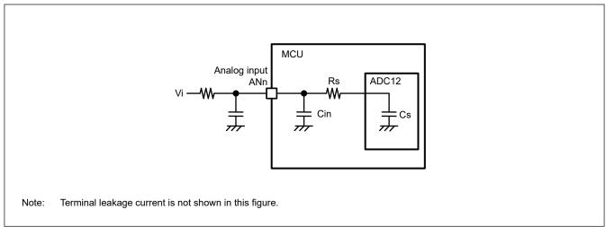
Figure 39.38 Equivalent circuit for analog input
