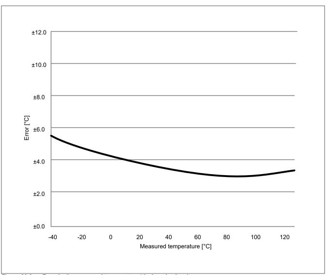
Figure 30.2 Error in the measured temperature (designed values)
