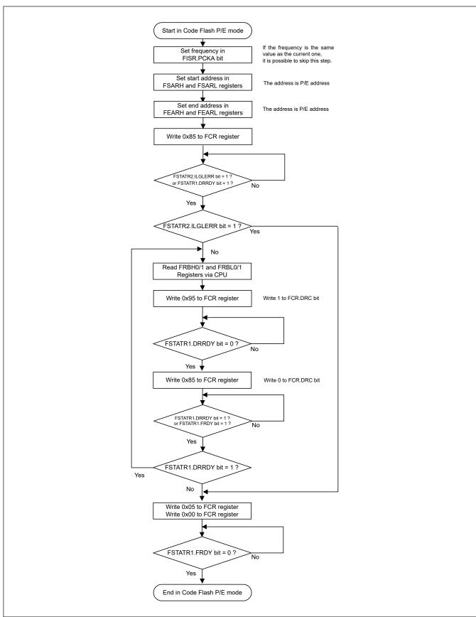
Figure 35.30 Simple flowchart for the consecutive read procedure
