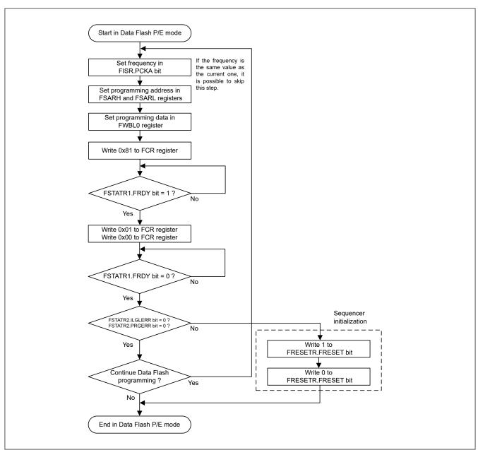
Figure 35.20 Flowchart for programming of the data flash
