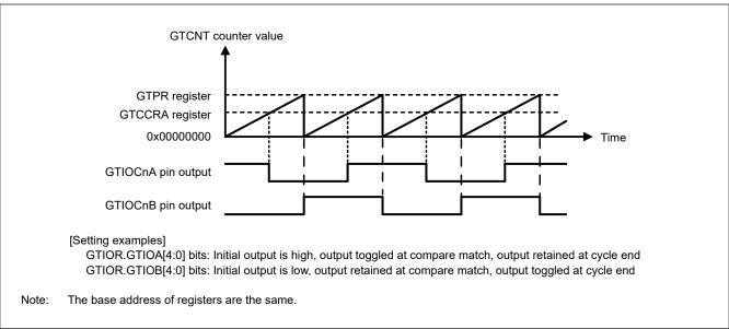
Figure 20.9 Example of toggled output operation (2)
