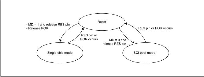
Figure 3.1 Mode-setting pin level and operating mode
