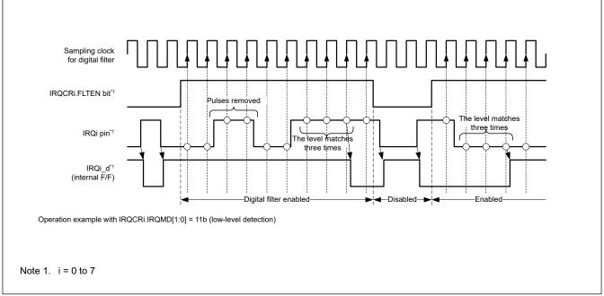
Figure 12.3 Digital filter operation example
