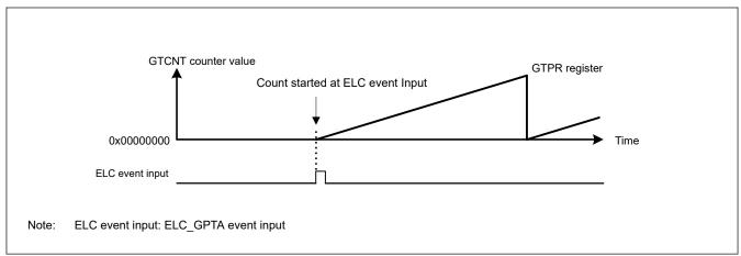
Figure 20.30 Example of count start operation by a hardware source started at the input of the signal from the ELC\_GPTA event
