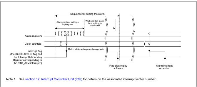
Figure 22.9 Timing for the alarm interrupt (RTC\_ALM)
