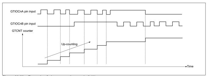
Figure 20.53 Example of phase counting mode 5 (A)
