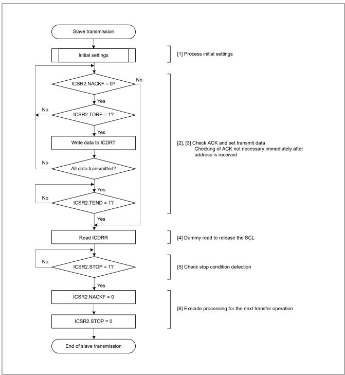
Figure 26.15 Example slave transmission flow
