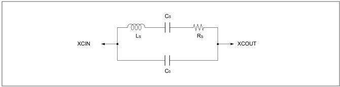
Figure 8.9 Equivalent circuit for the 32.768-kHz crystal resonator
