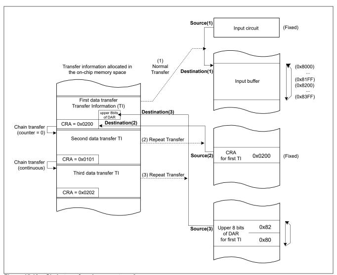
Figure 15.13 Chain transfer when counter = 0
