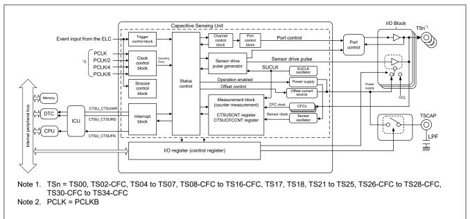
Figure 32.3 CTSU2 block diagram
