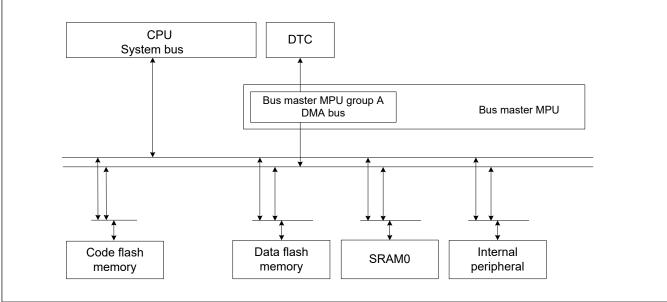
Figure 14.3 MPU bus master block diagram
