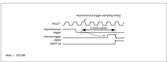
Figure 29.30 Asynchronous trigger input timing
