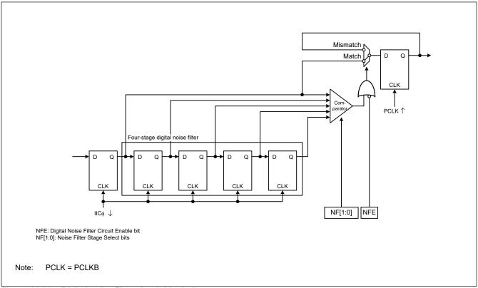
Figure 26.23 Digital noise filter circuit block diagram
