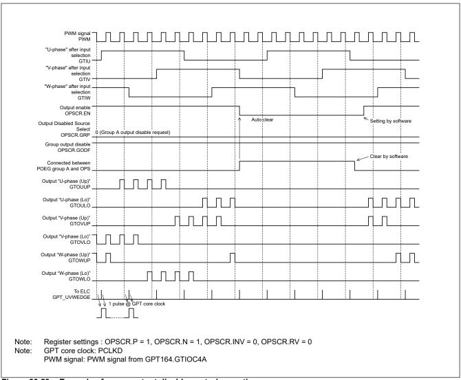
Figure 20.58 Example of group output disable control operation
