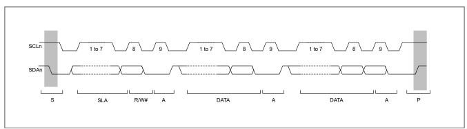
Figure 26.4 I<sup>2</sup>C bus timing when the SLA setting = 7 bits
