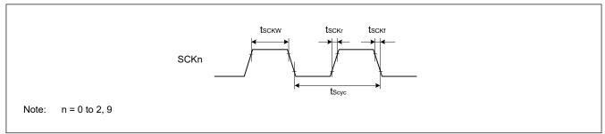
Figure 39.20 SCK clock input timing
