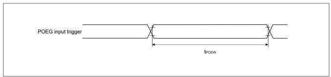
Figure 39.15 POEG input trigger timing
