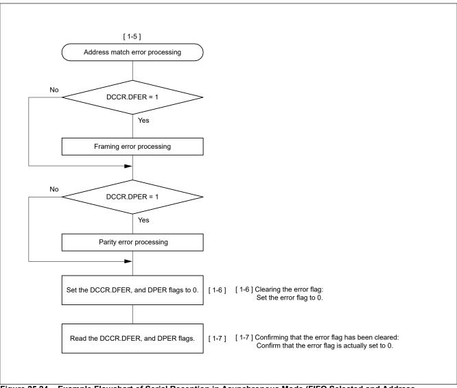
Figure 25.24 Example Flowchart of Serial Reception in Asynchronous Mode (FIFO Selected and Address Matching Enabled) (2)
