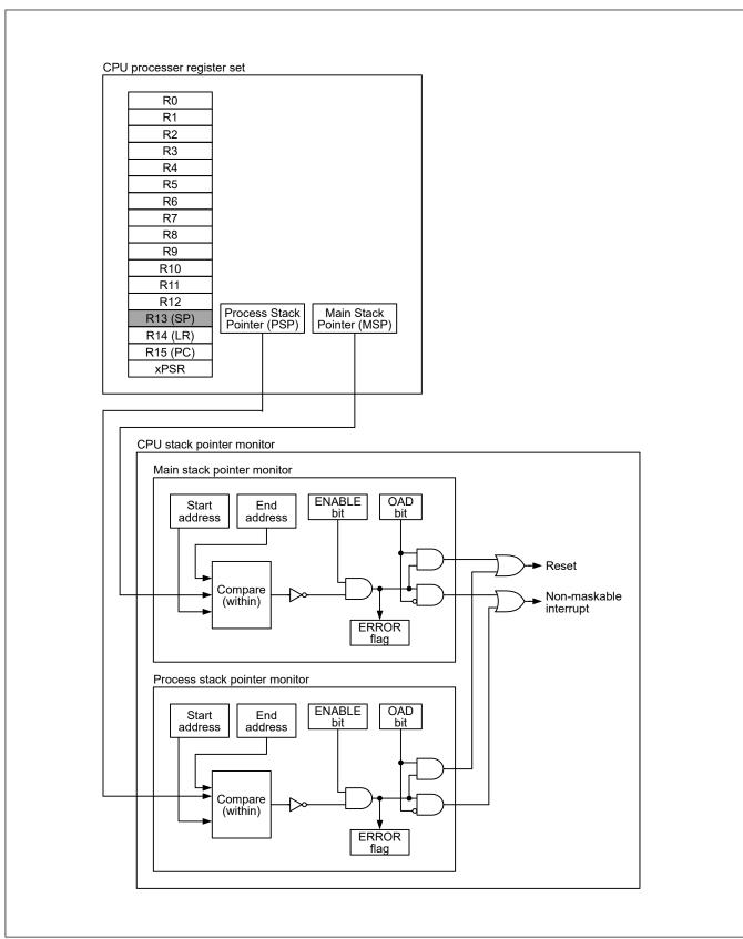
Figure 14.1 CPU stack pointer monitor block diagram
