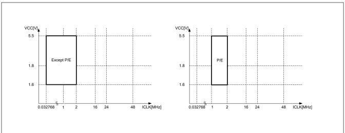
Figure 10.4 Operating voltages and frequencies in Low-speed mode
