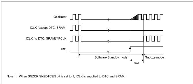
Figure 39.11 Recovery timing from Software Standby mode to Snooze mode
