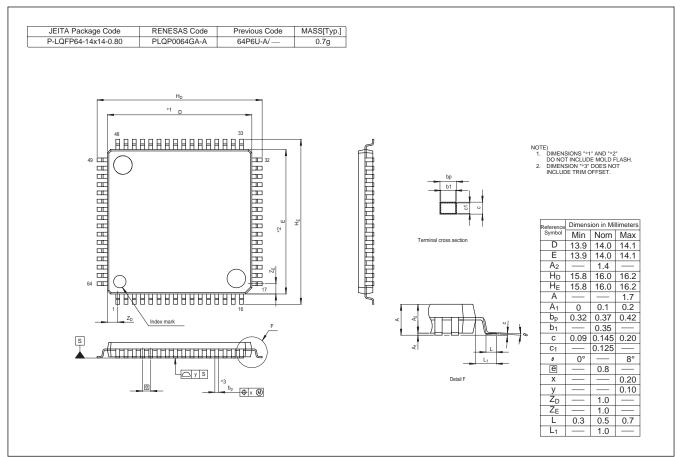
Figure 2.3 LQFP 64-pin 0.8mm pitch
