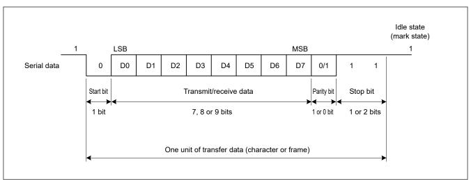
Figure 25.2 Data format in asynchronous serial communications with 8-bit data, parity bit, and 2 stop bits
