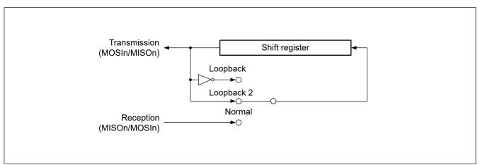
Figure 27.42 Configuration of shift register I/O paths in loopback mode for master mode
