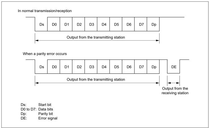
Figure 25.48 Data formats in smart card interface mode
