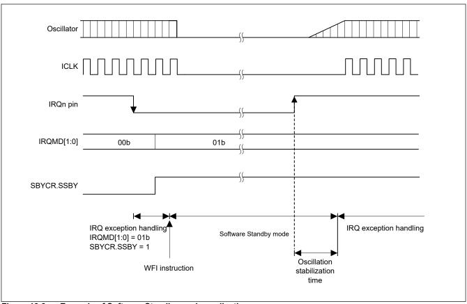
Figure 10.6 Example of Software Standby mode application
