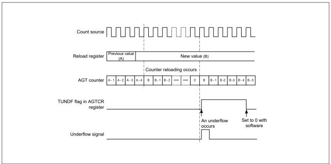
Figure 21.6 Operation example in timer mode
