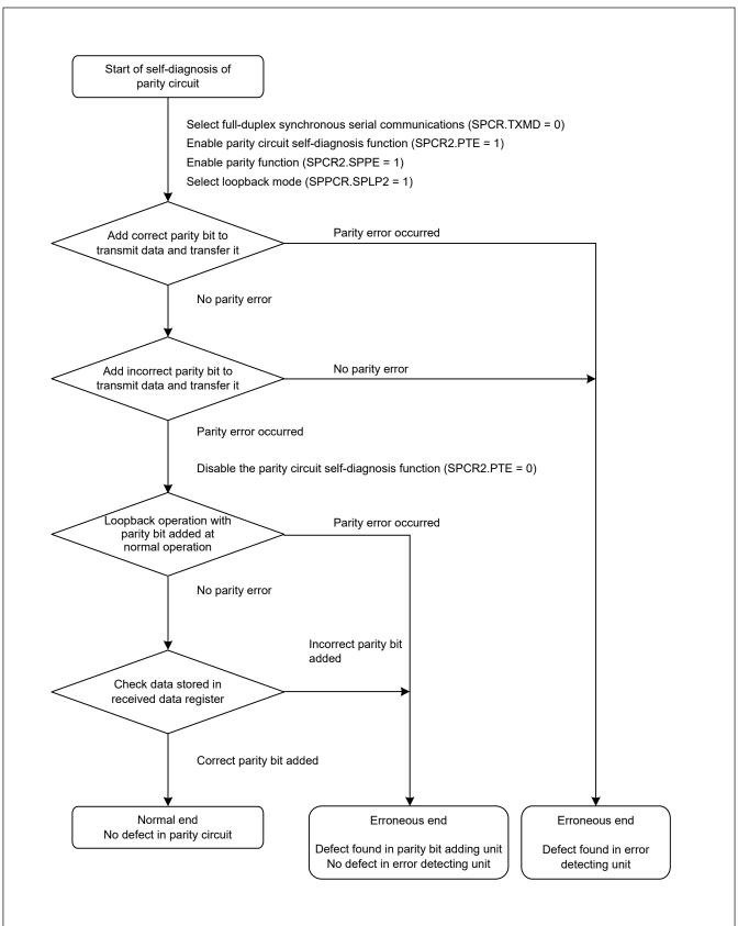
Figure 27.43 Self-diagnosis flow for parity circuit
