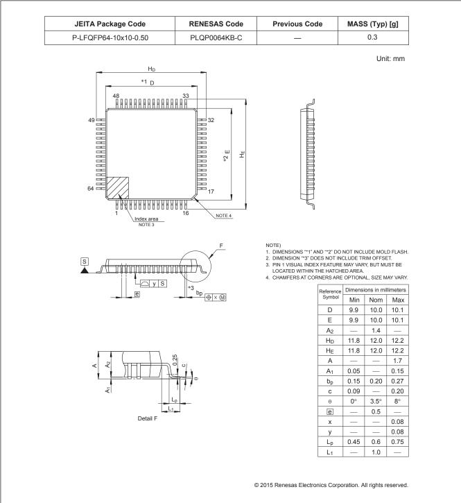
Figure 2.1 LQFP 64-pin 0.5mm pitch (1)
