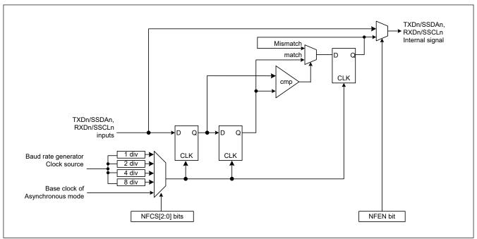
Figure 25.71 Digital noise filter circuit block diagram
