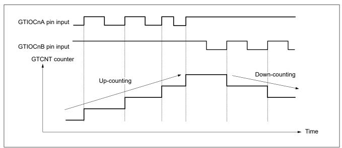
Figure 20.50 Example of phase counting mode 3 (B)
