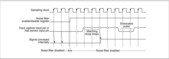
Figure 20.59 Timing of noise filtering
