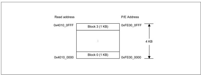
Figure 35.3 Mapping of the data flash memory
