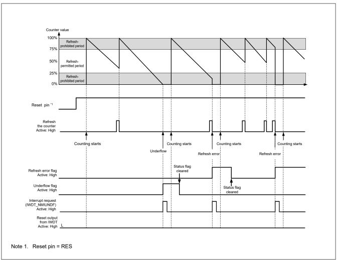
Figure 24.3 Operation example in auto start mode
