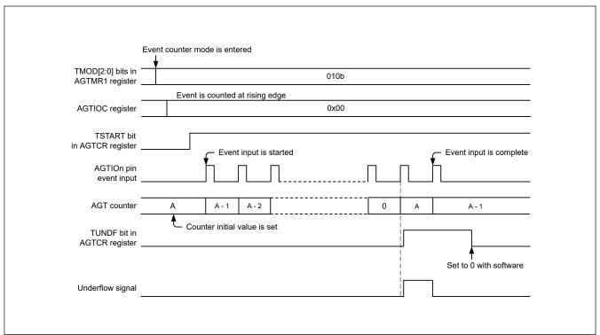
Figure 21.8 Operation example 1 in event counter mode
