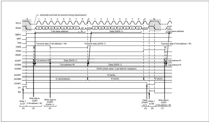
Figure 26.46 Restart condition issue timing after master transmission.
