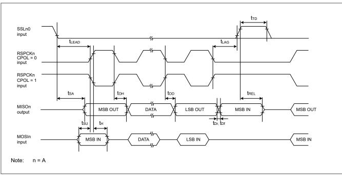
Figure 39.33 SPI timing (slave, CPHA = 0)
