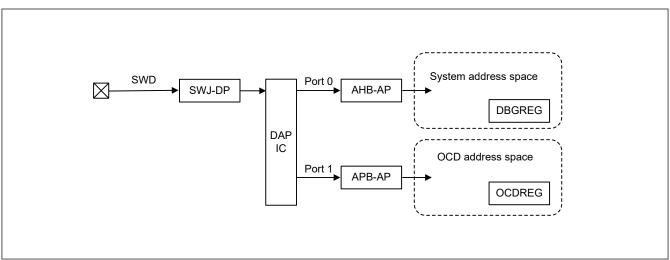
Figure 2.2 SWD authentication block diagram
