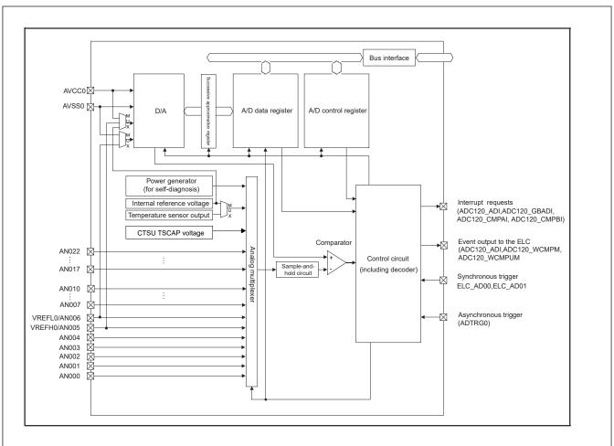
Figure 29.1 ADC12 block diagram
