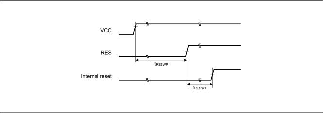
Figure 39.7 Reset input timing at power-on
