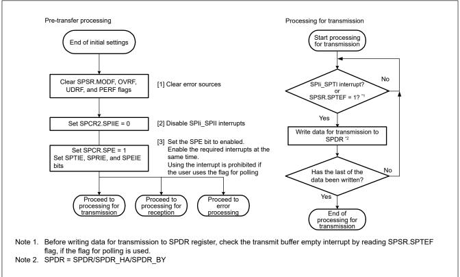
Figure 27.37 Transmission flow in slave mode
