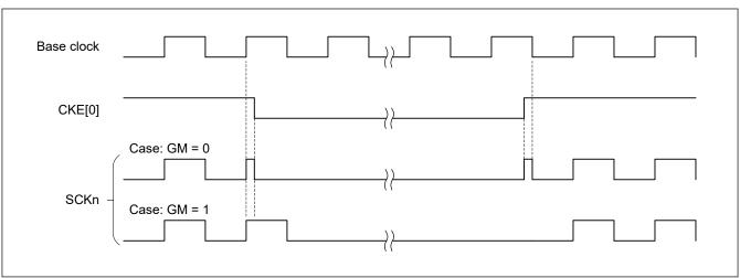
Figure 25.57 Clock Output timing
