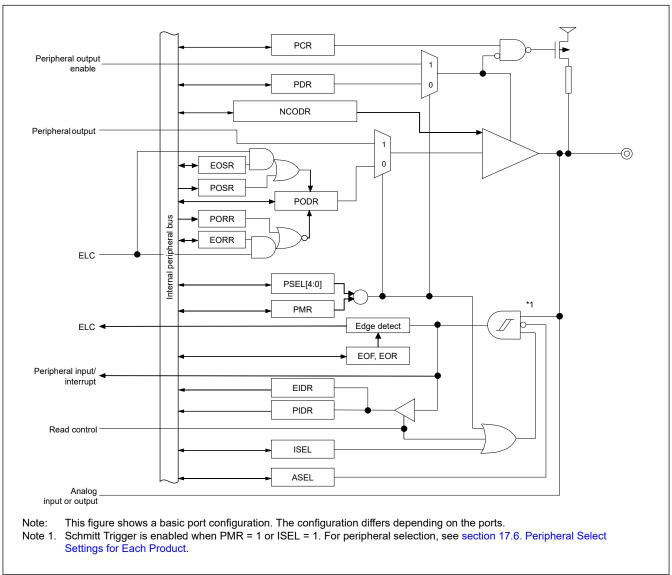
Figure 17.1 Connection diagram for I/O port registers
