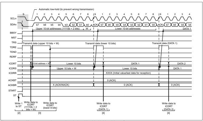
Figure 26.8 Master transmit operation timing (2) with 10-bit address format
