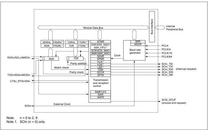
Figure 25.1 SCI block diagram
