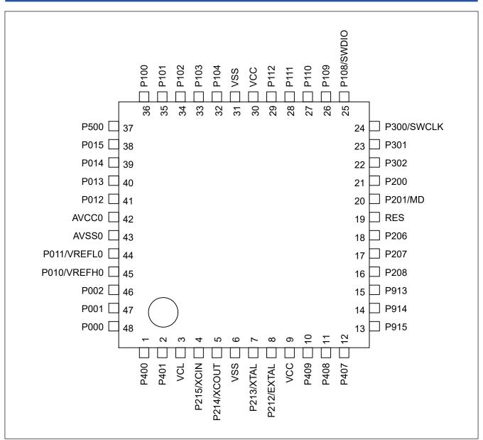
Figure 1.5 Pin assignment for LQFP/QFN 48-pin (top view)
