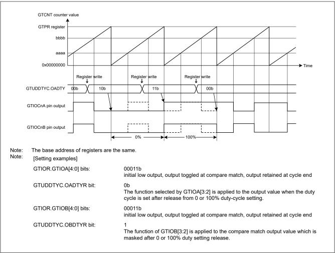
Figure 20.29 Example of output duty 0% and 100% function
