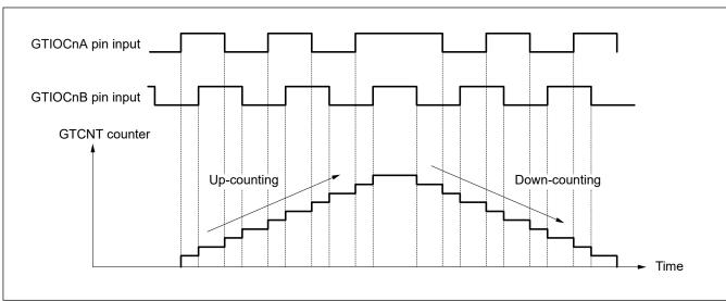
Figure 20.45 Example of phase counting mode 1
