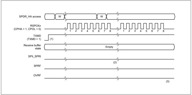
Figure 27.25 Operation example when SPCR.TXMD = 1
