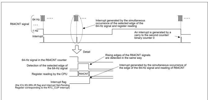
Figure 22.10 Timing for the carry interrupt (RTC CUP)
