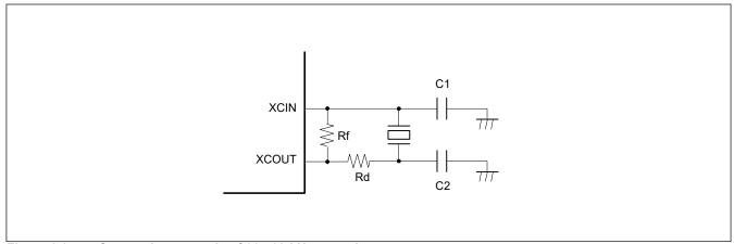
Figure 8.8 Connection example of 32.768-kHz crystal resonator
