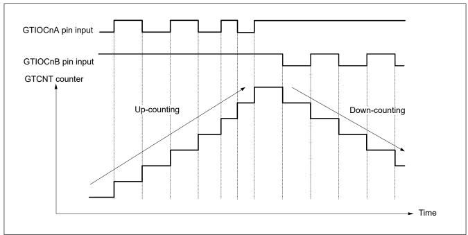
Figure 20.51 Example of phase counting mode 3 (C)
