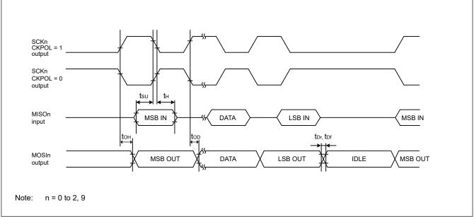
Figure 39.24 SCI simple SPI mode timing (master, CKPH = 0)
