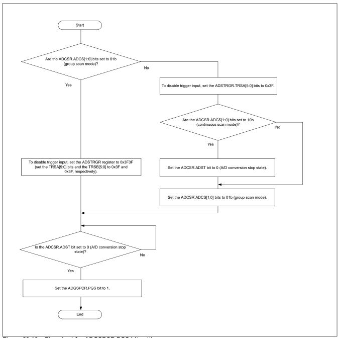
Figure 29.16 Flowchart for ADGSPCR.PGS bit setting
