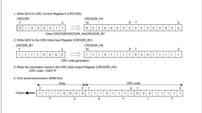
Figure 28.3 MSB-first data transmission
