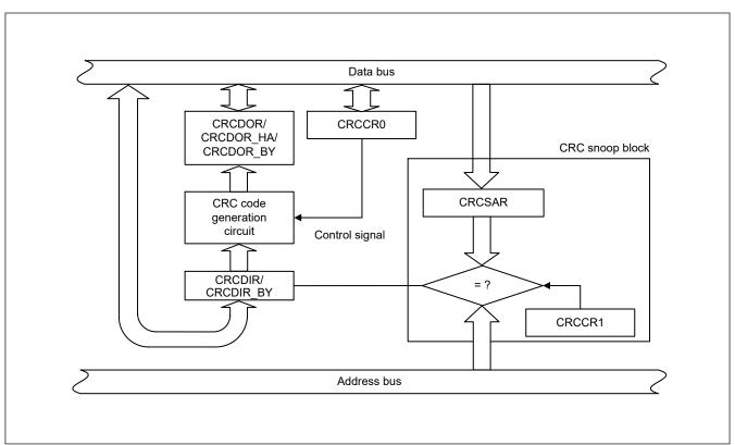
Figure 28.1 CRC calculator block diagram
