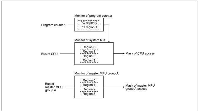
Figure 14.10 Security MPU block diagram
