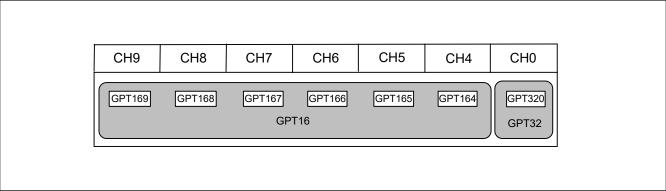
Figure 20.2 Association between GPT channels and module names
