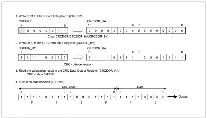
Figure 28.2 LSB-first data transmission
