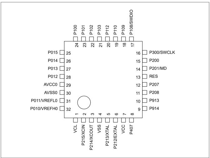
Figure 1.7 Pin assignment for LQFP/QFN 32-pin (top view)
