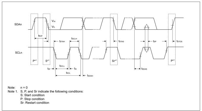
Figure 39.35 I<sup>2</sup>C bus interface input/output timing
