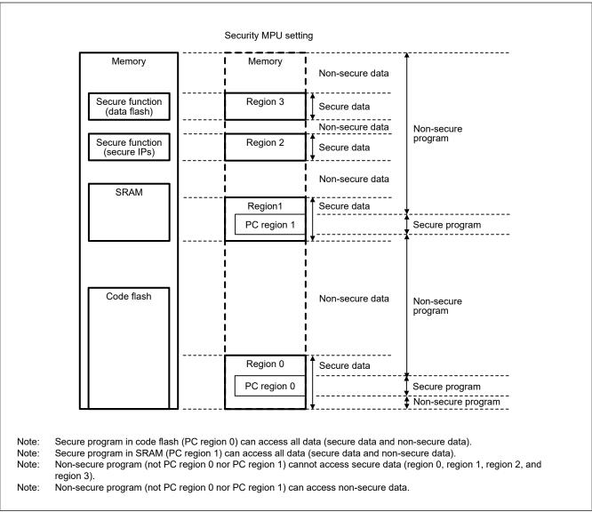
Figure 14.11 Use case of security MPU
