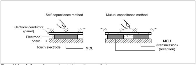
Figure 32.2 Self-capacitance and mutual capacitance methods
