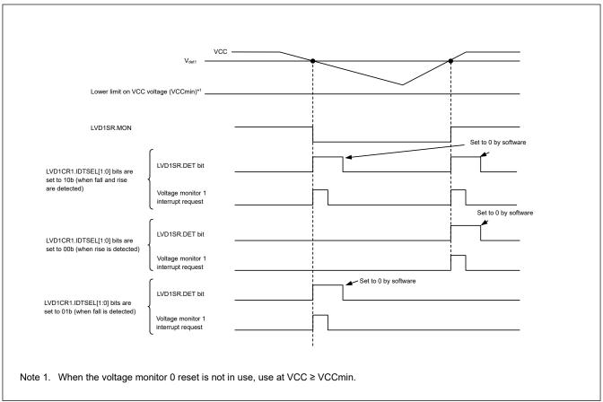
Figure 7.5 Example of voltage monitor 1 interrupt operation
