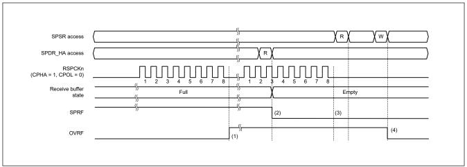
Figure 27.28 Operation example of the OVRF and SPRF flags
