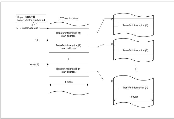
Figure 15.2 DTC vector table and transfer information
