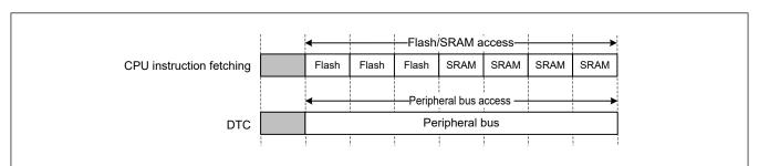
Figure 13.2 Example of parallel operations
