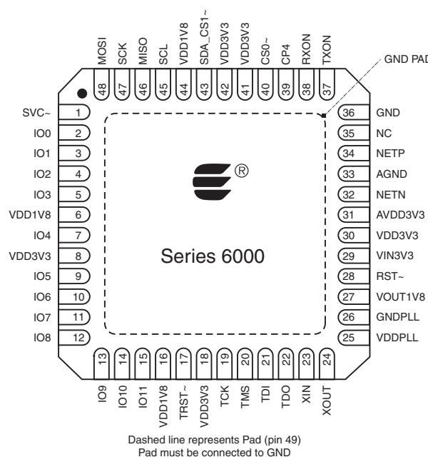
Figure 3. 6K IC Pin Configuration
