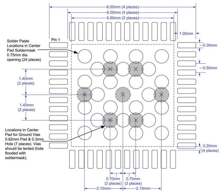
Figure 4. Recommended 6K Pad Layout
