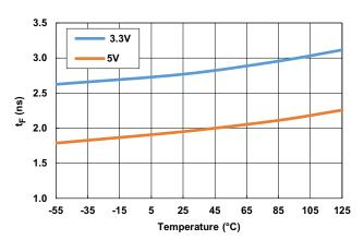
Figure 17. Output Fall Time vs Temperature vs  $V_{DD}$ Voltage
