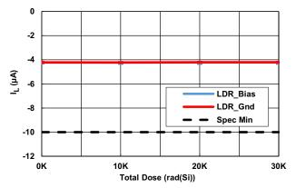
Figure 32. 5.5V Logic Input Current - Low vs TID
