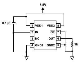
Figure 33. 5.5V Logic Input Current - High vs TID
