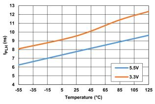
Figure 15. Propagation Delay (Low-to-High) vs Temperature vs  $V_{DD}$  Voltage
