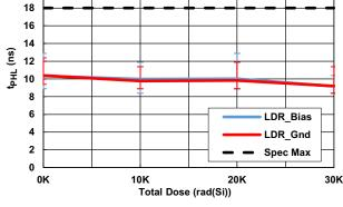
Figure 29. 5.5V Propagation Delay (Low-to-High) vs TID
