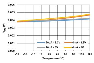
Figure 20. Logic Low Output Voltage vs Temperature
