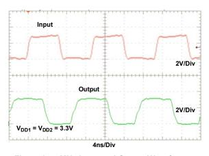
Figure 8. 75MHz Input and Output Waveforms
