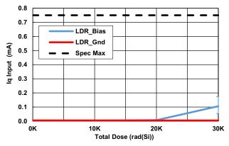
Figure 27. 5.5V Output Quiescent Supply Current vs TID
