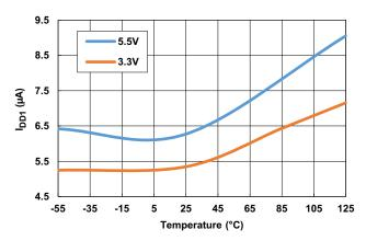
Figure 12. Input Quiescent Supply Current vs Temperature vs V<sub>DD1</sub> Voltage
