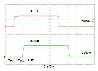
Figure 6. 10MHz Input and Output Waveforms
