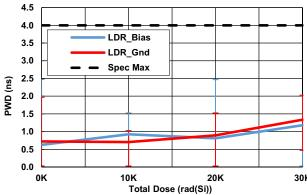
Figure 31. 5.5V Pulse-Width Distortion vs TID
