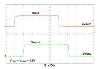
Figure 2. 10MHz Input and Output Waveforms
