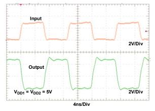
Figure 10. 75MHz Input and Output Waveforms
