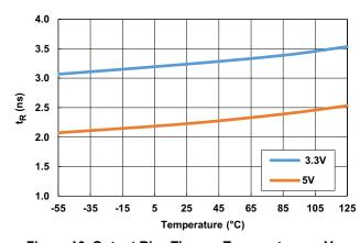
Figure 16. Output Rise Time vs Temperature vs  $V_{DD}$  Voltage
