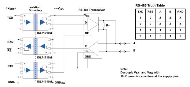
Figure 3. RS-485 Multi-Chip Isolated Transceiver Application Schematic
