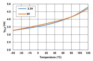
Figure 23. Propagation Delay Enable to Output (Low-to-High Impedance) vs Temperature
