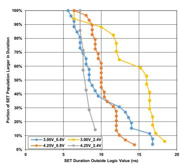
Figure 35. Plot of Cumulative SET Population Portion that is Above an Indicated SET Duration at LET 43MeV•cm<sup>2</sup>/mg
