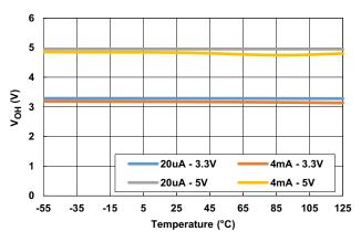
Figure 21. Logic High Output Voltage vs Temperature
