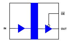
Figure 4. ISL71710M Block Diagram
