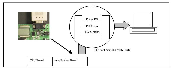
A RS232 driver, which is built on the application board, is required to interface the MCU to the PC.
