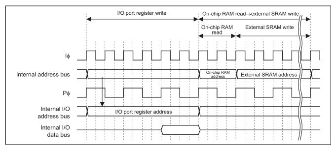
Figure 2 Example of Timing of Operations with the Write Data Buffer Function for Peripheral Modules not in Use (PWDBE = 0)
