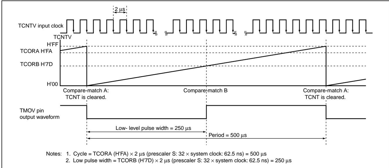
**Figure 2.2 Setting of the Overall and Low-Level Periods for the TMOV-Pin Output Waveform**
