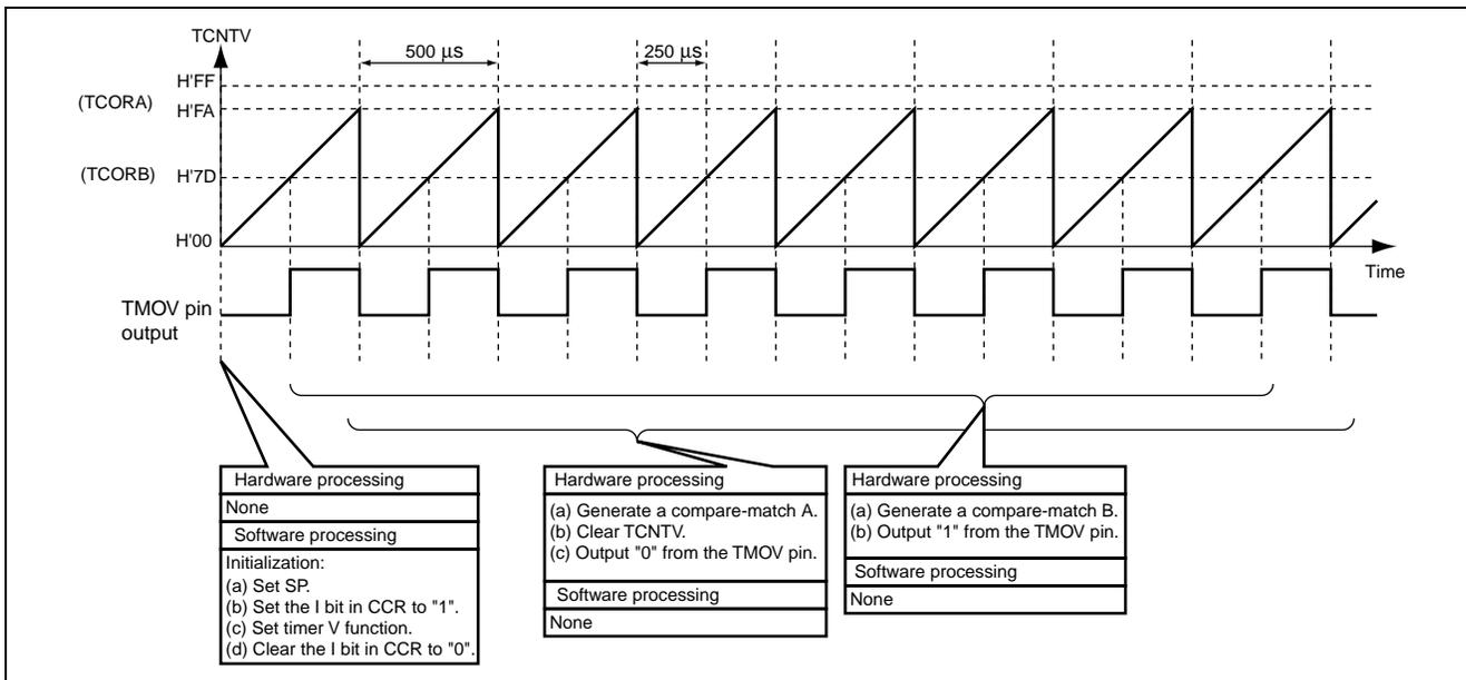
Figure 3.1 Operational Principle for TMOV Pin Output
