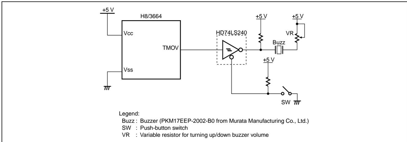
**Figure 1.1 Hardware Configuration**
