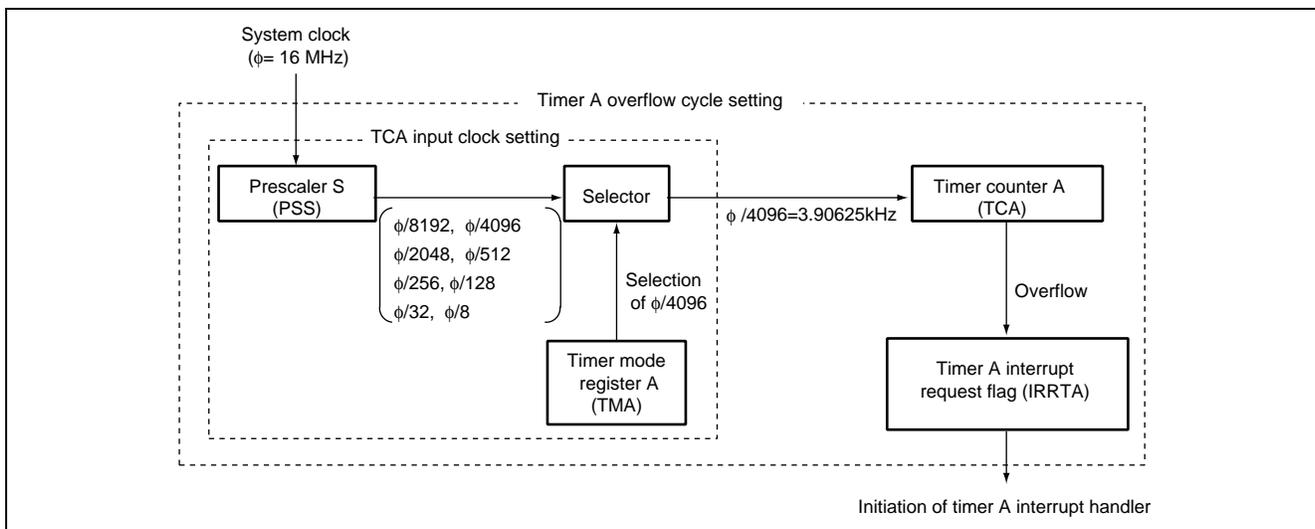
**Figure 2.1 Timer A's Interval Timing Function**
