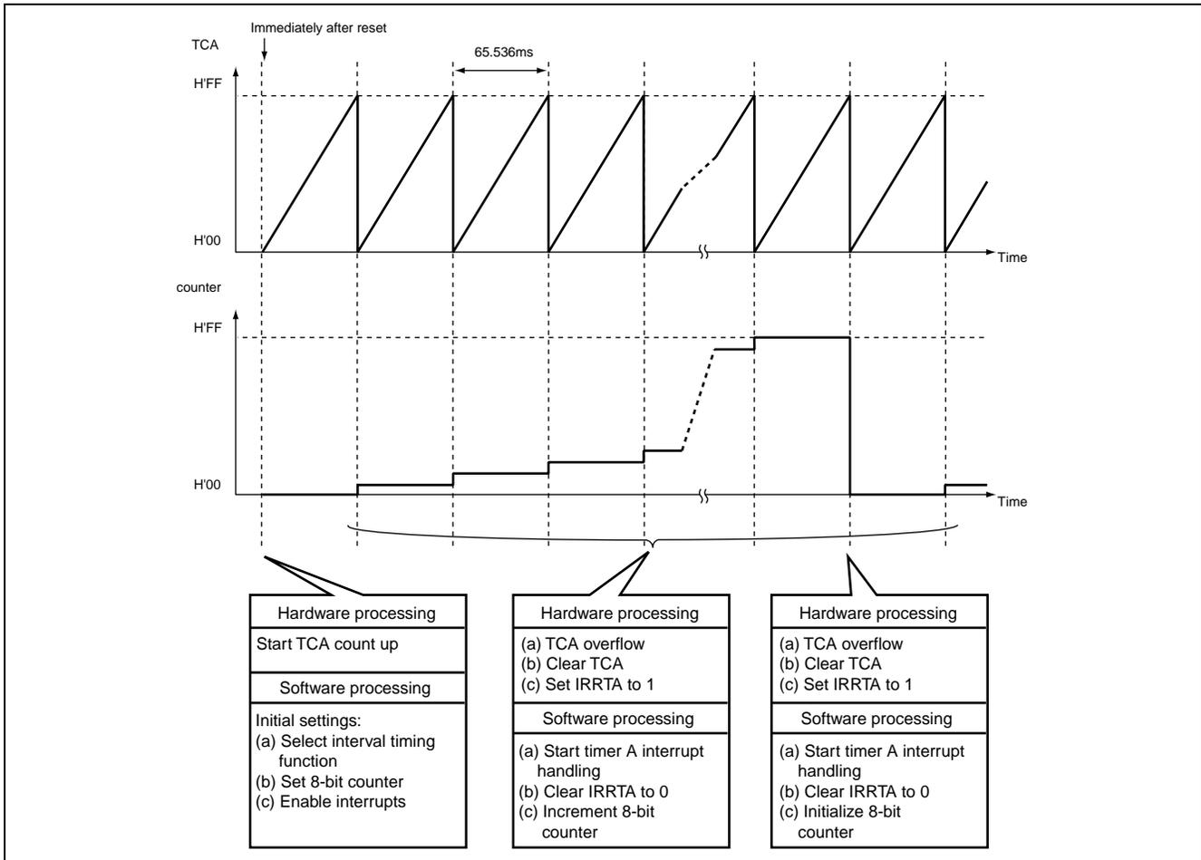
Figure 3.1 Operation Principle: Using Interval Timing Function of Timer A to Increment 8-Bit Counter
