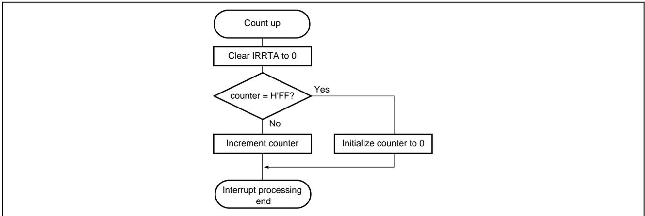
Figure 5.2 Flowchart for Timer A Interrupt Handling Routine
