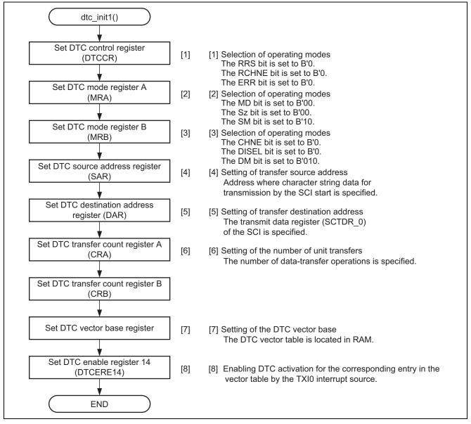
Figure 11 Flow 1 of DTC Initialization
