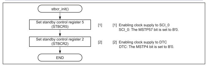
Figure 9 Flow of Setting for Release from Module-Standby Mode
