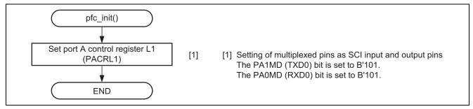
Figure 10 Flow for Setting up the Pin Function Controller
