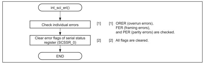
Figure 16 Flow for Handling Receive Error Interrupts
