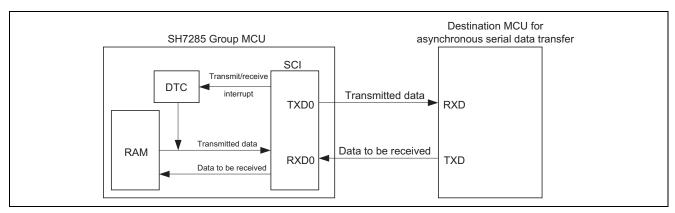
Figure 1 Example of Connection for Using the DTC in Transmission and Reception of Serial Data in Asynchronous Mode
