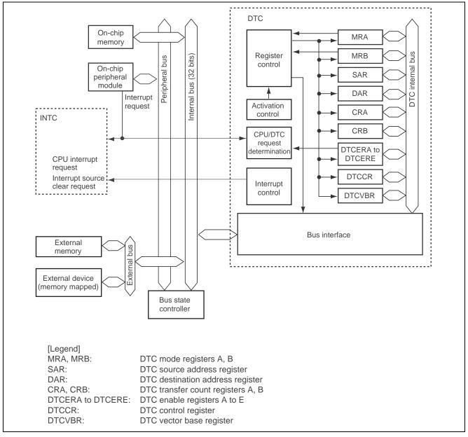
Figure 3 Block Diagram of the DTC
