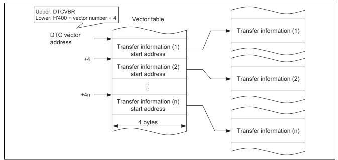
Figure 5 Correspondence between DTC Vector Addresses and Transfer Information
