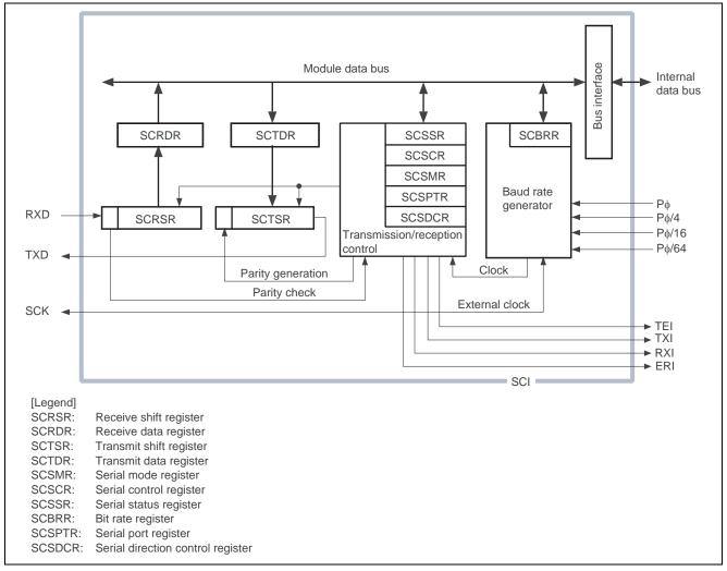
Figure 2 Block Diagram of the SCI
