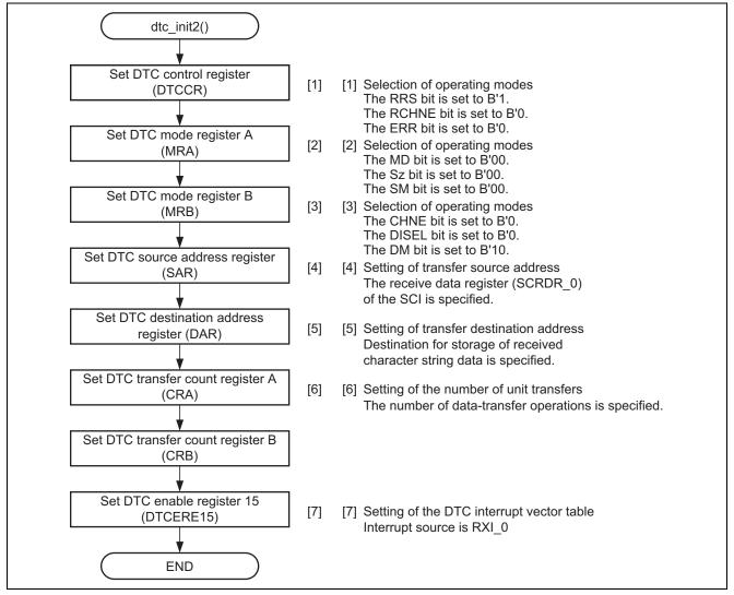
Figure 12 Flow 2 of DTC Initialization
