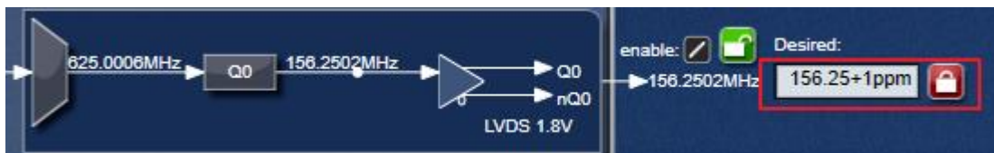
Figure 2. Output Frequency with PPM Offset
