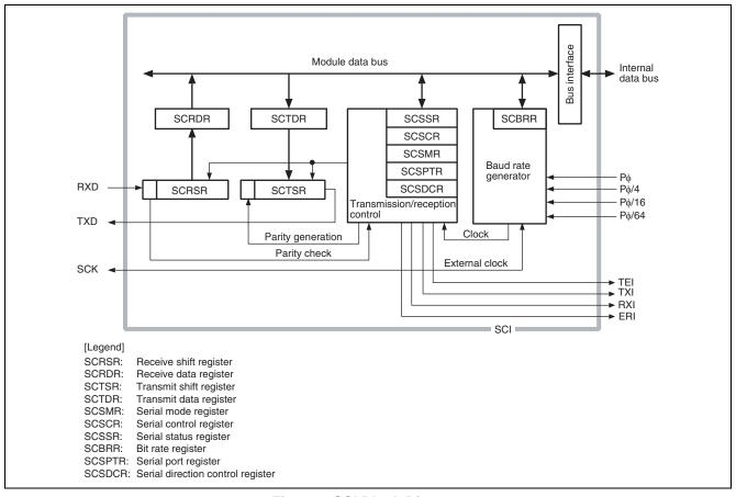
Figure 2 SCI Block Diagram
