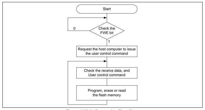
Figure 10 Main Processing Flow Chart
