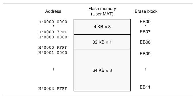
Figure 6 Dividing the Flash Memory Erase Block
