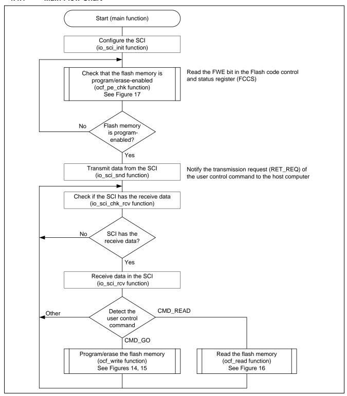
Figure 13 Main Processing Flow Chart
