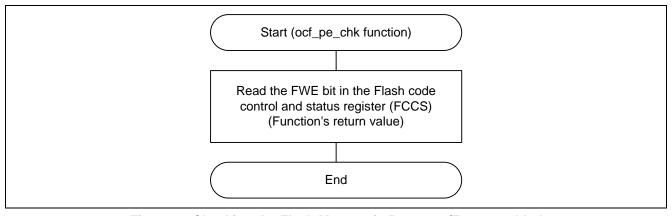
Figure 17 Checking the Flash Memory is Program-/Erase-enabled
