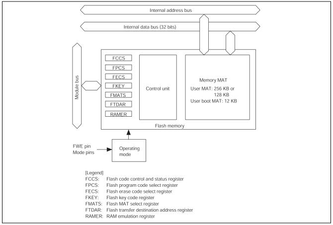
Figure 3 Flash Memory Block Diagram
