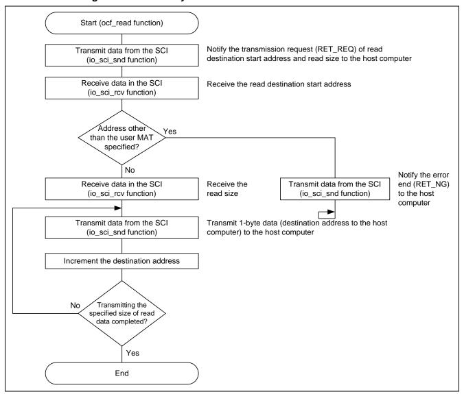
Figure 16 Reading the Flash Memory
