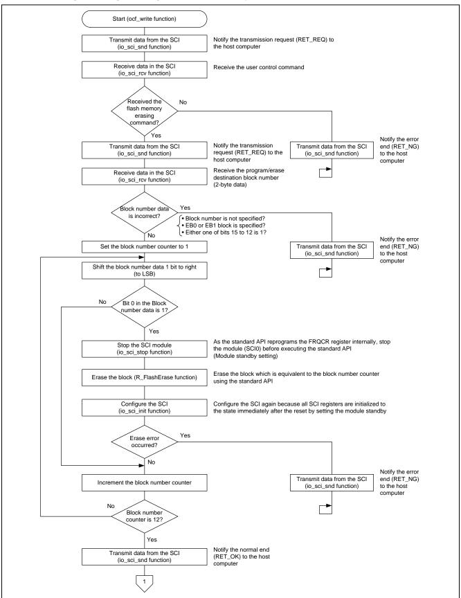
Figure 14 Programming/Erasing the Flash Memory (1/2)
