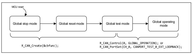
Figure 3-1 State transition diagram of the global mode
