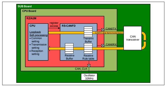
Figure 3-9 System configuration
