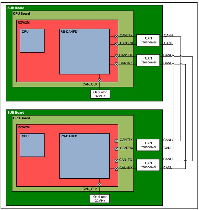
Figure 2-1 Hardware configuration
