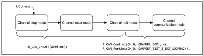
Figure 3-2 State transition diagram of the channel mode
