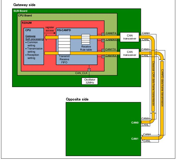
Figure 3-7 System configuration
