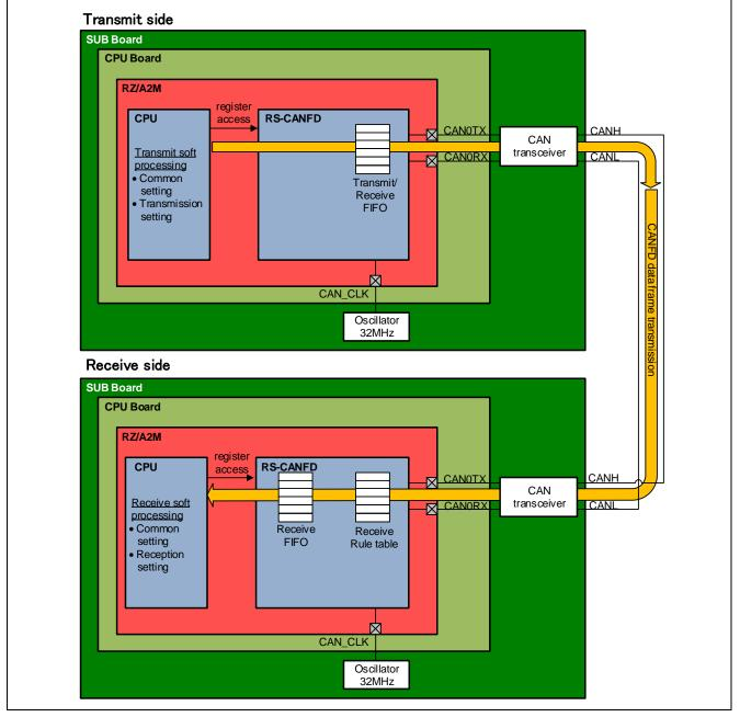
Figure 3-4 System configuration
