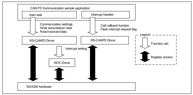
Figure 2-3 Sample program system block diagram
