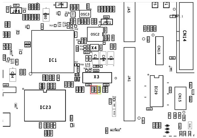
Figure 3-2 Location of modified resistors
