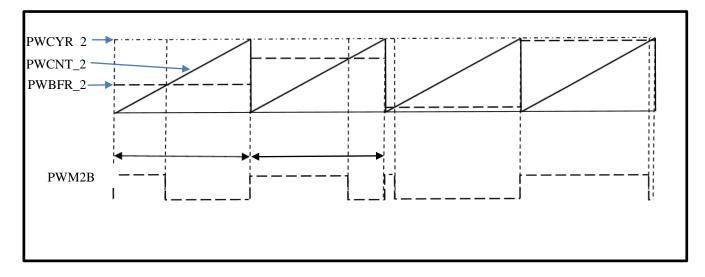
Figure 4-1 Description of PWM Operation
