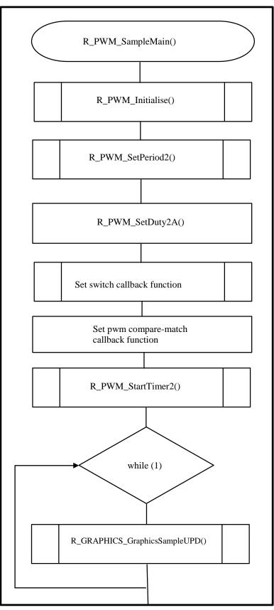
Figure 4-3 Backlight Background Program Flow
