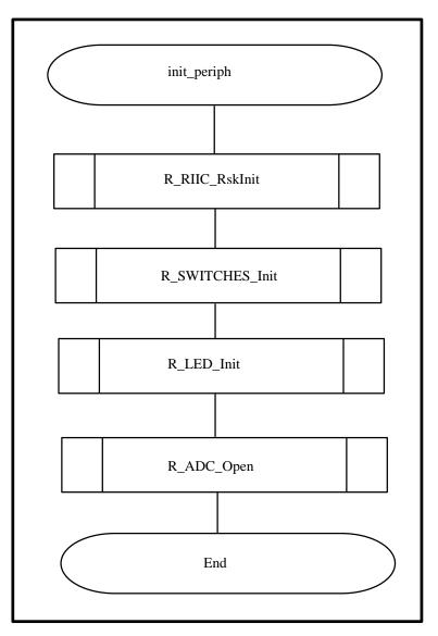
**Figure 4-2 Peripheral Initialisation Flow Chart**
