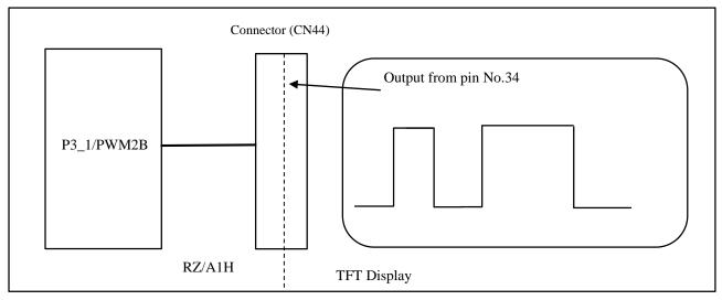
Figure 3-1 Connection of Backlight Control from MCU to Display
