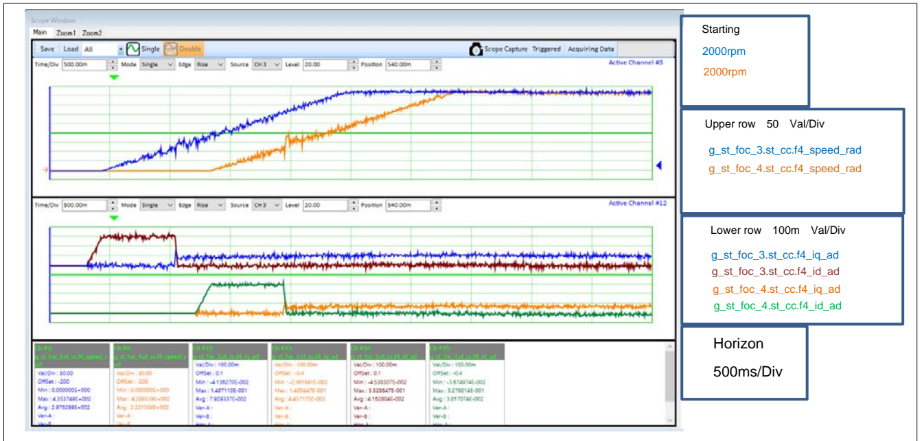
Figure 5-3 Driving Waveforms When Motors 3 and 4 are Starting up (3/3)
