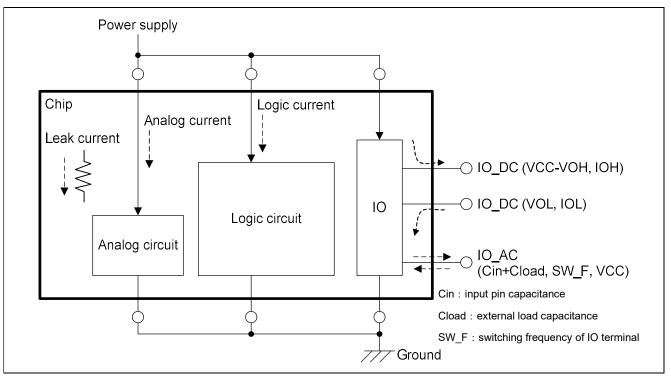
Figure 3.1 Current Path Configuration Diagram
