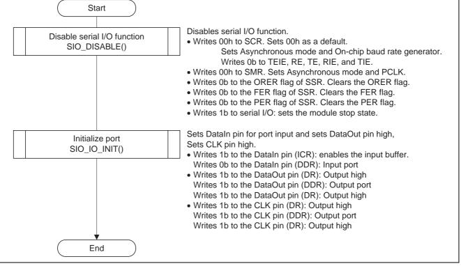
Figure 7 Serial I/O Disable Setup Processing Outline
