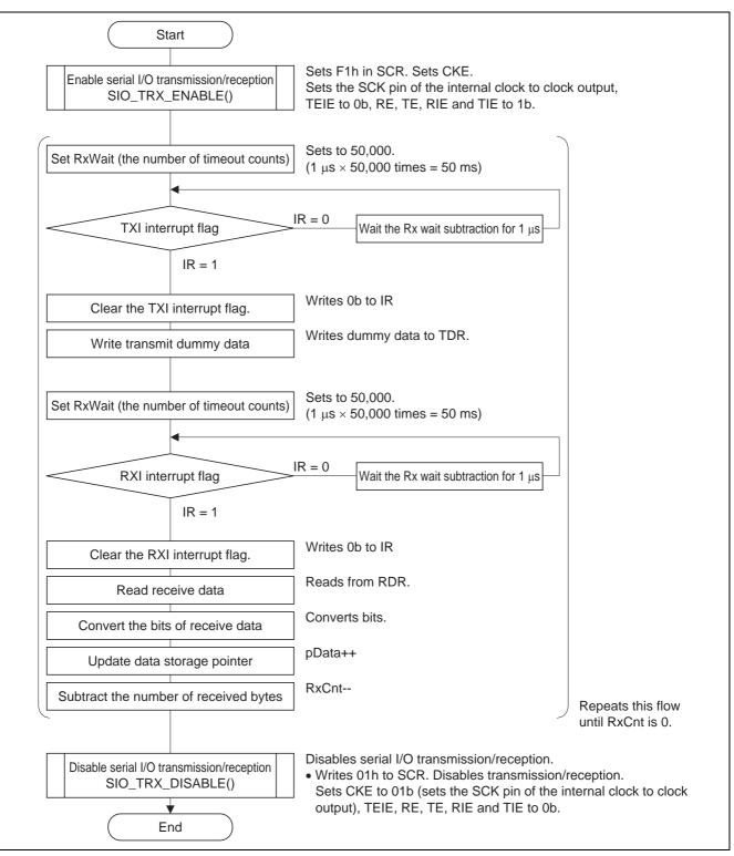
Figure 11 Serial I/O Data Reception Processing Outline
