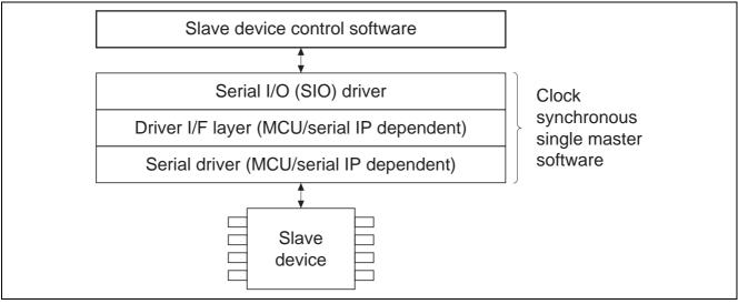
Figure 5 Software Configuration
