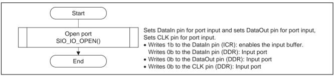
Figure 9 Serial I/O Open Setup Processing Outline
