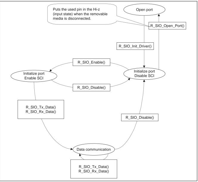
Figure 12 State Transition Diagram
