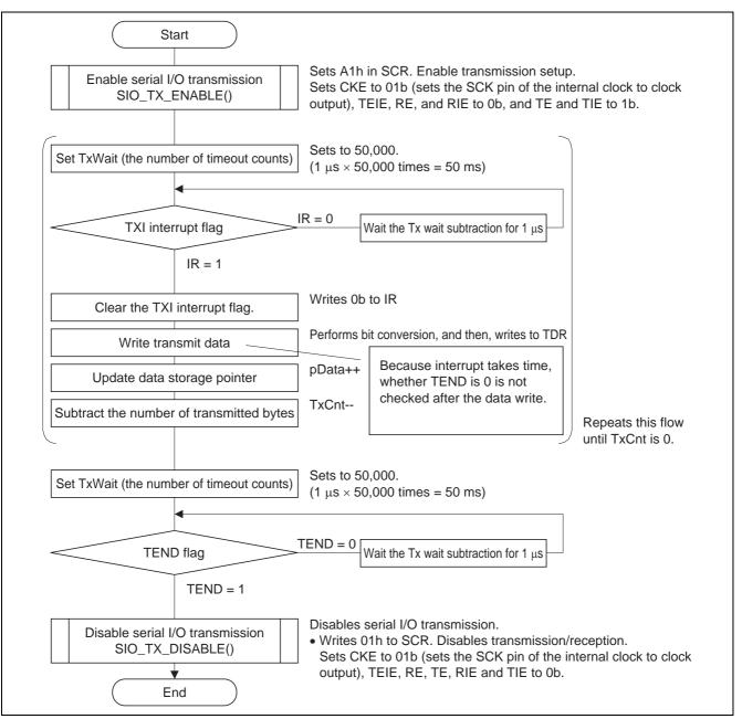
Figure 10 Serial I/O Data Transmission Processing Outline
