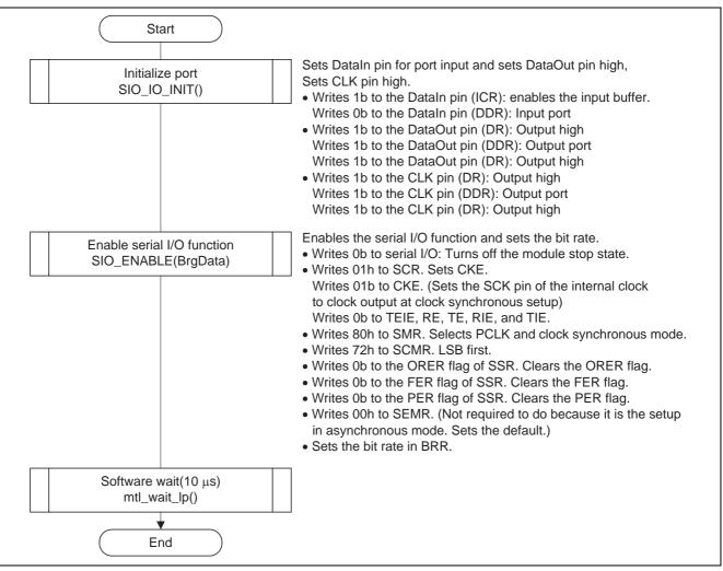
Figure 8 Serial I/O Enable Setup Processing Outline
