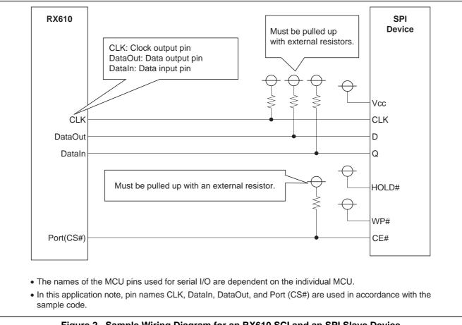
Figure 2 Sample Wiring Diagram for an RX610 SCI and an SPI Slave Device
