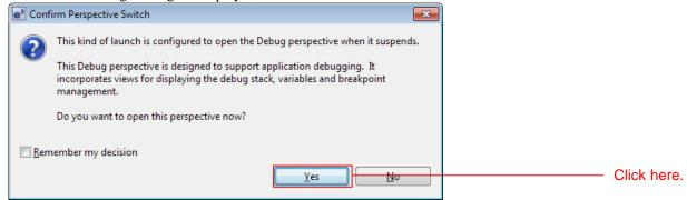
6. When the load module download completes, a **Debug** perspective opens.
