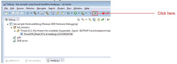
8. After the break at the start of the main function, click **Restart** on the tool bar again. The project will be run and the program will iterate toggling LED0 with a period of 0.5 seconds.
