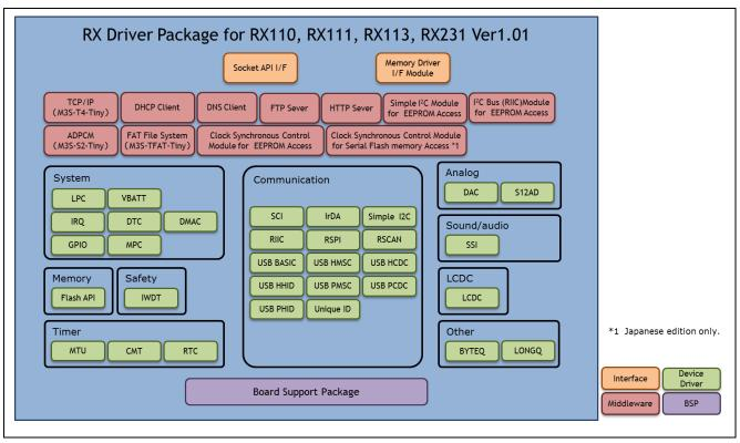
Figure 3-2 RX110, RX111, RX113, RX231 Group RX Driver Package FIT Module Structure
