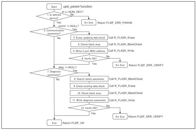
Figure 3.8 Parameter updating operation
