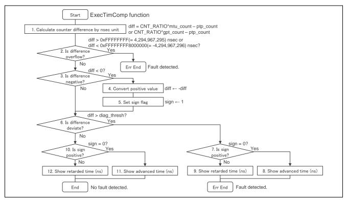
Figure 3.5 Multi-functional timer comparison's operation
