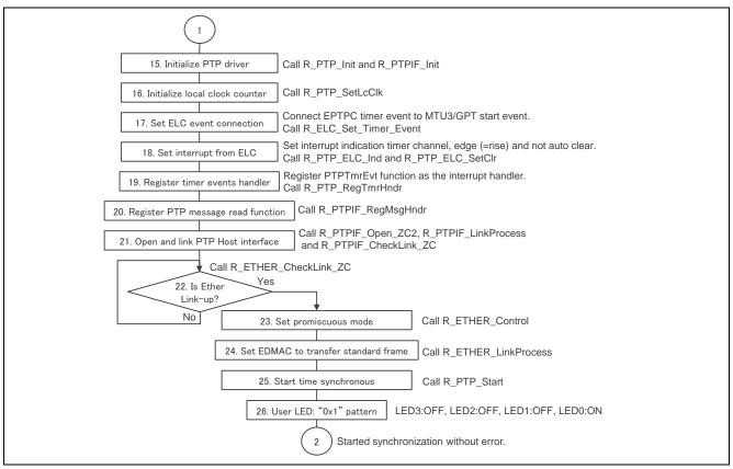
Figure 3.3 Synchronization initial setting
