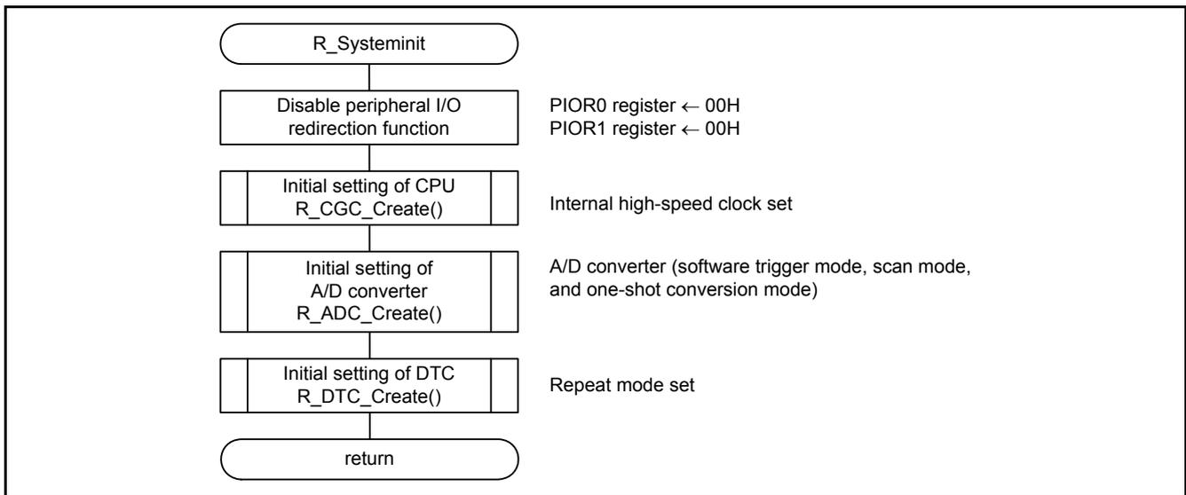
Figure 5.4 Initial Setting of Peripheral Functions
