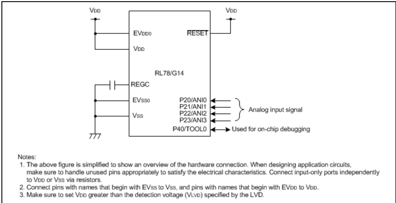
Figure 4.1 Hardware Configuration
