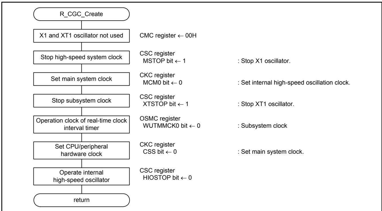
Figure 5.5 Initial Setting of the CPU
