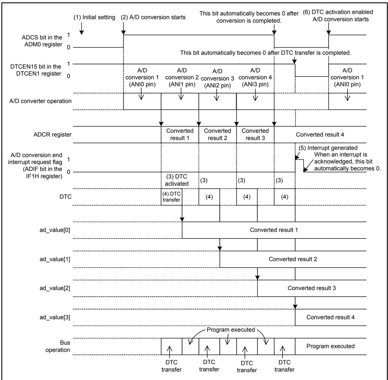
Figure 5.1 Timing Diagram of DTC Transfer and A/D Conversion
