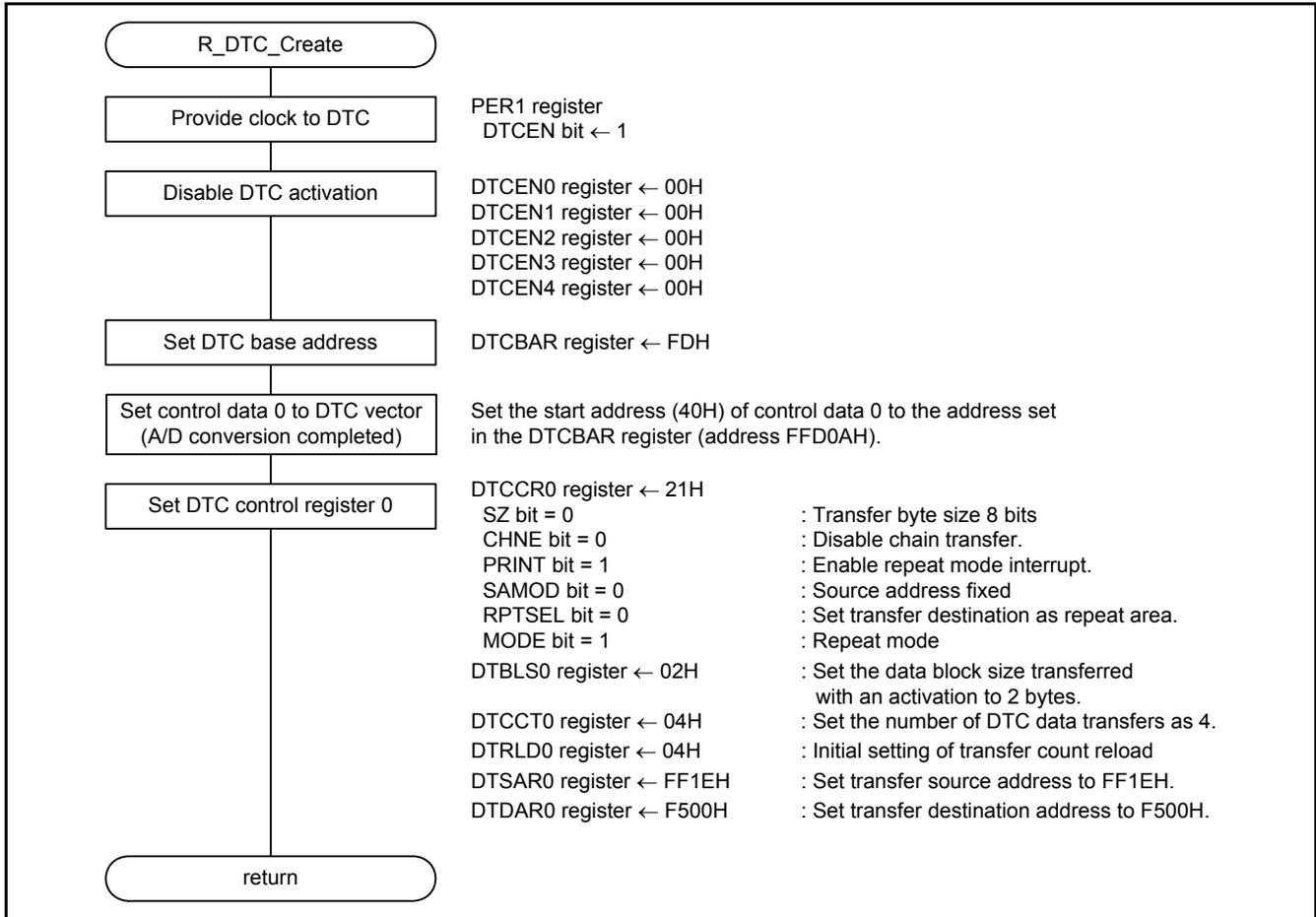
Figure 5.7 Initial Setting of the DTC
