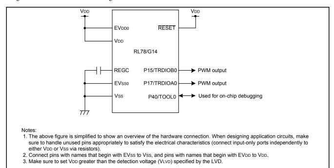
Figure 3.1 Hardware Configuration
