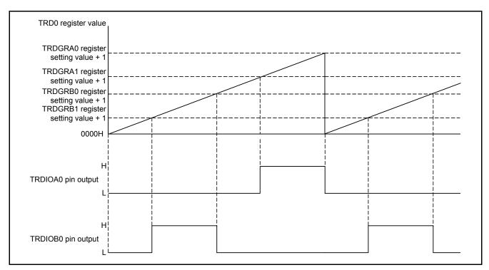
Figure 1.1 Output Timing Diagram
