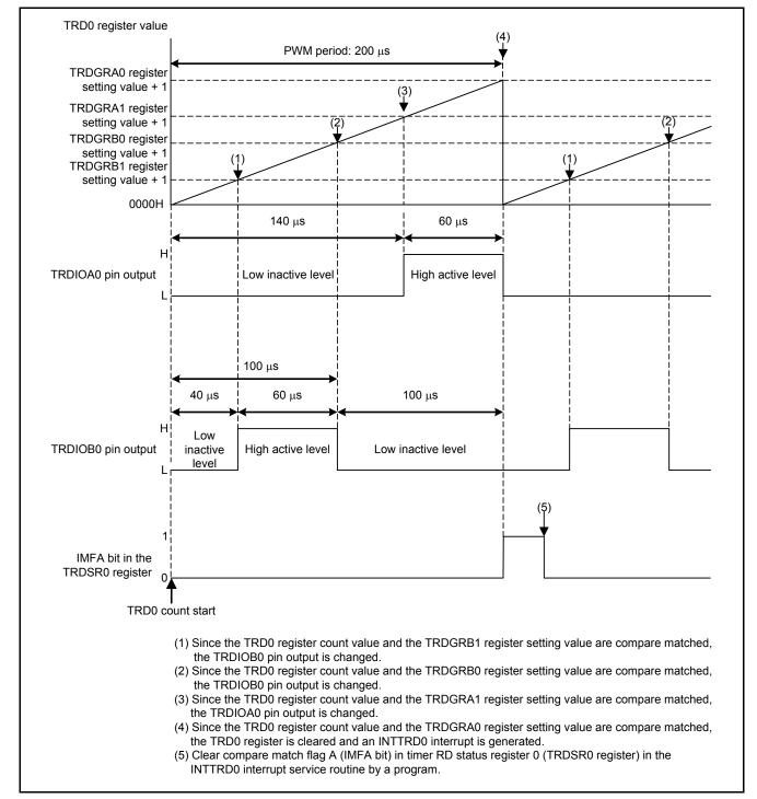
Figure 4.1 shows the PWM Output Waveform.
