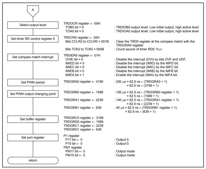
Figure 4.7 Initial Setting of Timer RD (2/2)
