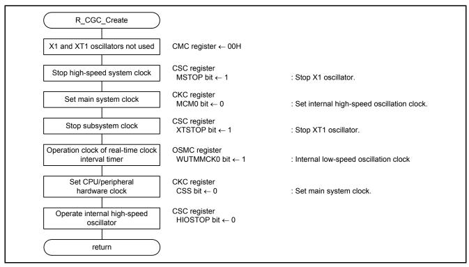
Figure 4.5 Initial Setting of the CPU
