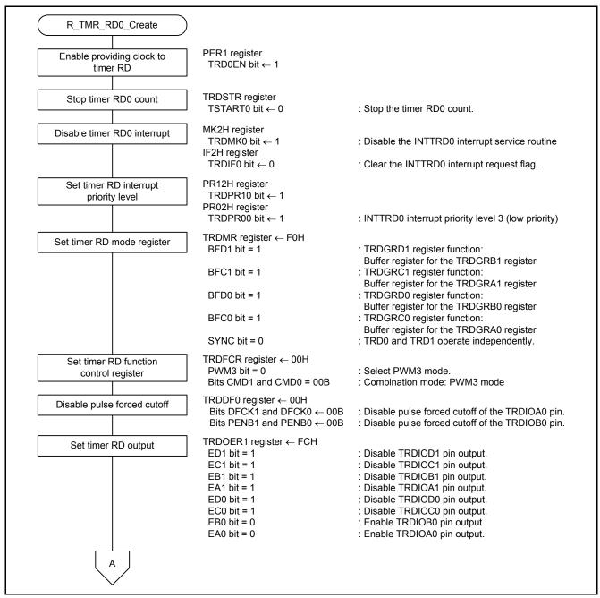
Figure 4.6 Initial Setting of Timer RD (1/2)
