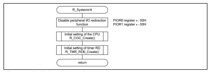
Figure 4.4 Initial Setting of Peripheral Functions
