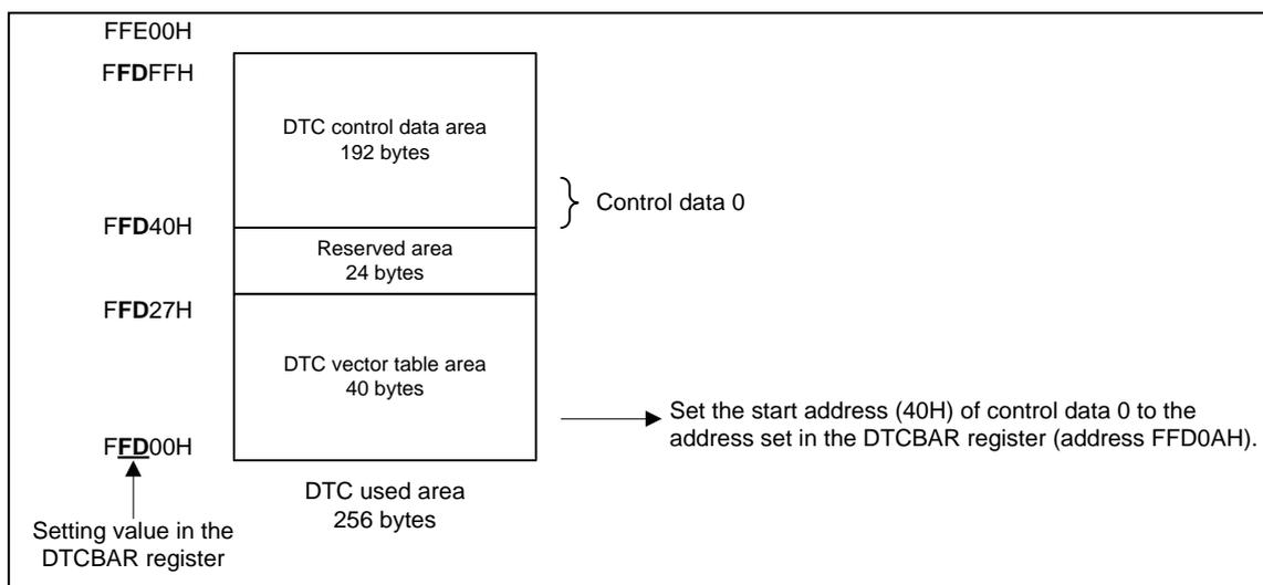
Figure 4.19 Memory Map of the DTC Used Area
