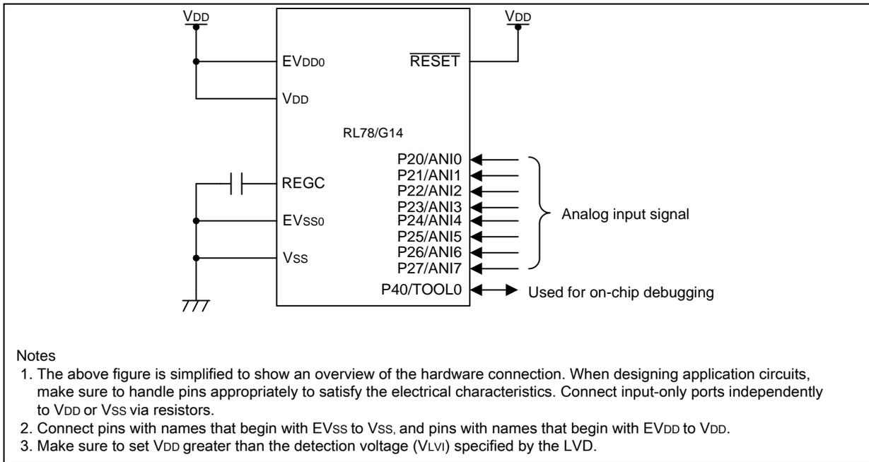
Figure 4.2 Hardware Configuration
