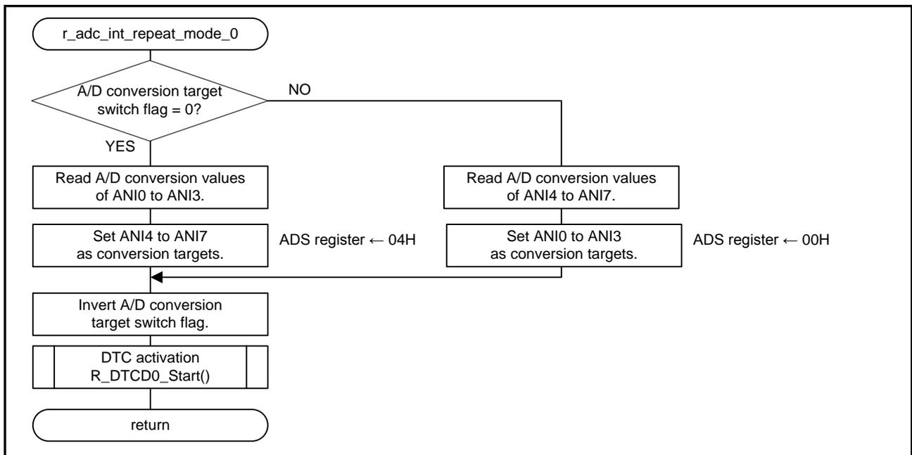
Figure 4.25 Interrupt Handling for Migration from the Repeat Sweep Mode 0
