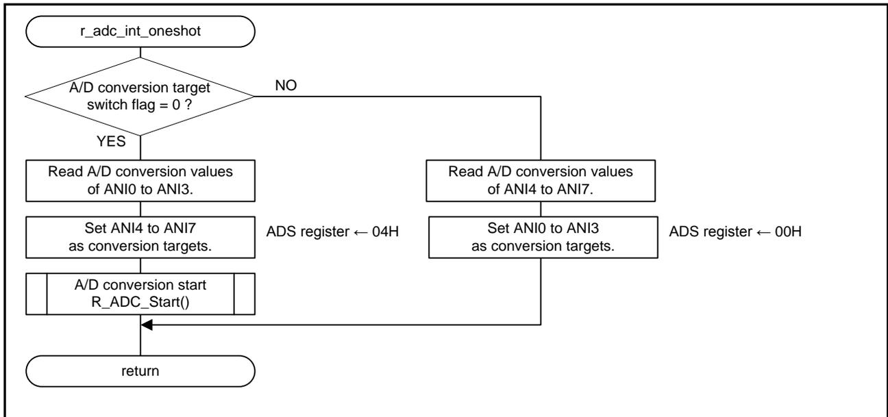
Figure 4.24 Interrupt Handling for Migration from the Single Sweep Mode
