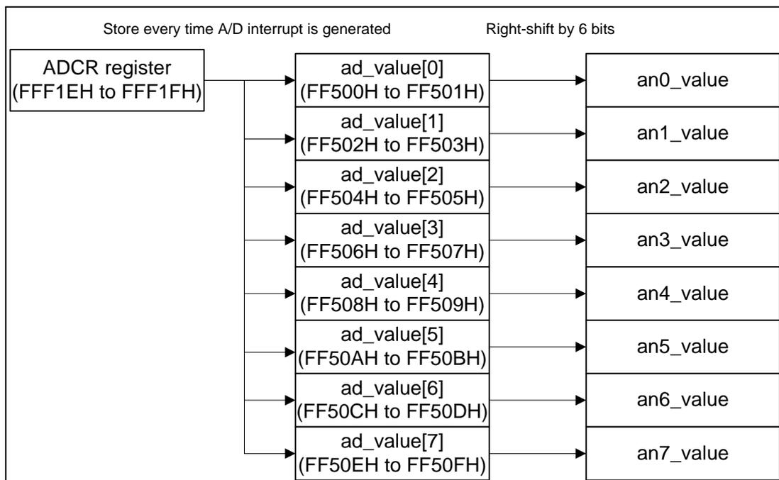
**Figure 4.7 Relationship between the ADCR Register and RAM
