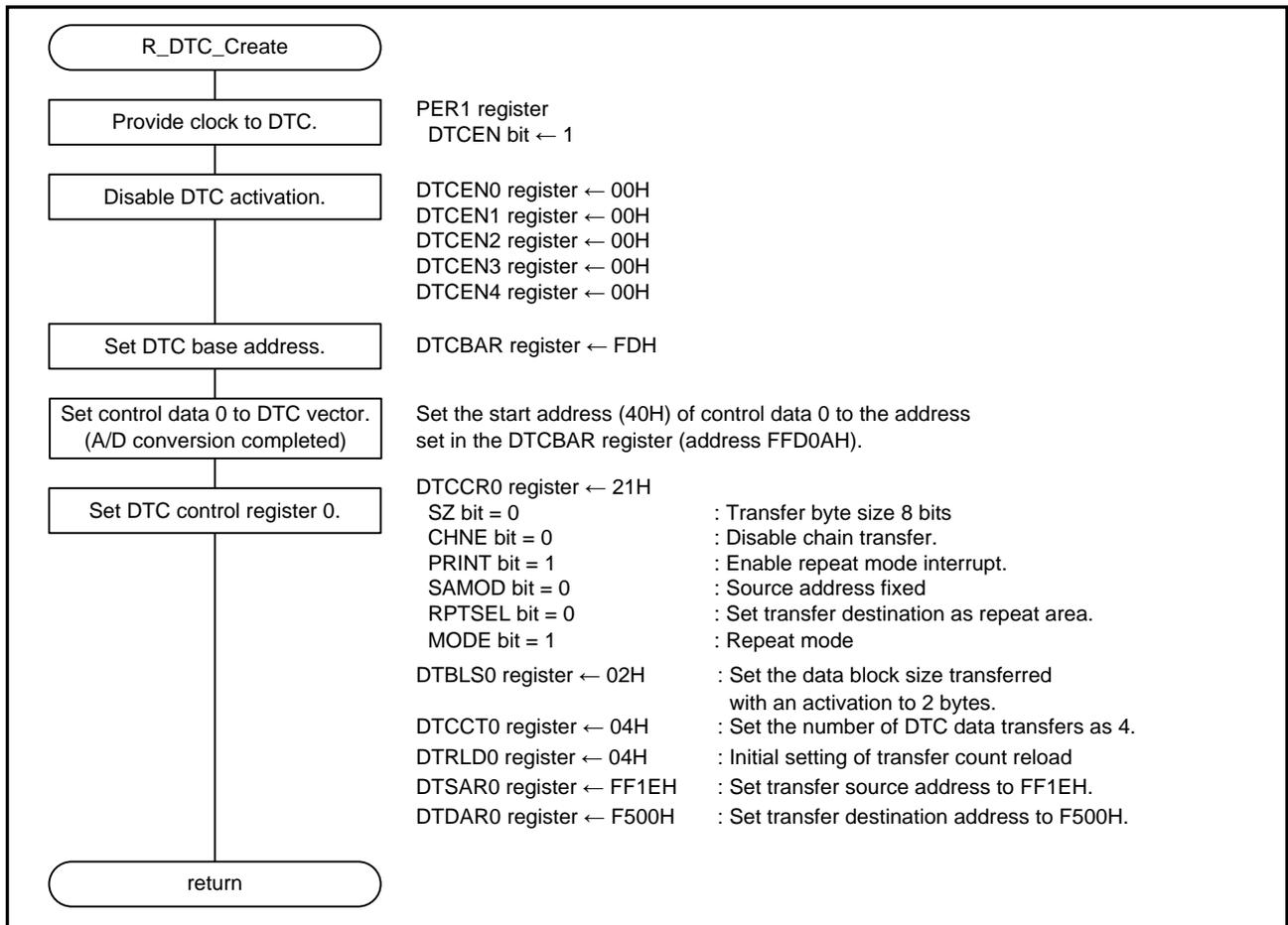
Figure 4.18 Initial Setting of DTC
