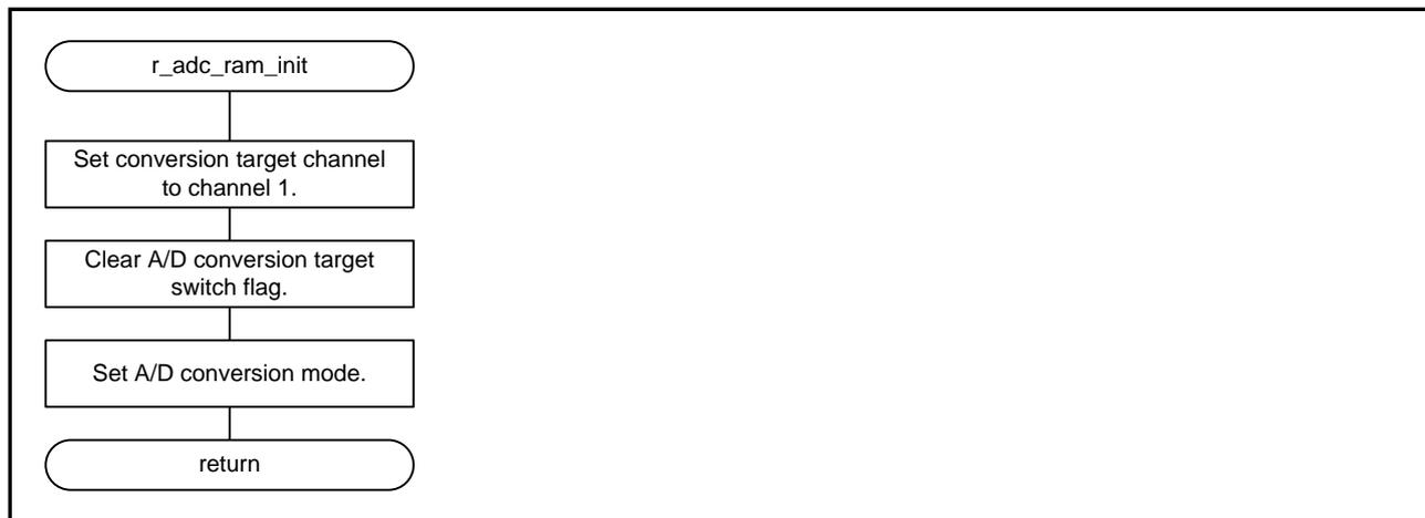
**Figure 4.17 Initialization of Variables Associated with A/D Conversion**
