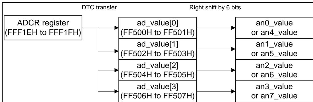
**Figure 4.6 Relationship between the ADCR Register and RAM (Example of Migration from the Repeat Sweep Mode 0)**
