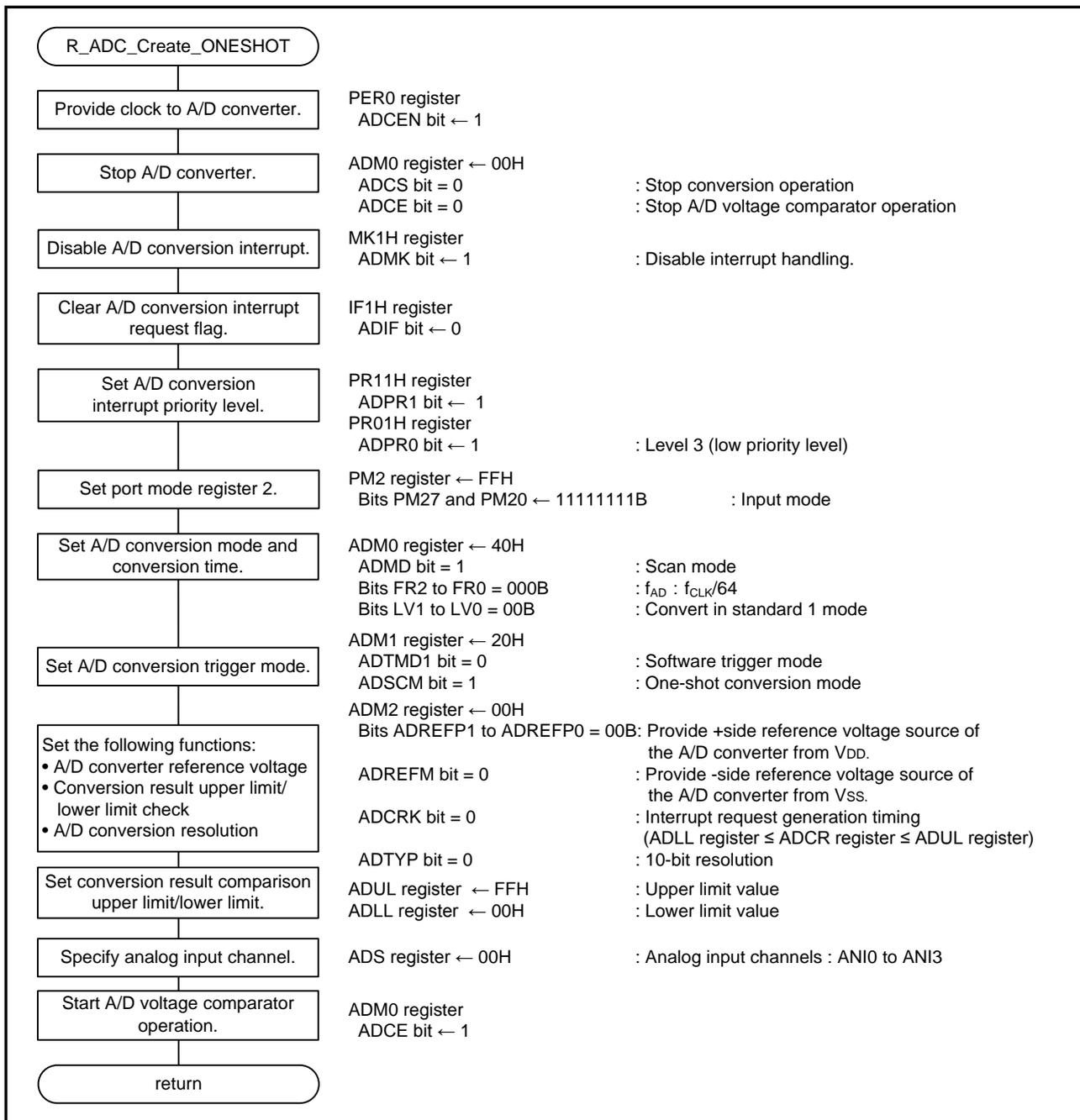
Figure 4.14 Initial Setting for Migration from the Single Sweep Mode
