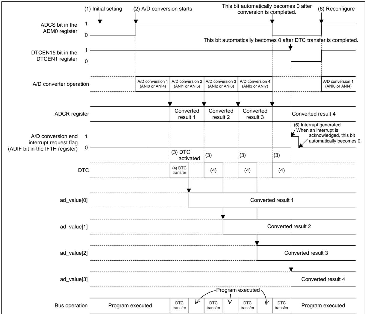
**Figure 4.5 Timing Diagram of DTC Transfer and A/D Conversion (Example of Migration from the Repeat Sweep Mode 0)**
