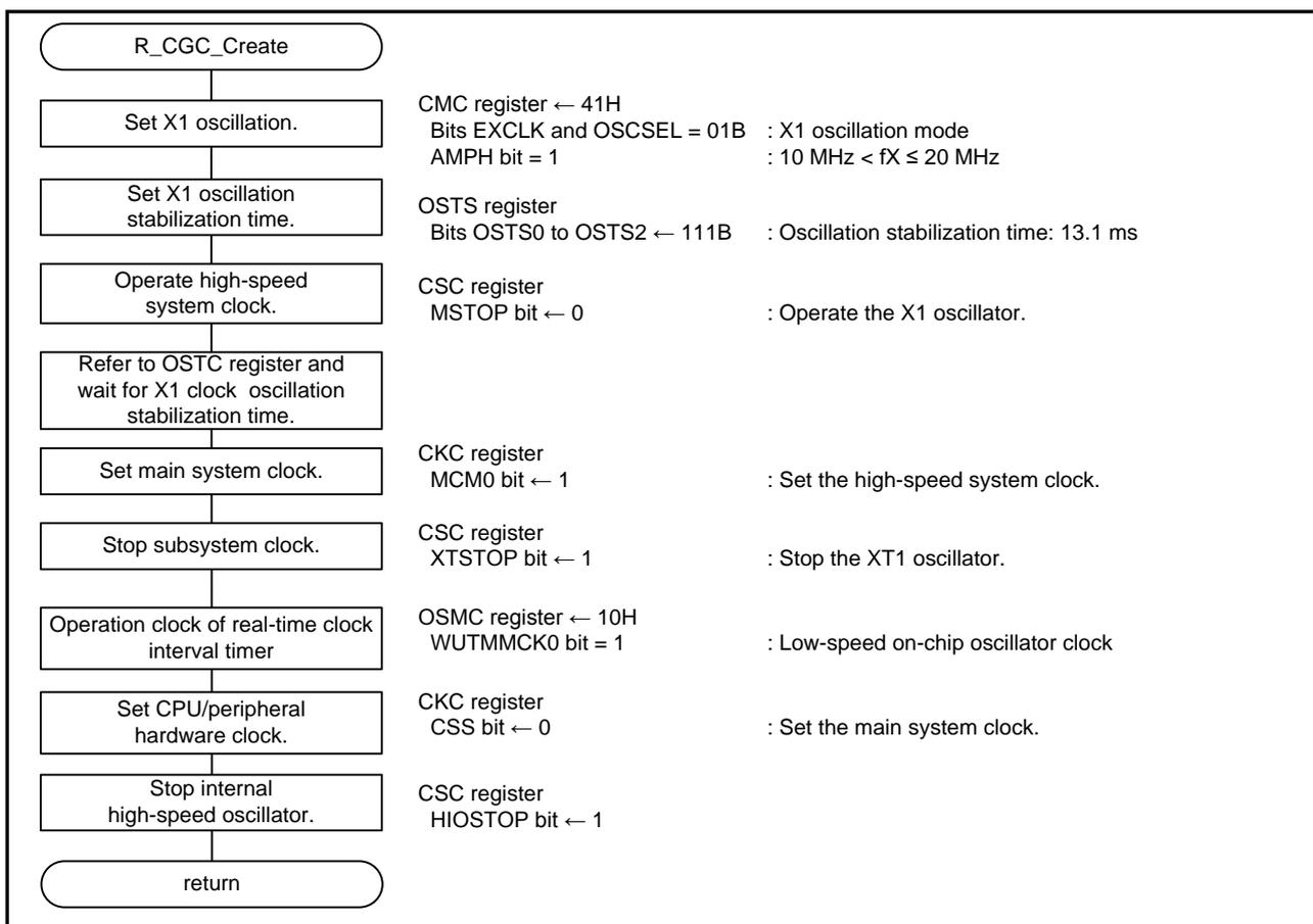
Figure 4.11 Initial Setting of CPU
