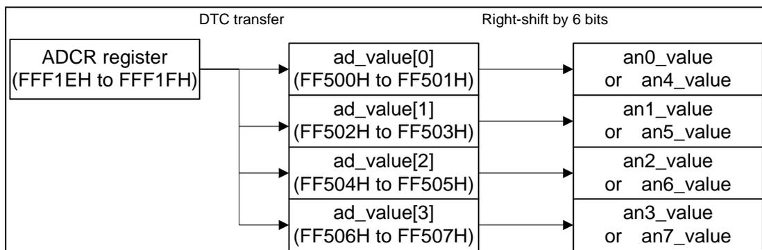
**Figure 4.4 Relationship between the ADCR Register and RAM (Example of Migration from the Single Sweep Mode)**
