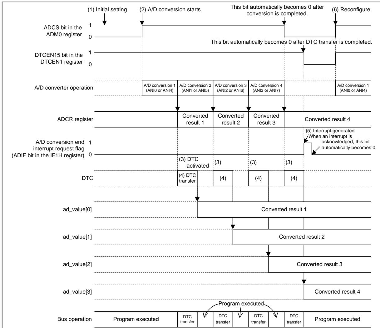
**Figure 4.3 Timing Diagram of DTC Transfer and A/D Conversion (Example of Migration from the Single Sweep Mode)**
