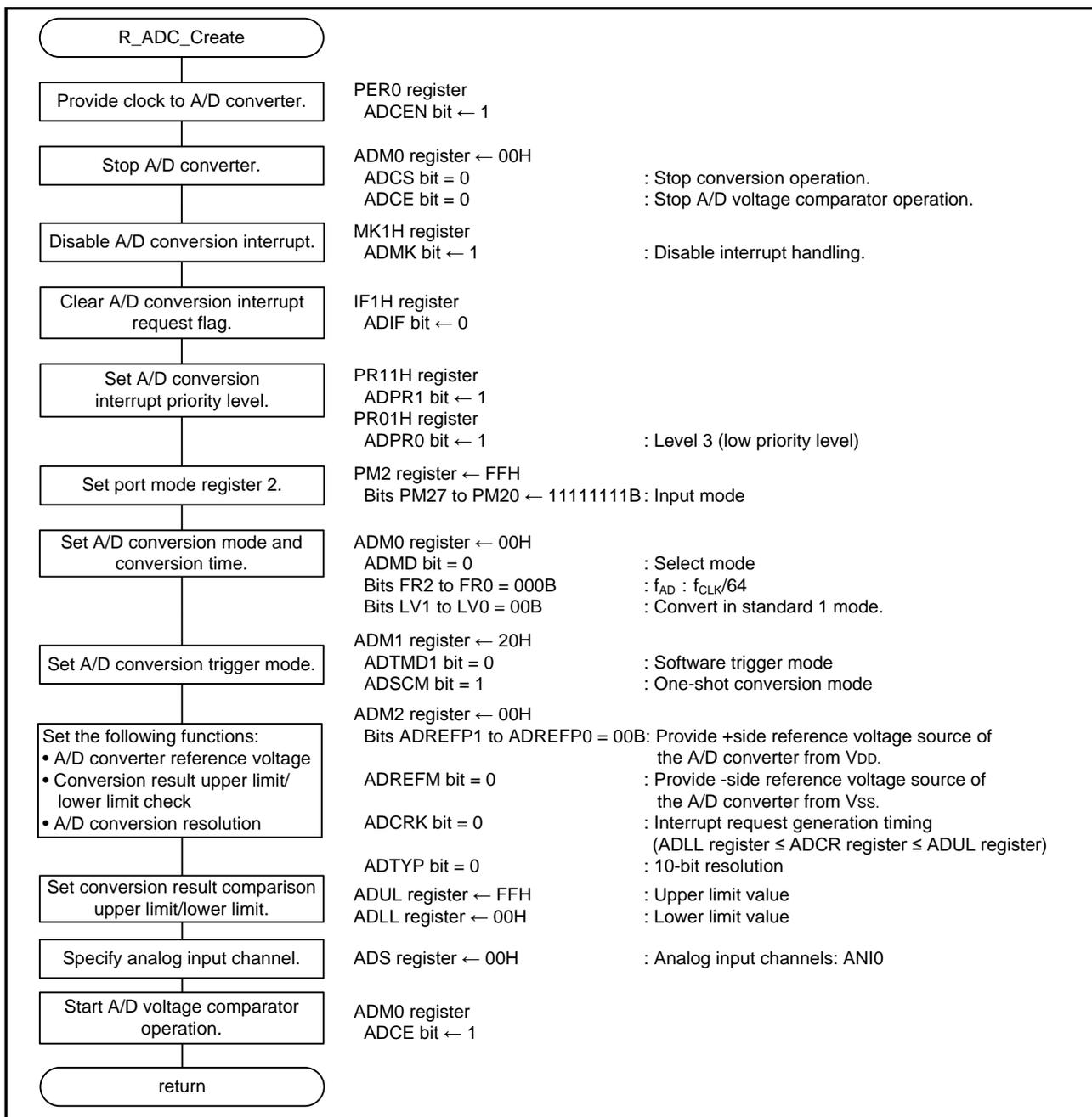
Figure 4.12 Initial Setting of the A/D Converter
