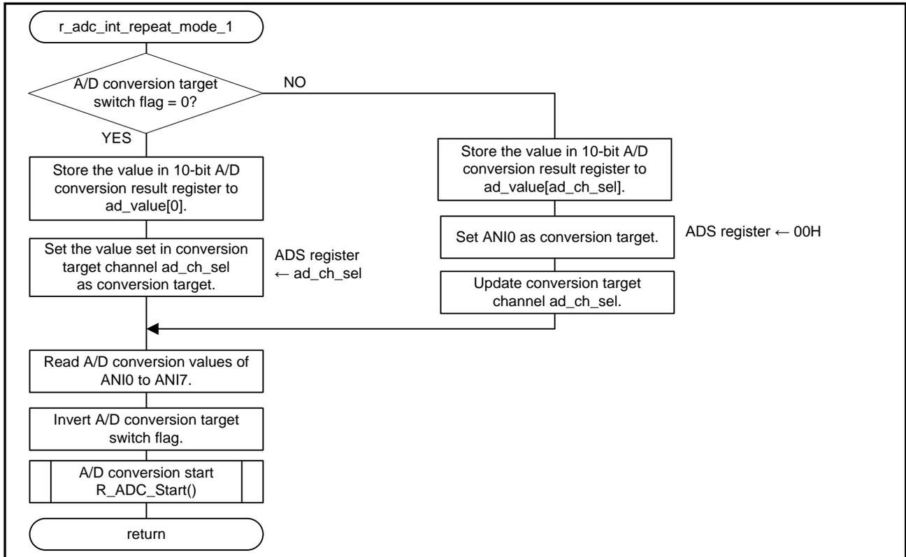
Figure 4.26 Interrupt Handling for Migration from the Repeat Sweep Mode 1
