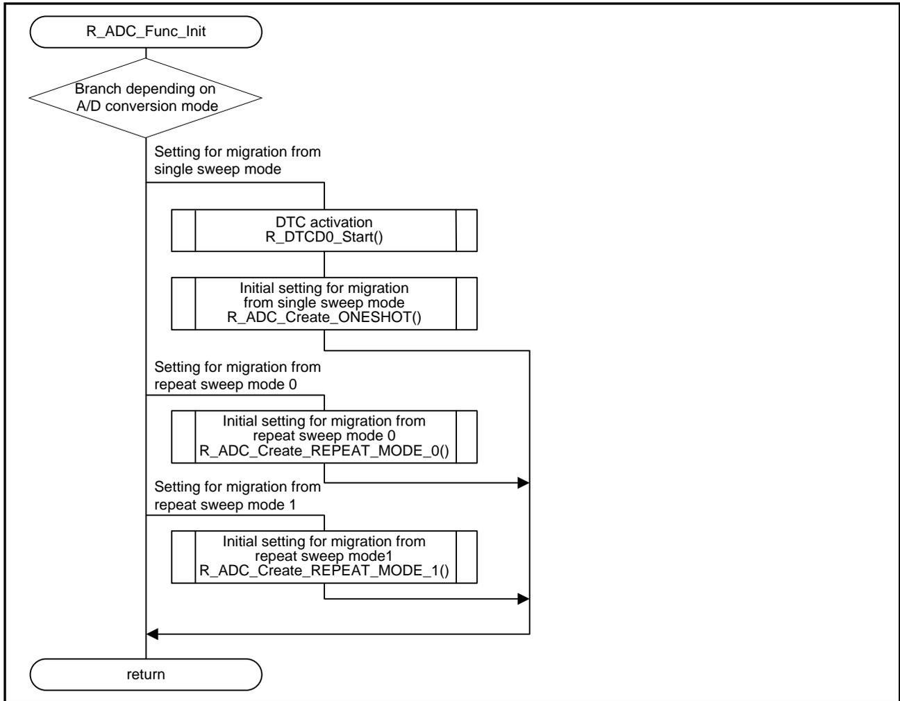
Figure 4.13 Initial Setting Depending on A/D Conversion Functions
