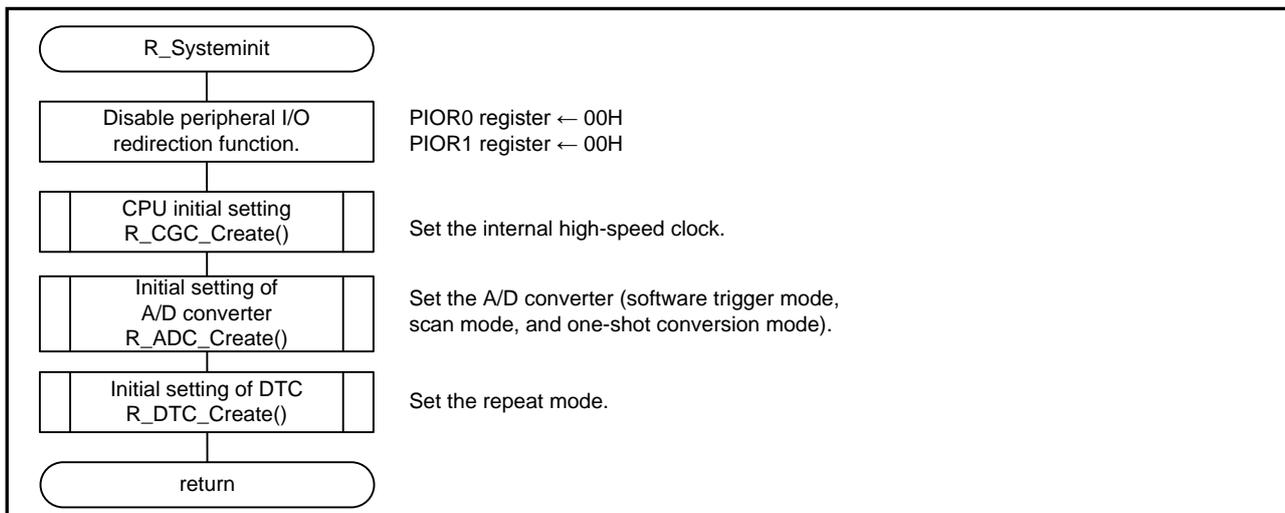
Figure 4.10 Initial Setting of Peripheral Functions
