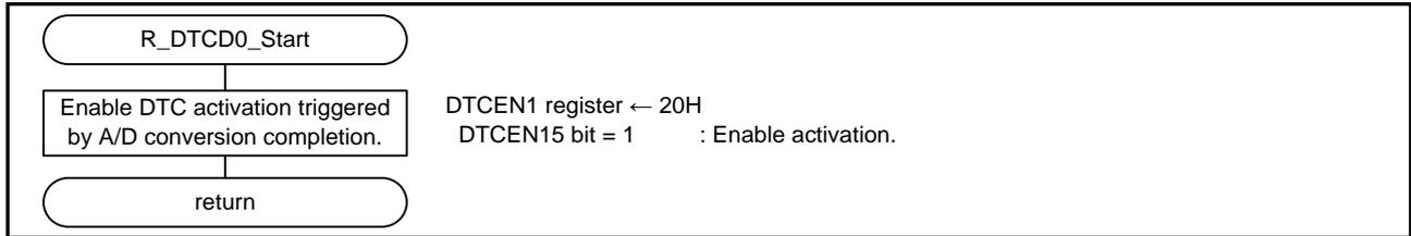
Figure 4.21 DTC Activation
