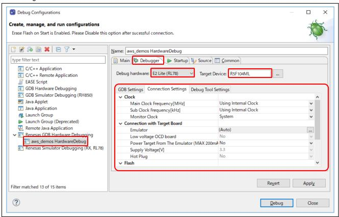
Figure 5.2 Hardware Debugging Settings
