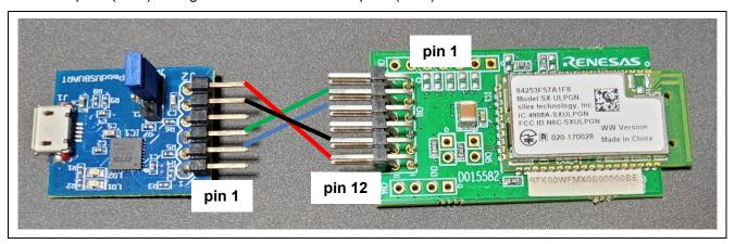
Figure 4.5 Connections between Digilent Pmod USBUART and SX-ULPGN
