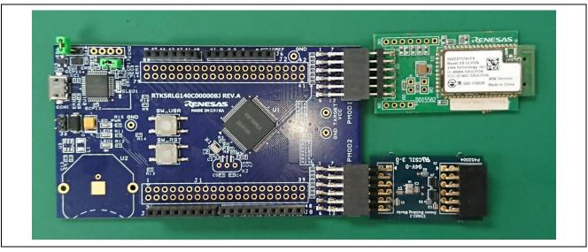
Figure 4.1 RL78/G14 Fast Prototyping Board and Wi-Fi Module (SX-ULPGN (Silex Technology))
