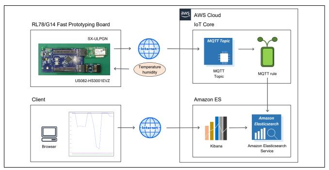
Figure 1.1 System Diagram from Acquisition of Sensor Information to Visualization
