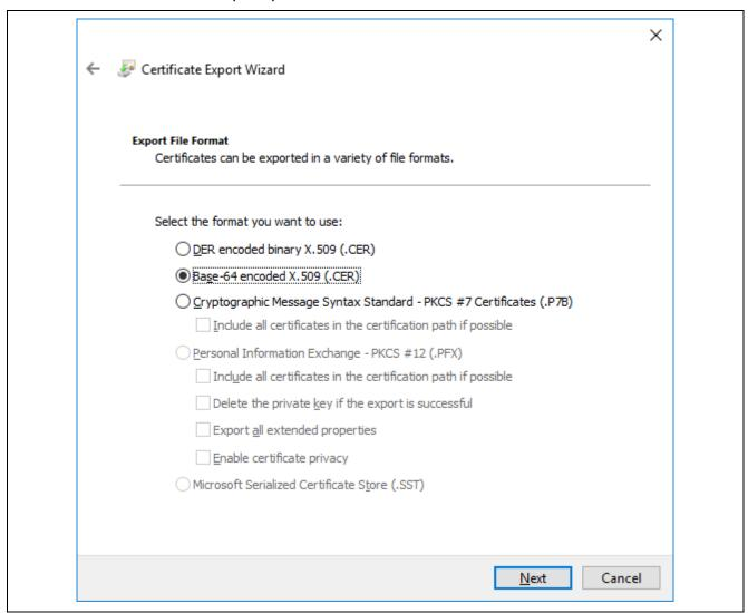
Figure 4.3 Selecting Base 64 encoded X.509 (.CER)
