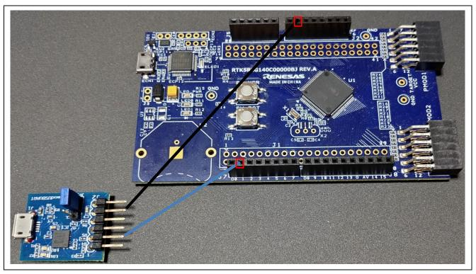
Figure 4.8 Connecting the Digilent Pmod USBUART to the RL78/G14 Fast Prototyping Board
