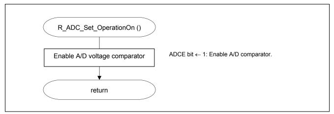
Figure 5.8 Enabling A/D Voltage Comparator
