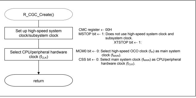
Figure 5.5 CPU Clock Setup
