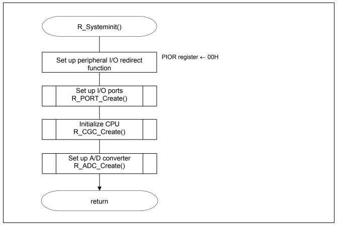
Figure 5.3 System Initialization Function
