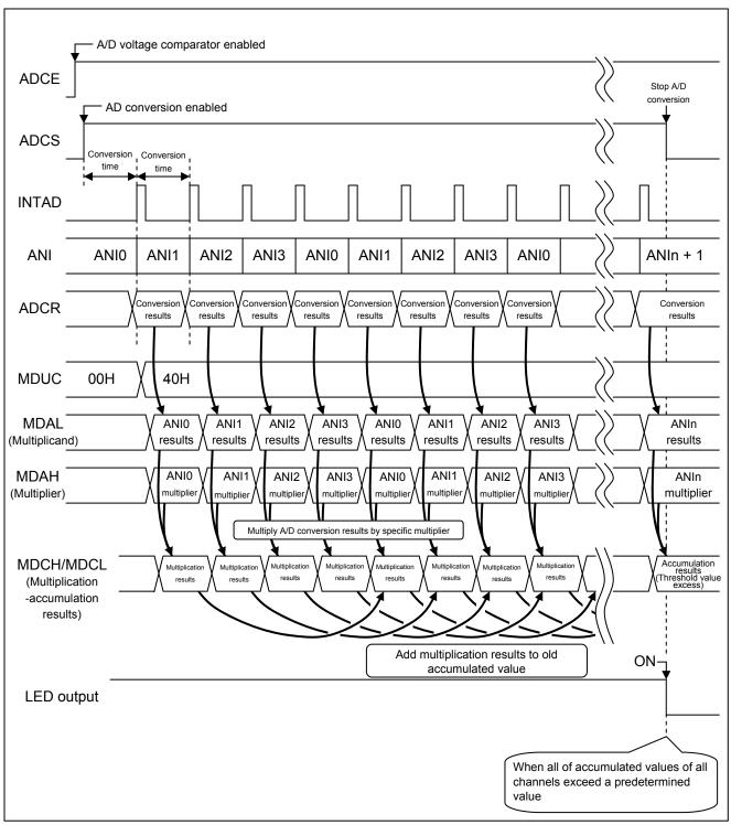
Figure 1.2 Outline of Multiplication-Accumulation Operation
