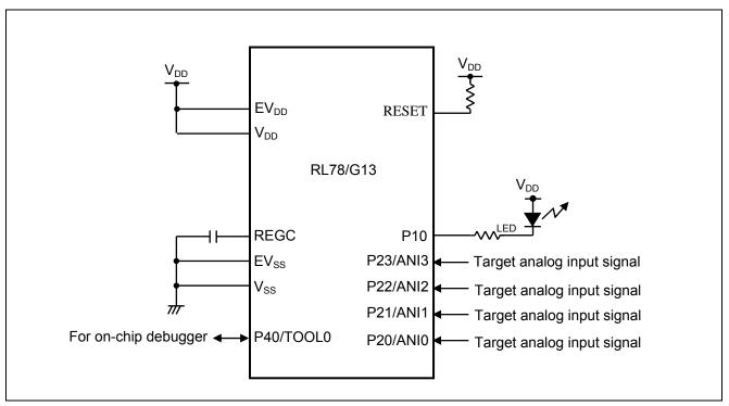
Figure 4.1 Hardware Configuration
