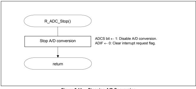
Figure 5.11 Stopping A/D Conversion
