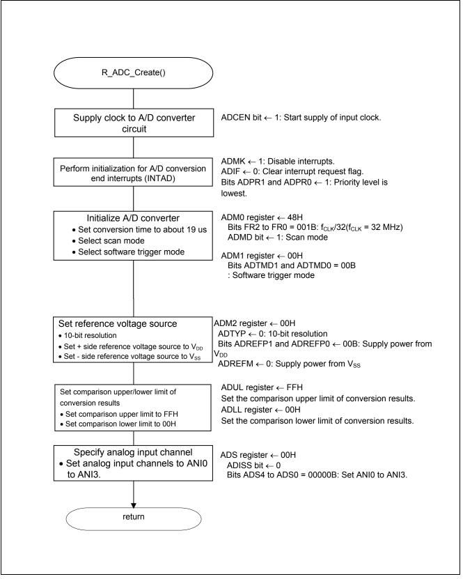
Figure 5.6 A/D Converter Setup
