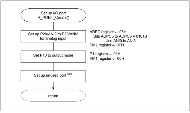
Figure 5.4 I/O Port Setup
