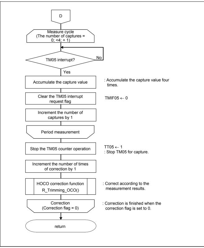
Figure 5.13 Calibration with XT1 Oscillation (2/2)
