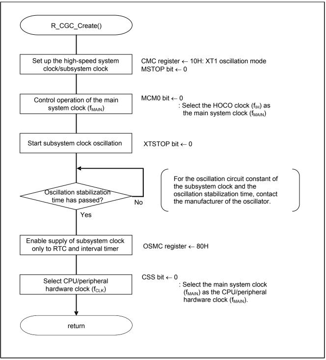
Figure 5.5 CPU Clock Setup
