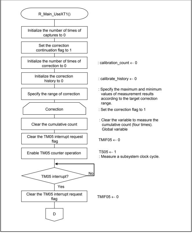
Figure 5.12 Calibration with XT1 Oscillation (1/2)
