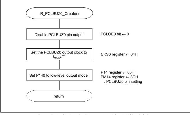
Figure 5.8 Clock Output/Buzzer Output Control Circuit Setup
