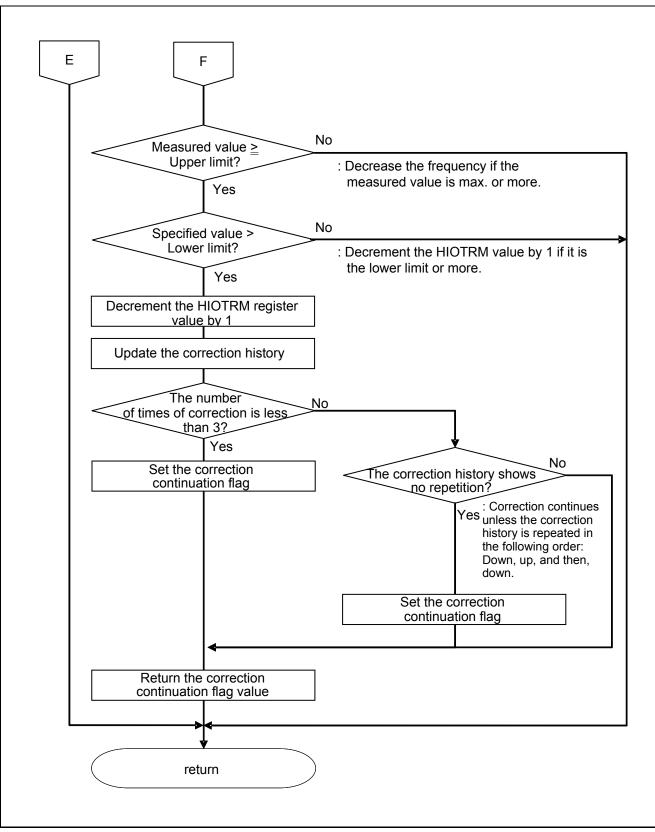
Figure 5.16 HOCO Correction Function (2/2)
