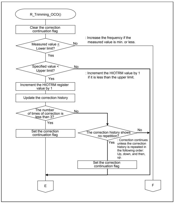
Figure 5.15 HOCO Correction Function (1/2)
