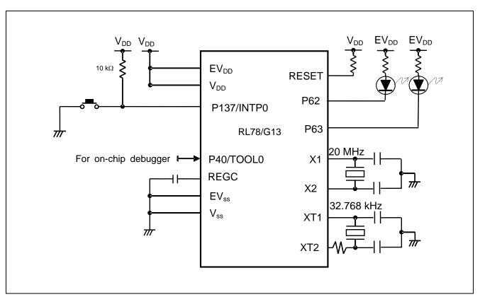
Figure 4.1 Hardware Configuration
