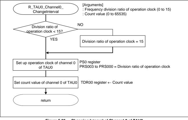
Figure 5.23 Changing Interval of Channel 0 of TAU0
