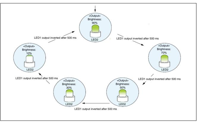
Figure 1.1 Overview of PWM Output Operation
