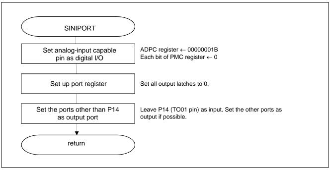
Figure 5.3 I/O Port Setup
