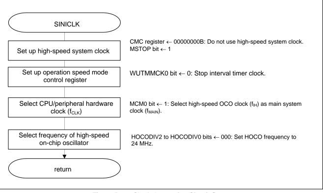
Figure 5.4 Clock Generation Circuit Setup
