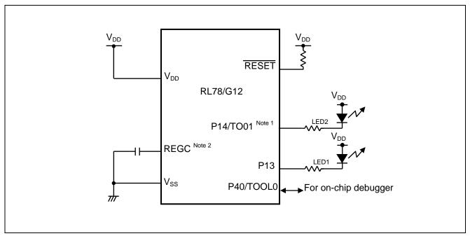
Figure 4.1 Hardware Configuration
