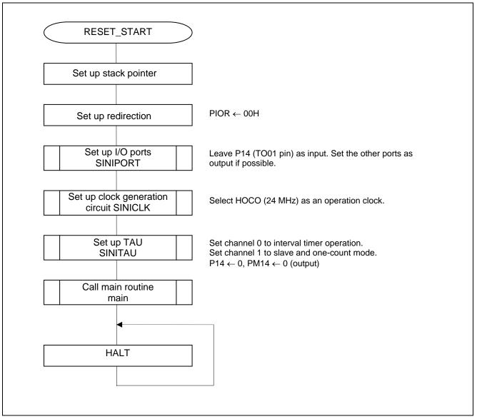
Figure 5.2 CPU Initialization Function
