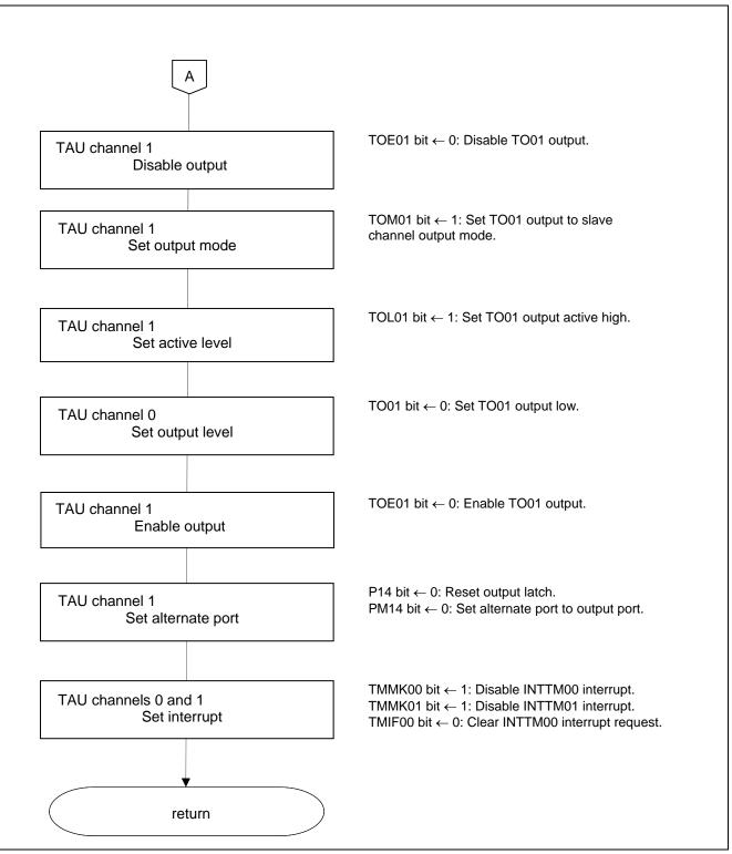
Figure 5.5 Timer Array Unit Setup (2/2)
