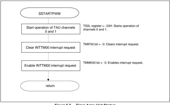
Figure 5.7 Timer Array Unit Startup
