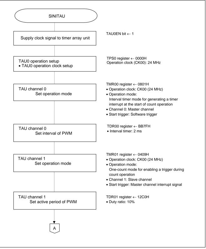
Figure 5.5 Timer Array Unit Setup (1/2)
