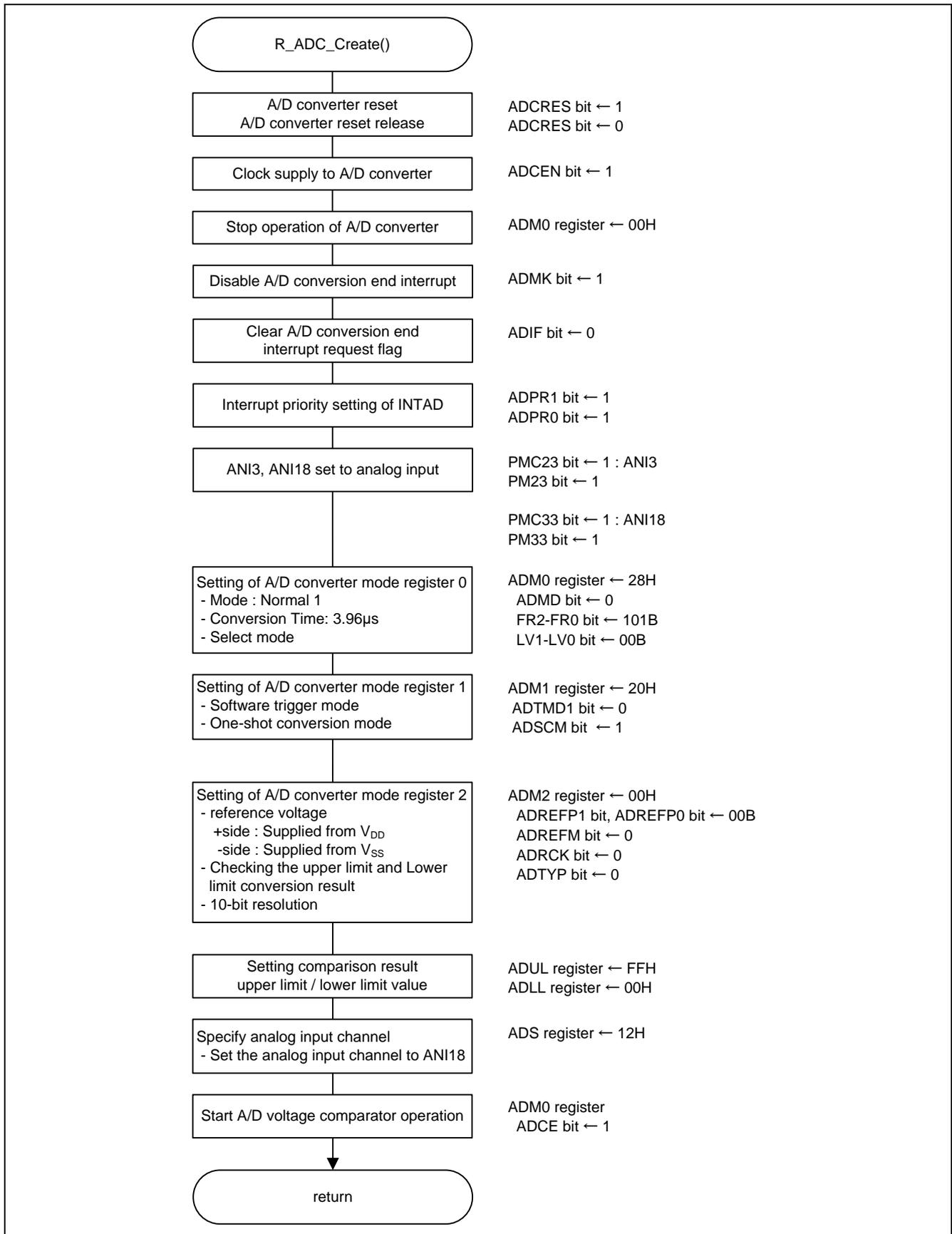
Figure 5.11 A/D Converter Initial Setting
