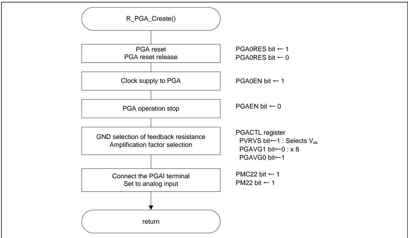
Figure 5.7 Programmable gain amplifier (PGA) Initial Setting
