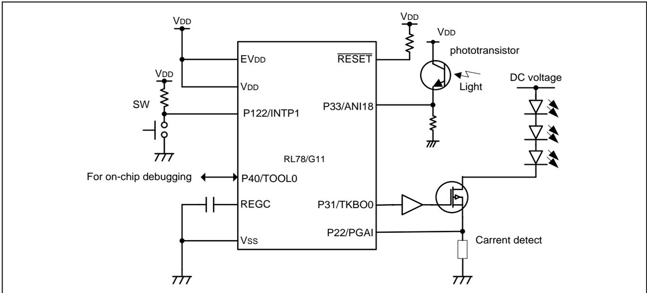
Figure 4.1 Hardware Configuration
