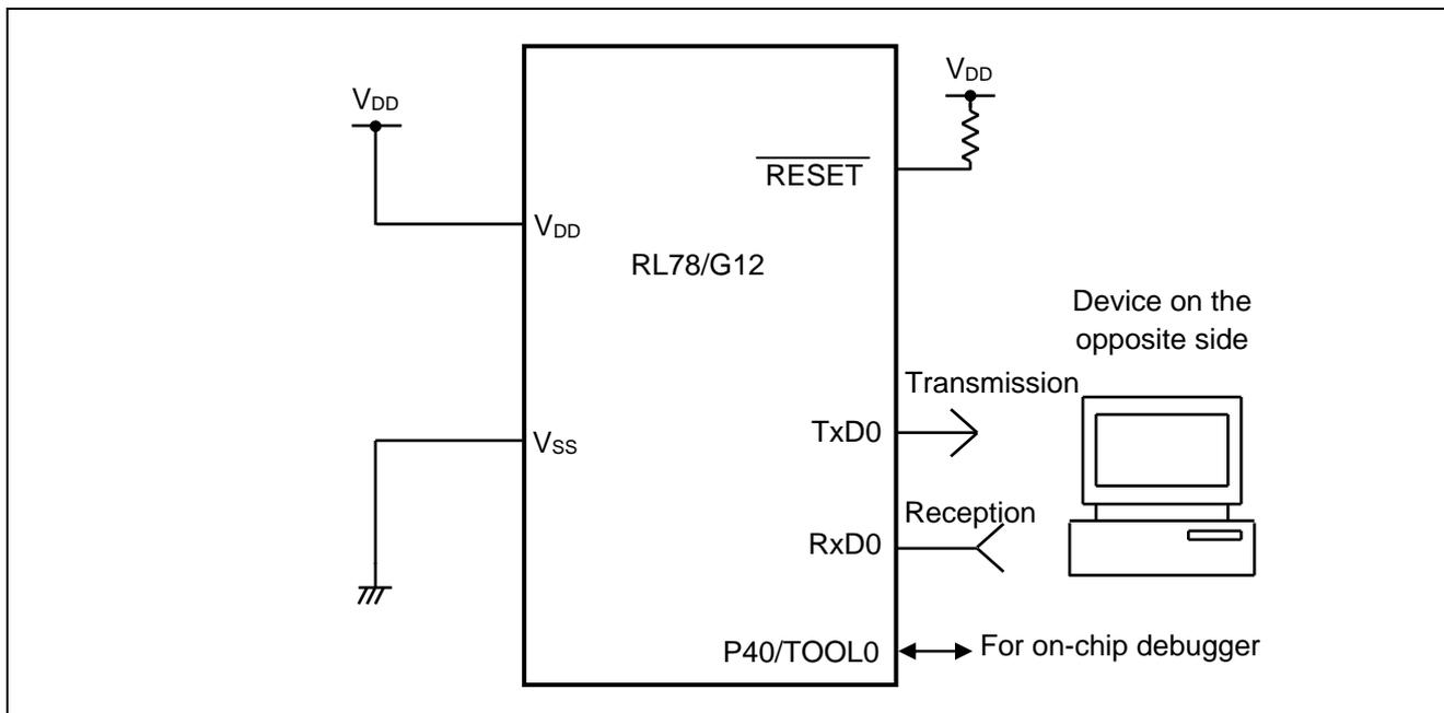
**Figure 4.1 Hardware Configuration**
