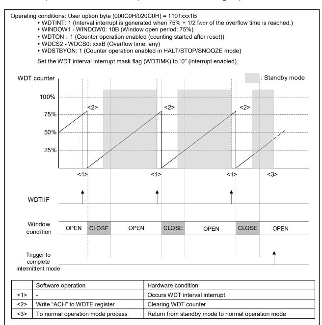
Figure 2-1 Processing Example when Using the WDT Function
