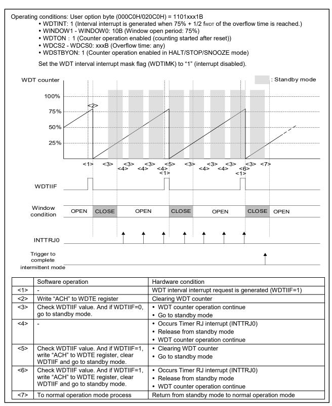
Figure 2-2 Processing Example when Using Timer RJ
