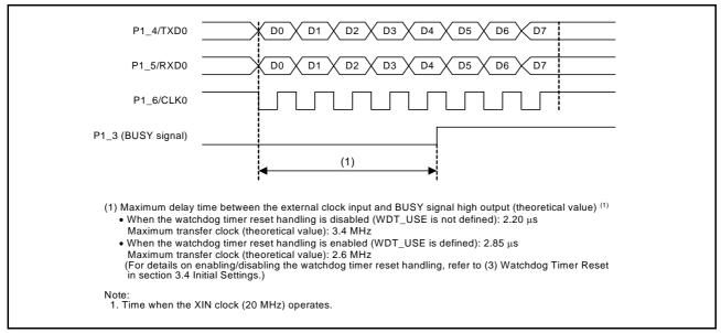
Figure 3.6 Timing between Transfer Clock Input and the BUSY Signal Becoming High
