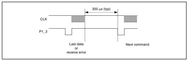
Figure 5.1 Serial Communication Provision
