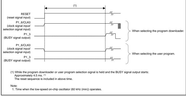
Figure 3.5 Signal Control Timing after Reset
