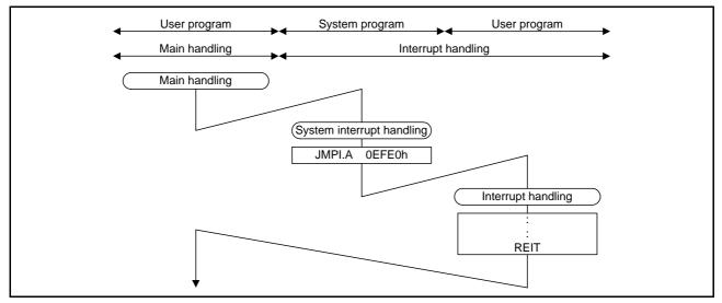
Figure 3.4 System Interrupt Operation (Overflow Interrupt)
