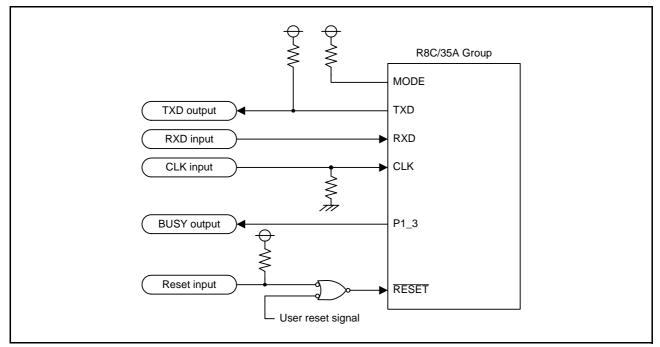
Figure 7.1 Programmer Configuration
