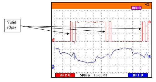
Figure 9 Filtered Back EMF and comparator output
