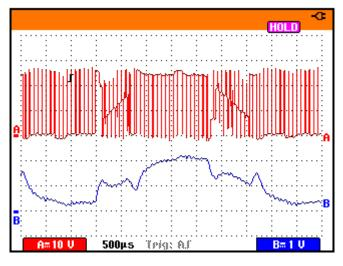
Figure 3 Raw and filtered motor voltage
