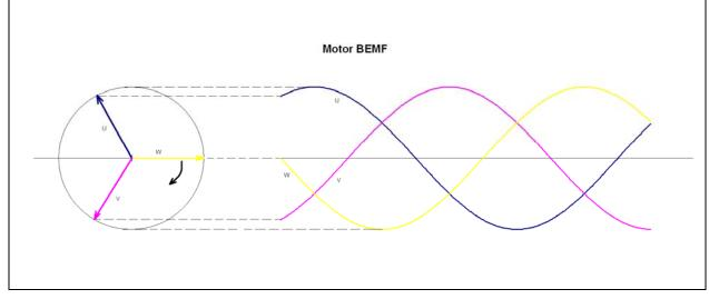
Figure 2 Rotating vector representation of motor phases
