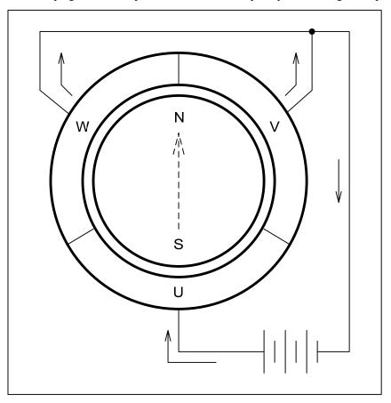
Figure 7 Concept of alignment current
