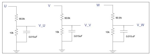
Figure 4 Filtering and Scaling of phase voltages to match the logic levels
