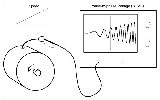
Figure 1 Voltage and frequency measured externally at rotating BLDC motor
