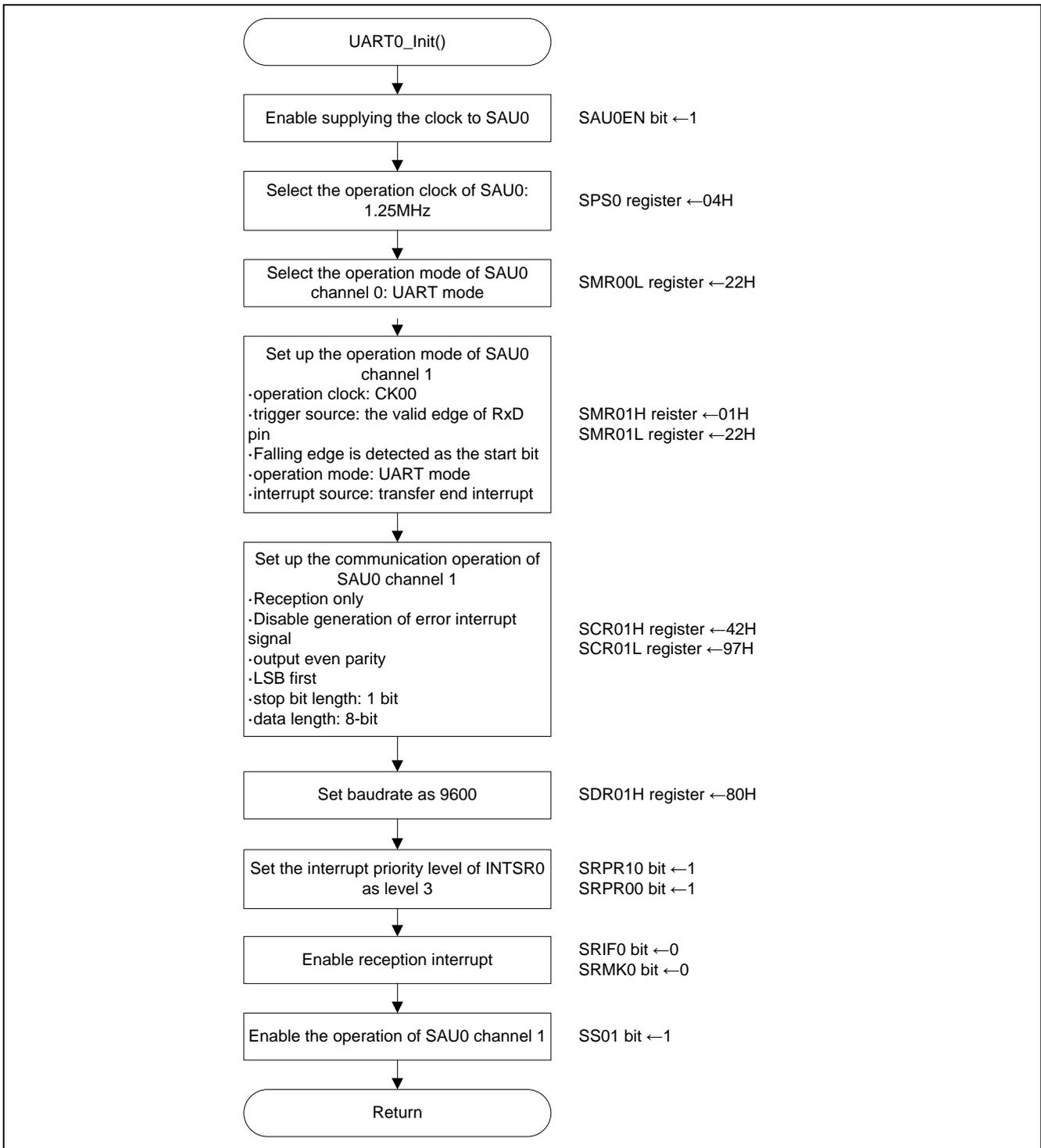
Figure 5.5 Initial Setting of Serial Array Unit
