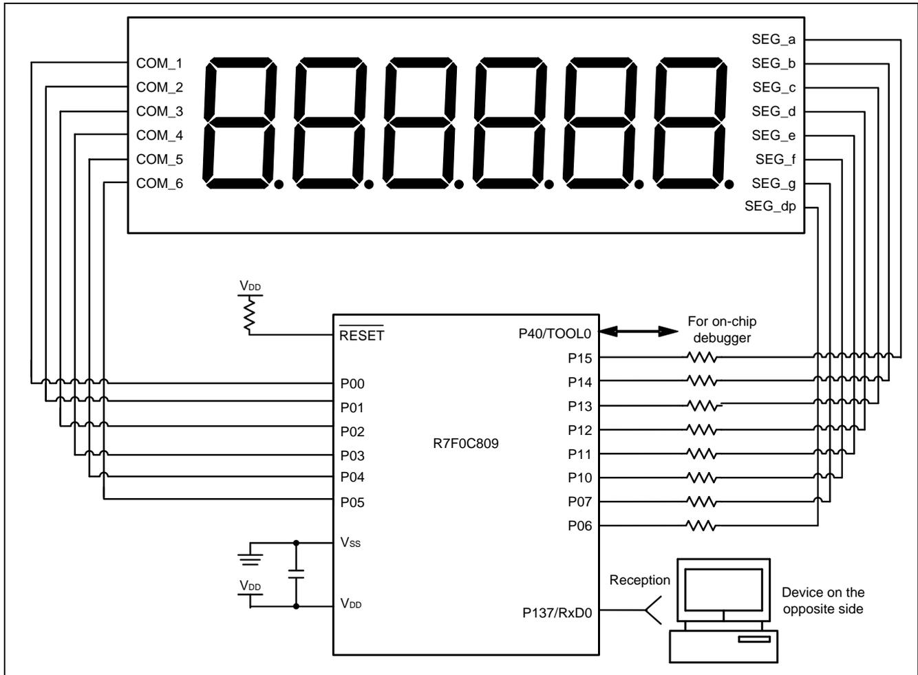
**Figure 4.1 Hardware Configuration**
