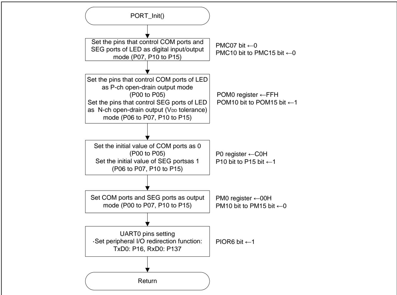
Figure 5.3 Initial Setting of I/O ports
