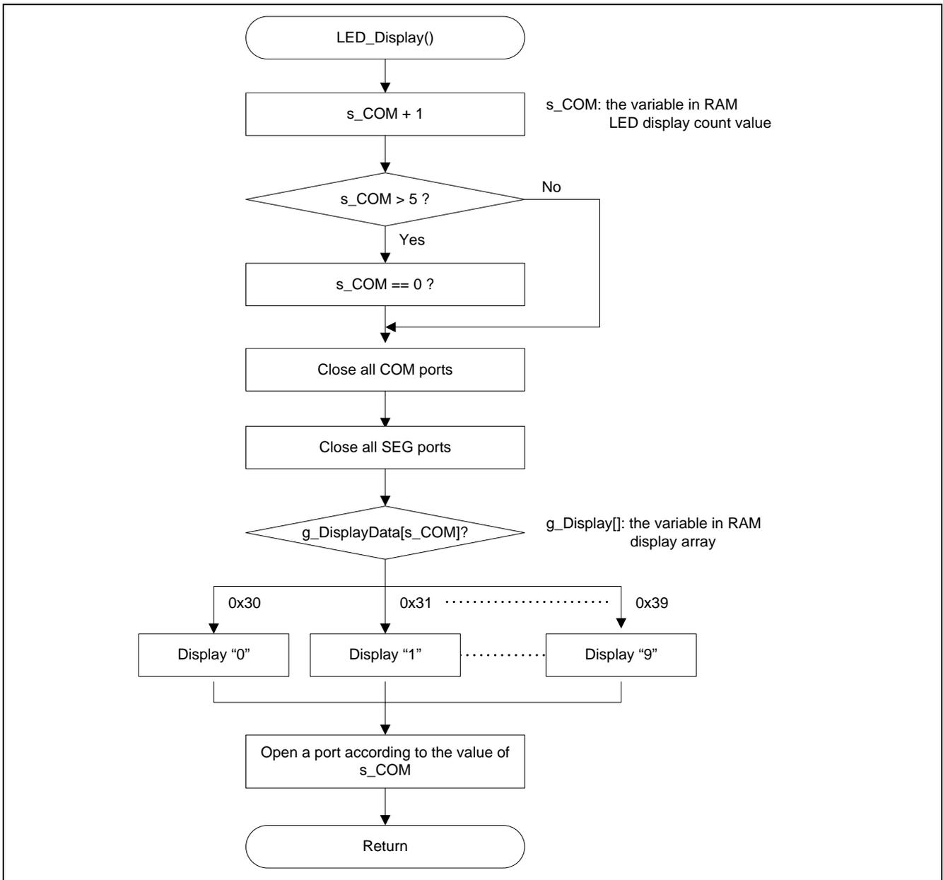
Figure 5.9 LED Display Function
