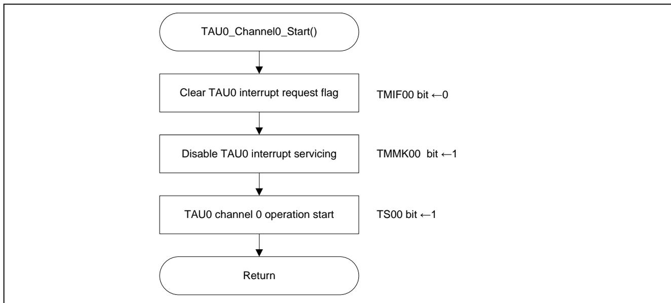
**Figure 5.7 Start the Operation of Timer Array Unit 0**
