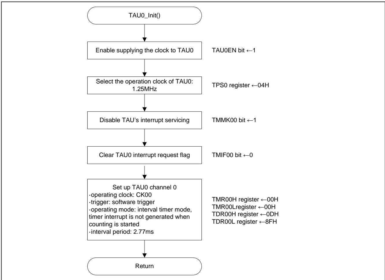
Figure 5.4 Initial Setting of Timer Array Unit
