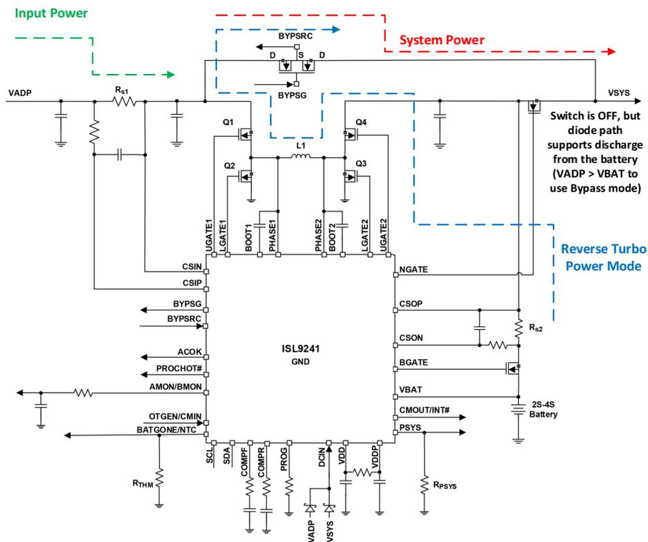
Figure 3. Reverse Turbo Boost with Battery Charging
