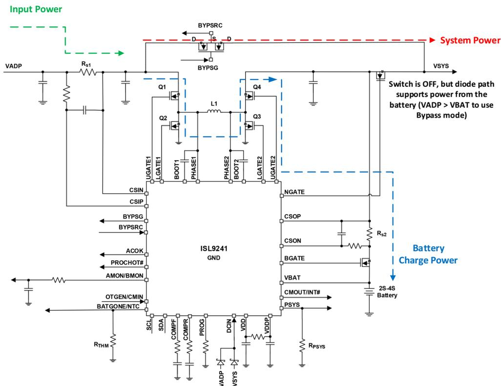
Figure 2. Bypass Mode with Battery Charging
