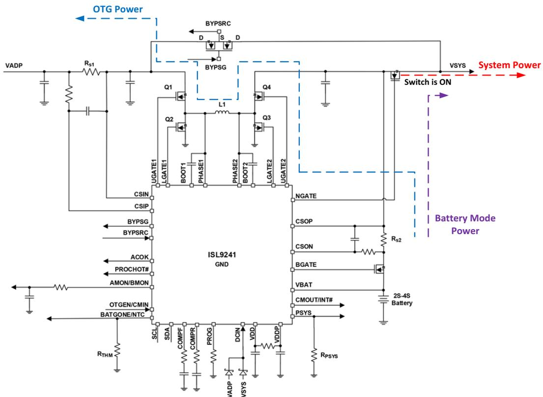
Figure 4. Battery Only Mode and OTG Mode
