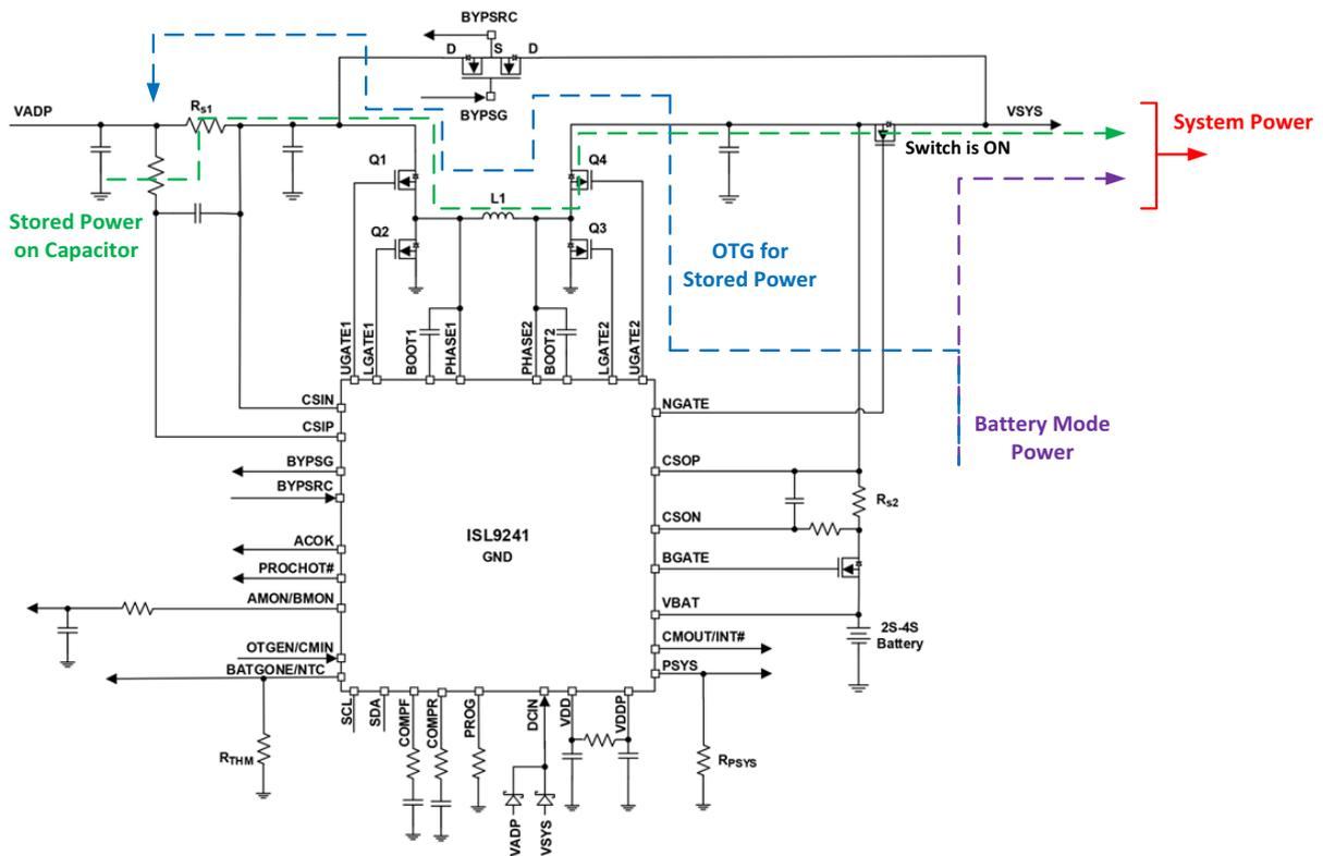
Figure 5. Supplemental Mode (Intel VMIN Active Protection)
