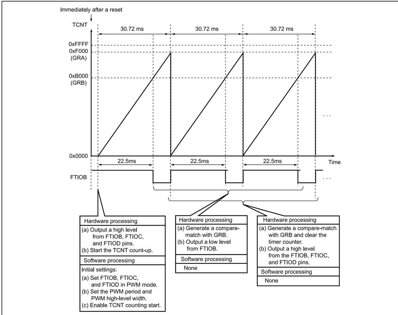
Figure 3.1 Principle of Operation: Output of PWM Waveform by Using PWM Mode of Timer W
