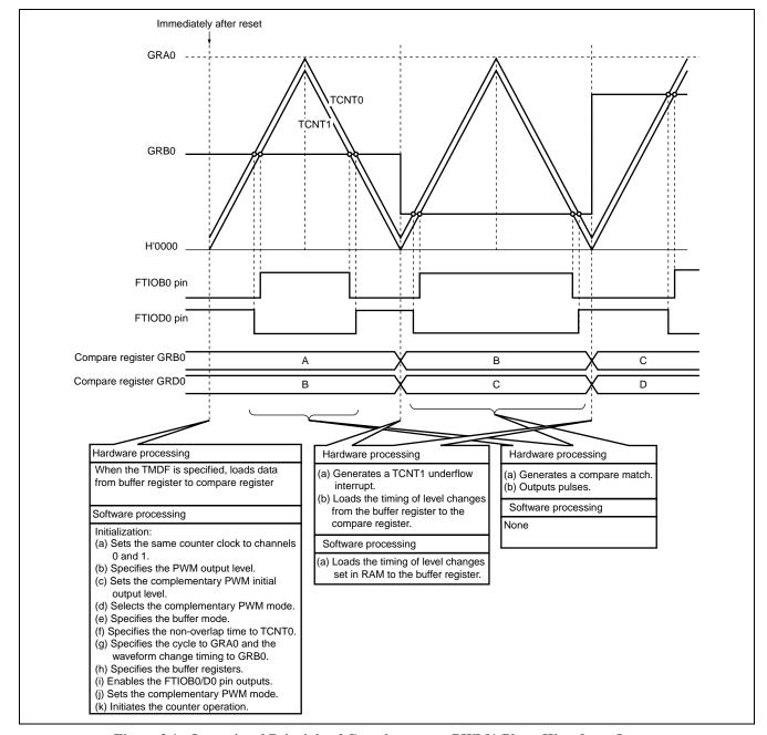
Figure 3.1 Operational Principle of Complementary PWM1-Phase Waveform Output
