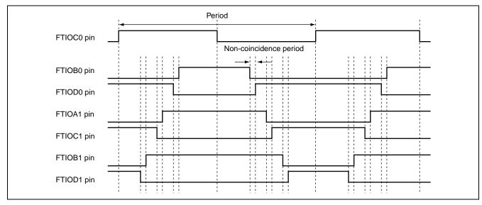
Figure 1.1 Output of Three Complementary (Normal and Inverse Phase) Pairs of PWM Signals
