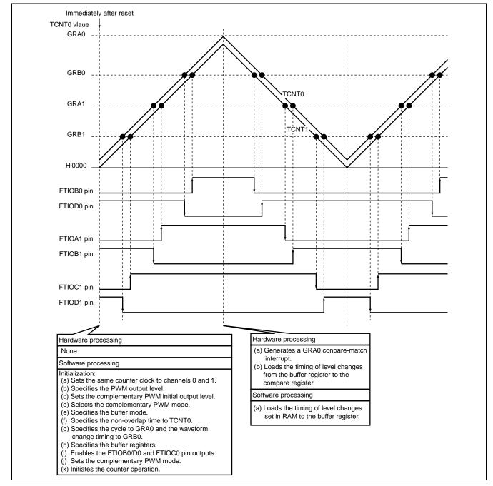
Figure 3.3 Operational Principle of PWM Waveform Output
