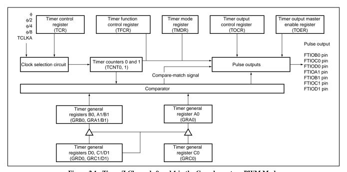
Figure 2.1 Timer Z Channels 0 and 1 in the Complementary PWM Mode
