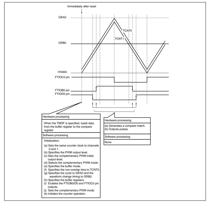
Figure 3.2 Operational Principle for the Output of a Waveform Toggled in Synchronization with the PWM Cycle
