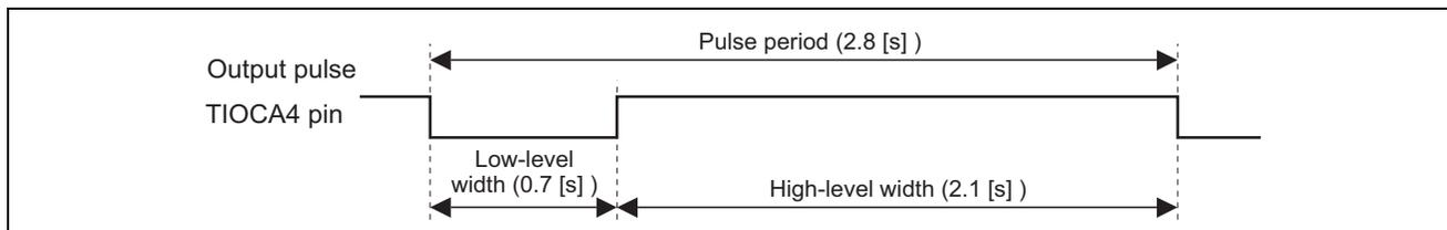
**Figure 1 Example of Long-Period Pulse Output**
