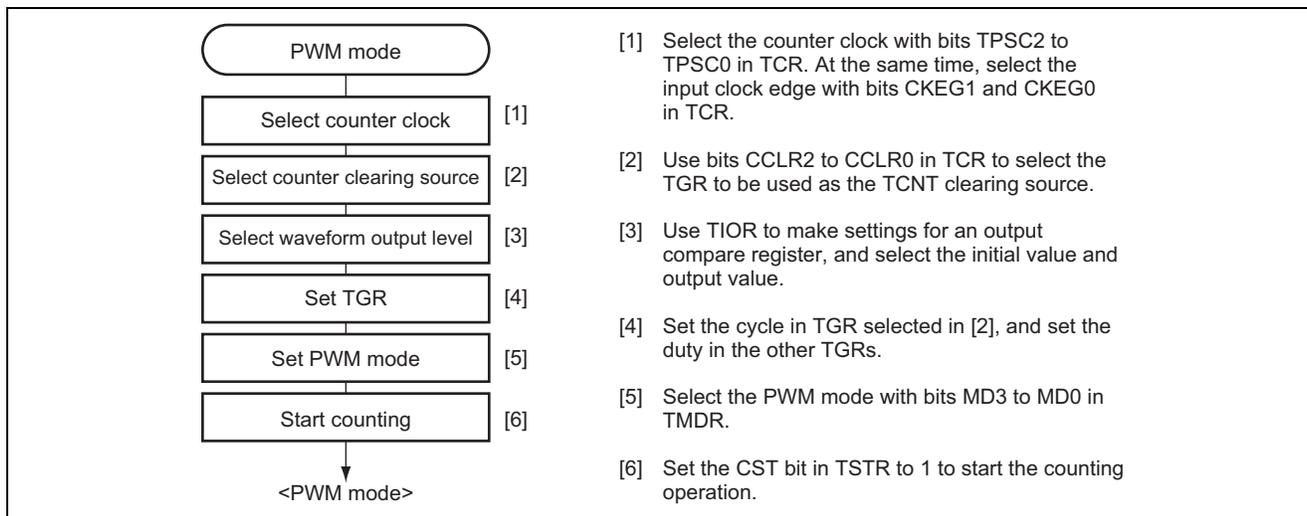
**Figure 4 Example of Procedure for Setting PWM Mode**
