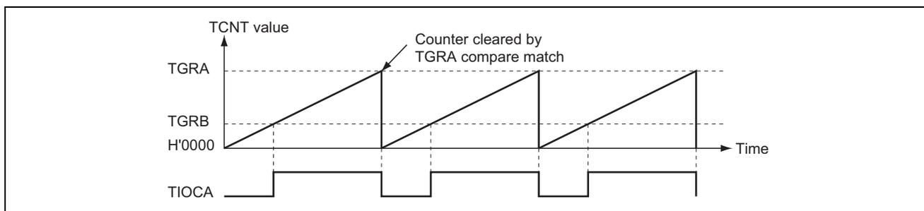
**Figure 5 Example of PWM Mode Operation (1)**
