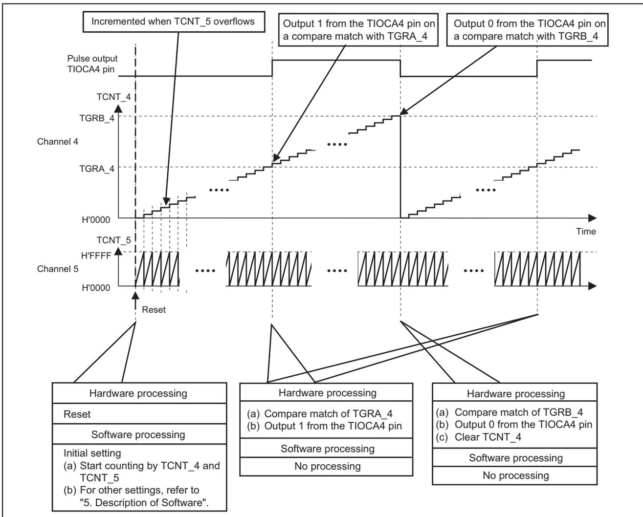
Figure 7 Timing of Operation to Output Long-Period Pulses
