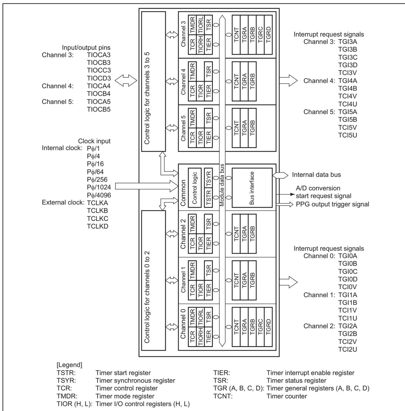
**Figure 2 Block Diagram of the TPU**
