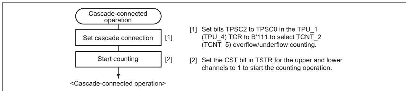
**Figure 3 Example of Procedure for Setting Cascade-Connected Operation**
