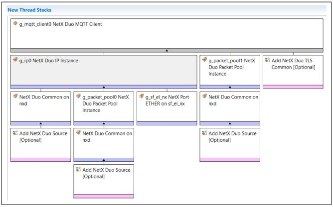
Figure 6 MQTT Client block with the NetX Port Ether driver added
